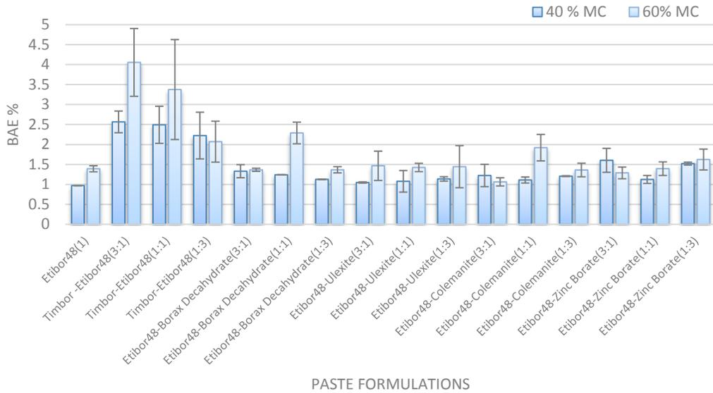
Figure IV-14. Boron levels 0–6 mm from the surface in Douglas-fir blocks conditioned to 40% or 60% MC and then treated with Etibor48 in 16 different paste formulations and incubated for 6 weeks (BAE = boric acid equivalent).
