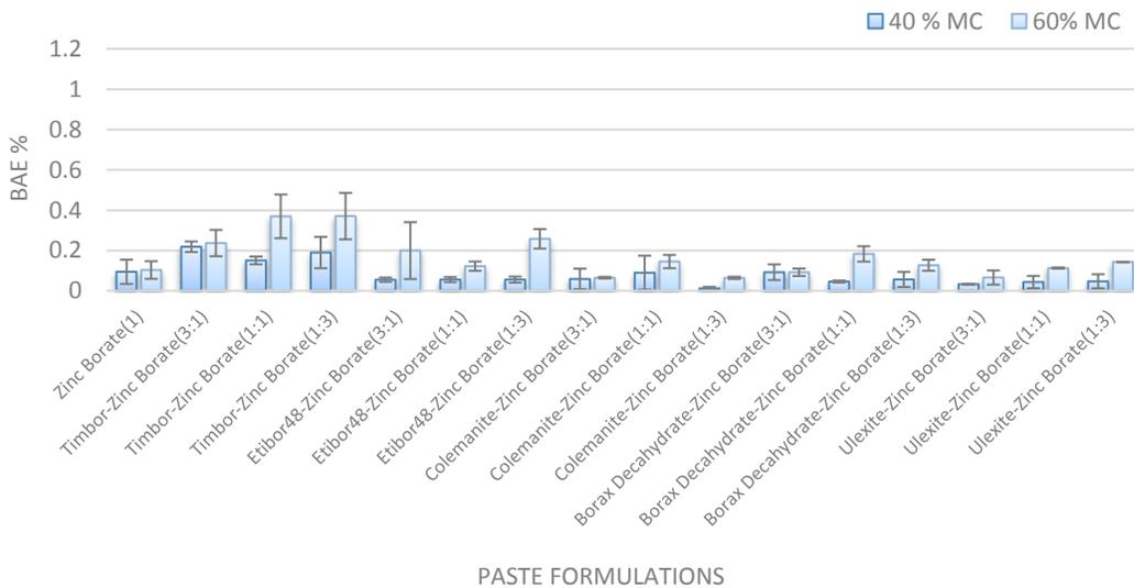
Figure IV-26. Boron levels 6–13 mm from the surface in Douglas-fir blocks conditioned to 40% or 60% MC and then treated with zinc borate in 16 different paste formulations and incubated for 6 weeks (BAE = boric acid equivalent).
