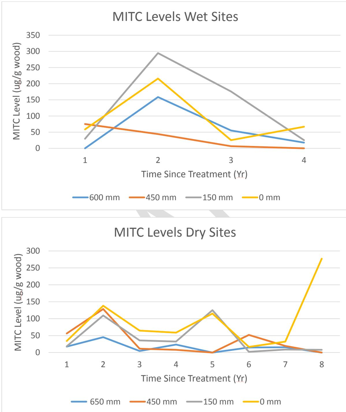
Figure I-21. Residual MITC levels between groundline and 600 mm below groundline in the inner zones of Douglas-fir poles in wet or dry sites 1 to 8 years after dazomet treatment.
