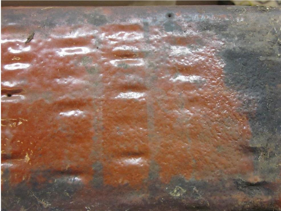
*Figure III-2. Example of lower, non-UV exposed surface of a coated, penta treated section showing evidence of oil migration towards the surface after 6 years of exposure in Hilo, Hawaii.*
