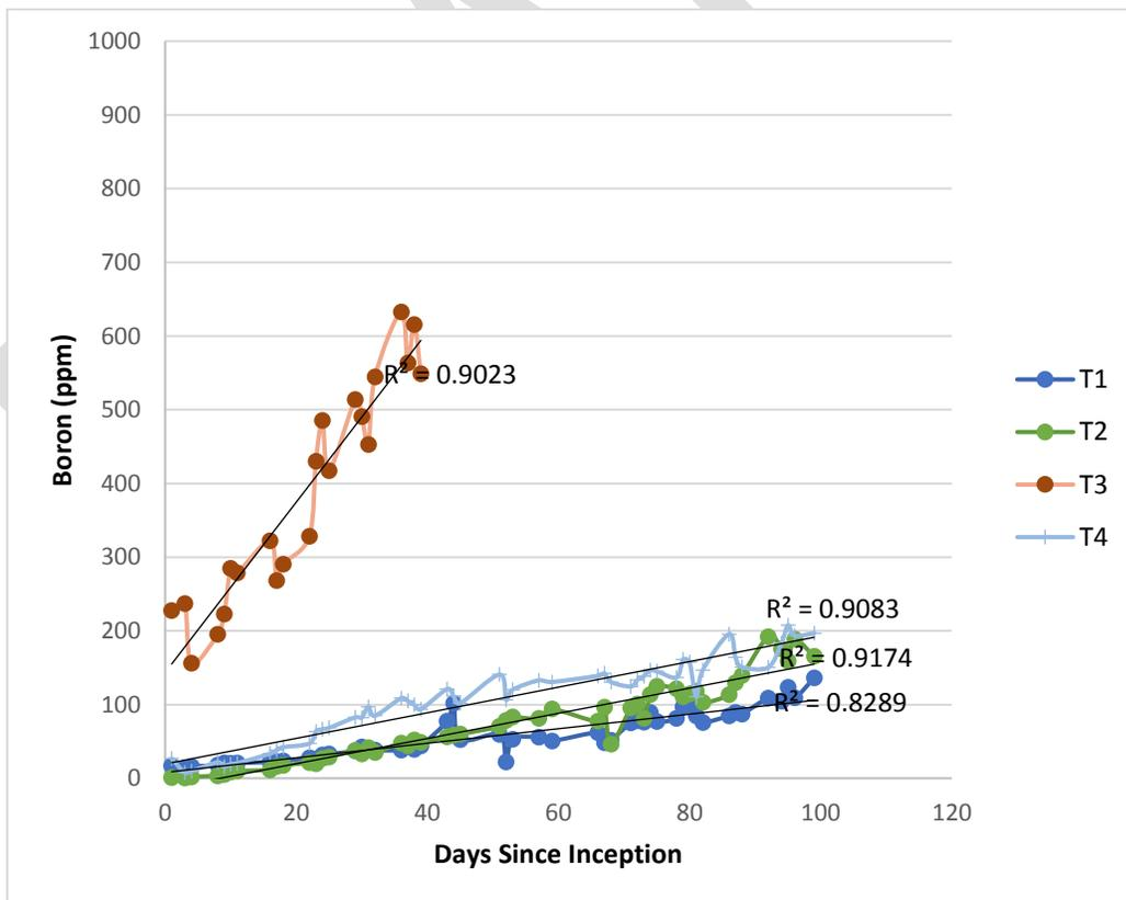
Figure I-16. Boron concentrations vs time on the receiving end of diffusion tests using radially oriented Douglas-fir sapwood with (T samples) or without a biodiesel treatment (C samples). Test sample T3 developed a leak and was dropped from the test
