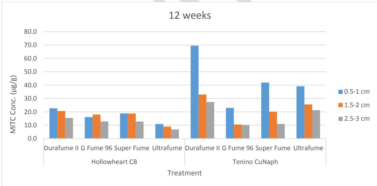
Figure I-4. MITC content above and below a treatment hole 12 weeks after receiving various dazomet formulations with either a micronized copper or copper naphthenate.
