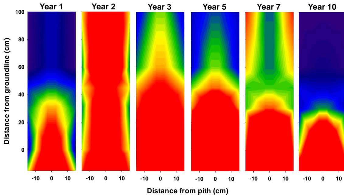
Figure I-5. MITC distribution in Douglas-fir poles 1, 3, 5, 7 and 10 years after treatment with granular dazomet alone with no additional copper naphthenate accelerant. Values moving from light blue to yellow or red signify MITC levels increasingly above the threshold for fungal protection ( $20 \mu\text{g/g}$  wood).
