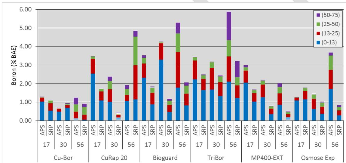
Figure IV-3. Boron content in the outer 75 mm of poles of various species segregated by utility 17, 30, or 56 months after application of various boron-containing pastes. Solid bars are above the toxic threshold of 0.275% BAE for the outer zone or 0.10 for the three inner zone.
