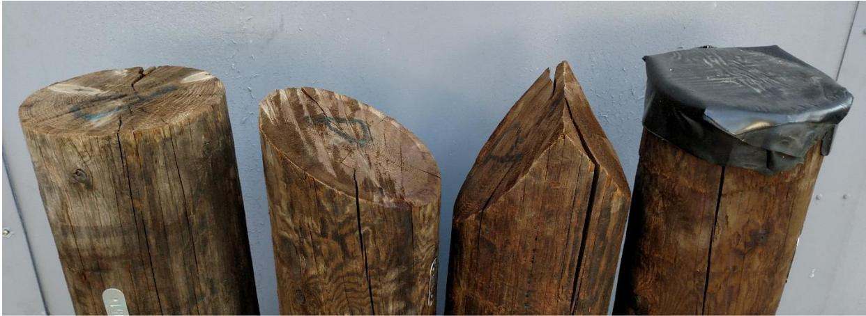
Figure III-12. Examples of the different pole top roofing patterns assessed for their ability to resist moisture ingress.
