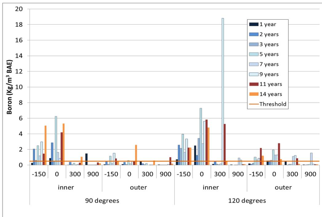
Figure I-10. Boron levels at selected locations above or below groundline in Douglas-fir poles 1 to 14 years after treatment with 4 boron/copper rods.
