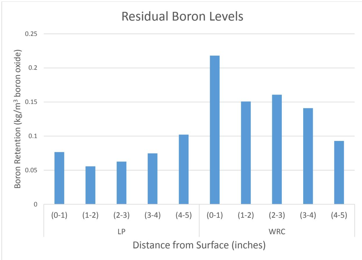
Figure III-26. Residual boron levels in western redcedar and lodgepole pole pine poles sampled after various treatment periods.
