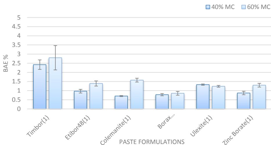
Figure IV-12. Boron levels 0–6 mm from the surface in Douglas-fir sapwood blocks conditioned to 40% or 60% MC and then treated with one of six different paste formulations and incubated for 6 weeks (BAE = boric acid equivalent).
