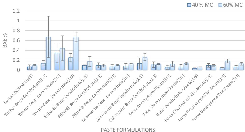
Figure IV-24. Boron levels 6–13 mm from the surface in Douglas-fir blocks conditioned to 40% or 60% MC and treated with Borax Decahydrate in 16 different paste formulations and incubated for 6 weeks (BAE = boric acid equivalent).
