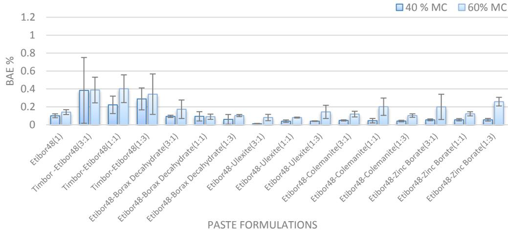
Figure IV-22. Boron levels 6–13 mm from the surface in Douglas-fir blocks conditioned to 40% or 60% MC and then treated with Etibor48 in 16 different paste formulations and incubated for 6 weeks (BAE = boric acid equivalent).
