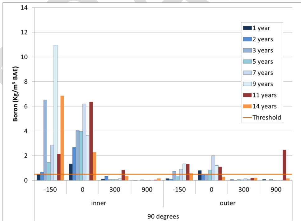
Figure I-12. Boron levels at selected locations above or below groundline in Douglas-fir poles 1 to 14 years after treatment with 8 boron/copper rods.
