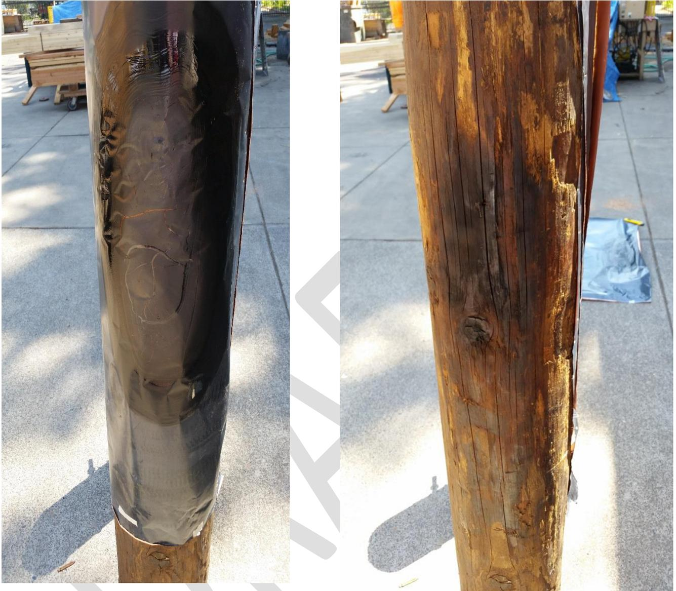
*Figure III-17. CopperCare barrier system showing damage to the barrier but only slight charring beneath after the barrier was removed.*
