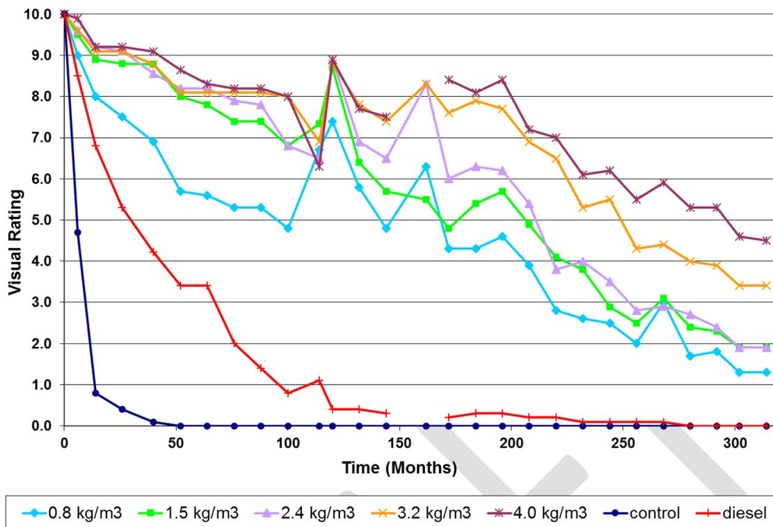
Figure V-2. Condition of weathered western redcedar sapwood stakes treated with selected retentions of copper naphthenate in diesel oil and exposed in a soil bed for 314 months.
