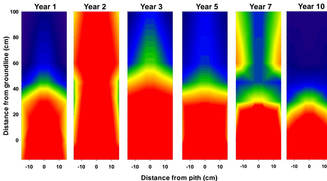
Figure I-8. MITC distribution in Douglas-fir poles 1 to 10 years after treatment with dazomet in a cardboard tube along with a copper naphthenate accelerant. Values moving from light blue to yellow or red signify MITC levels increasingly above the threshold for fungal protection ( $20 \mu\text{g/g}$  wood).
