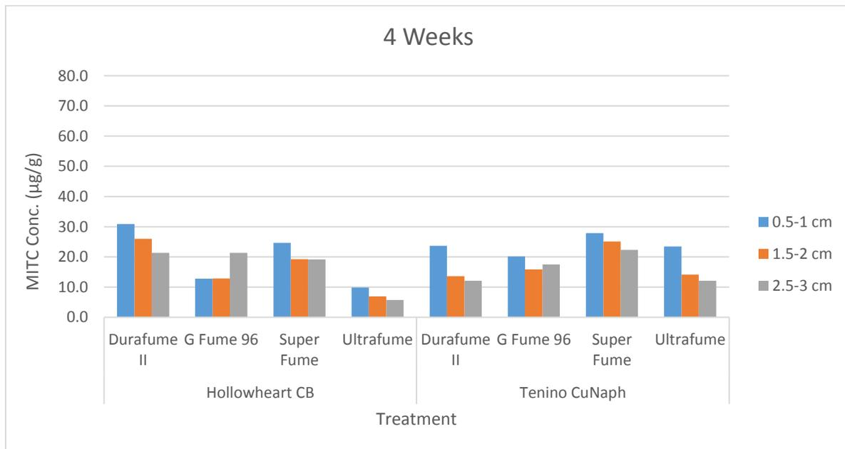
Figure I-2. MITC content above and below a treatment hole 4 weeks after receiving various dazomet formulations with either a micronized copper or copper naphthenate.
