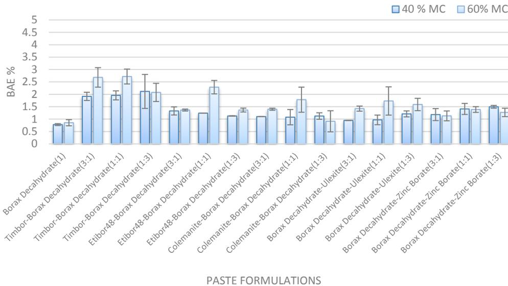
Figure IV-16. Boron levels 0–6 mm from the surface in Douglas-fir blocks conditioned to 40% or 60% MC and then treated with Borax Decahydrate in 16 different paste formulations and incubated for 6 weeks (BAE = boric acid equivalent).
