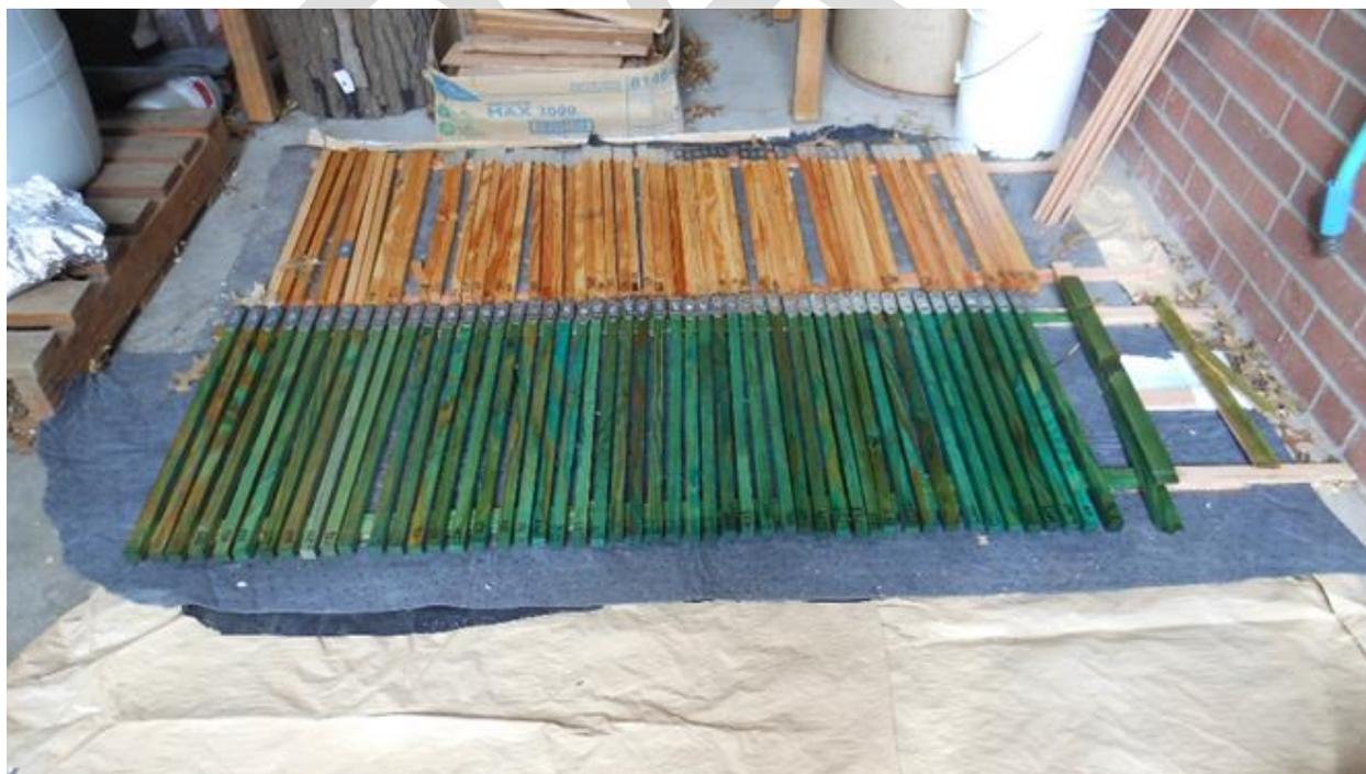
*Figure III-27. Stakes drying under cover after treatment with copper naphthenate (bottom) or penta (top).*
