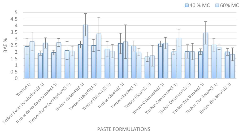
Figure IV-13. Boron levels 0–6 mm from the surface in Douglas-fir blocks conditioned to 40% or 60% MC and then treated with Timbor in 16 different paste formulations and incubated for 6 weeks (BAE = boric acid equivalent).
