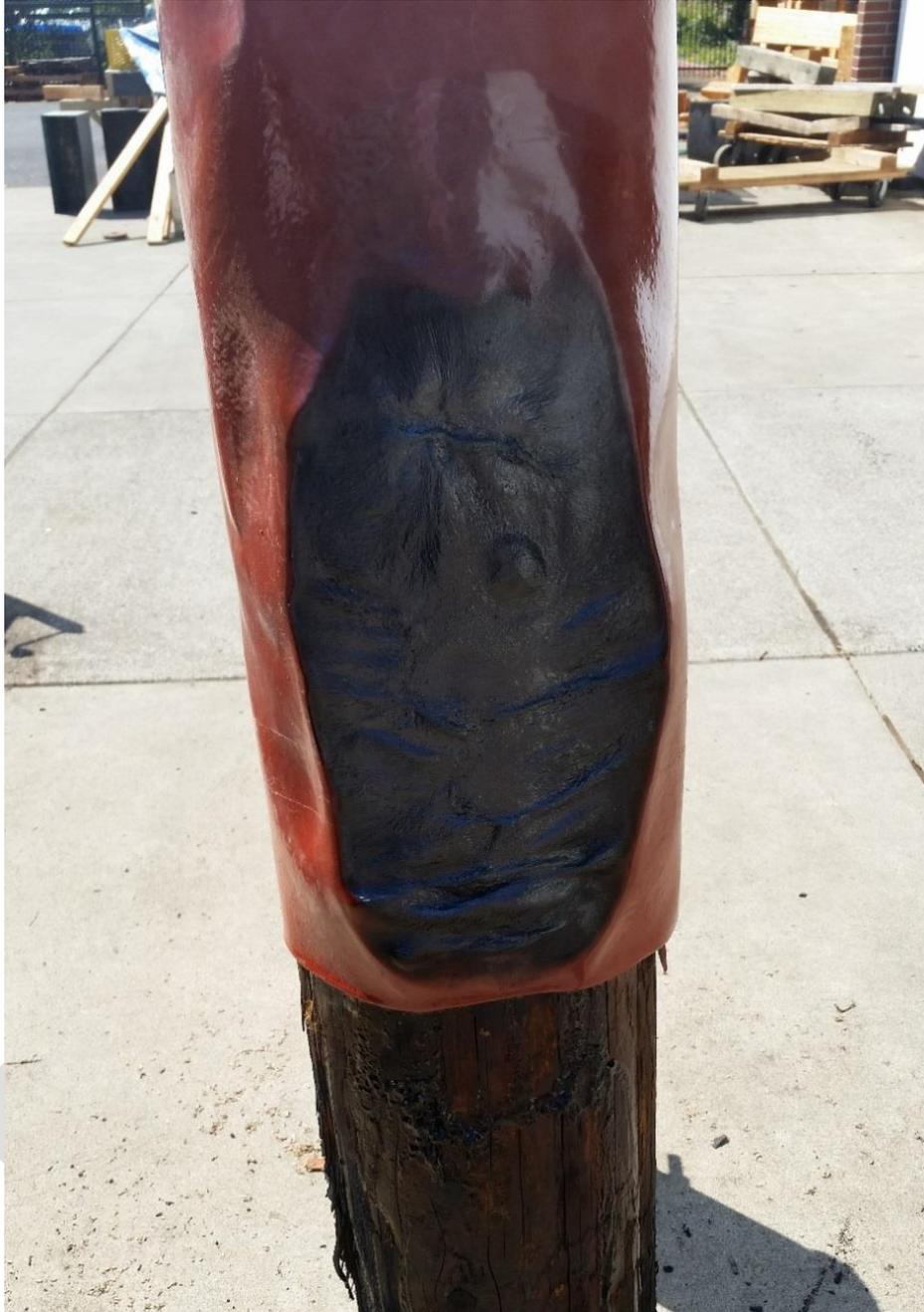
*Figure III-16. Brooks fire retardant wrap after test showing charred area of the barrier that protected the pole from fire.*
