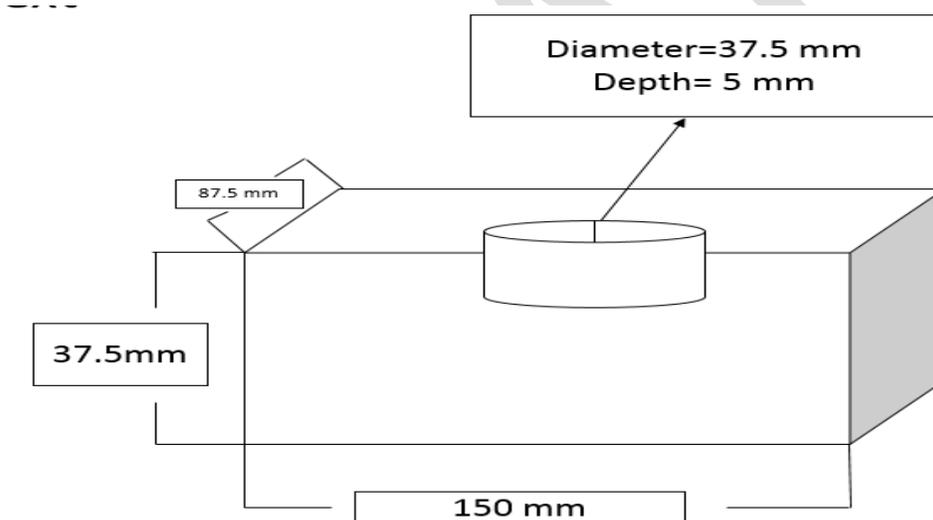
Figure IV-9. Diagram showing a test block with a drilled hole for paste application.
