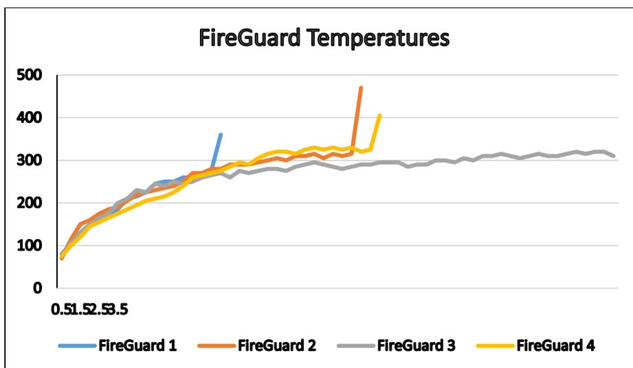
Figure III-21. Surface temperatures on poles treated with Fireguard and subjected to infra-red heating for 30 minutes or until ignition of the wood surface.
