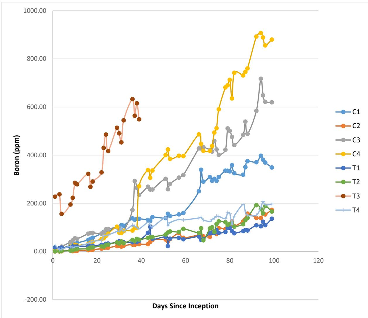
Figure I-15. Boron concentrations on the receiving end of diffusion tests using radially oriented Douglas-fir sapwood with or without a biodiesel treatment where C= no treatment and T= diesel treated samples. The T-3 sample developed a leak and was dropped from the test.
