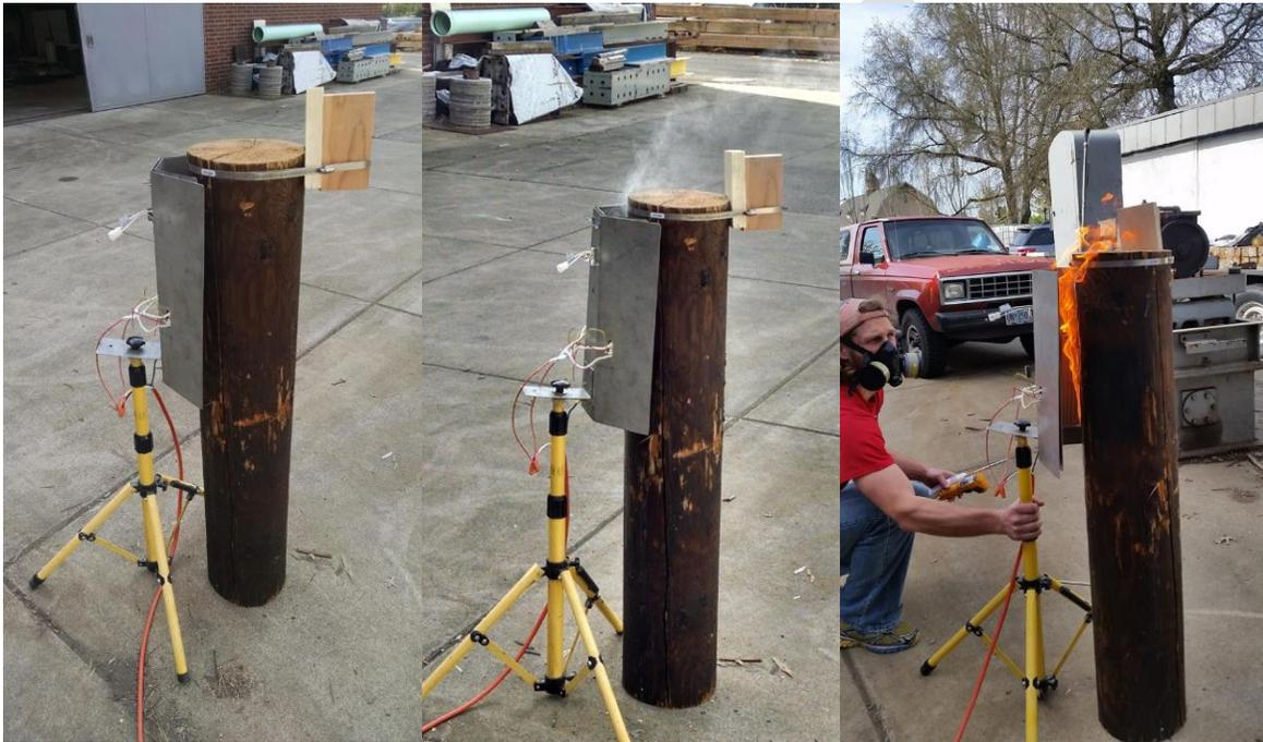
*Figure III-14. Example of the fire test apparatus being applied to a penta treated Douglas-fir pole showing initial heating, the beginning of combustion with smoke and finally, the pole on fire.*
