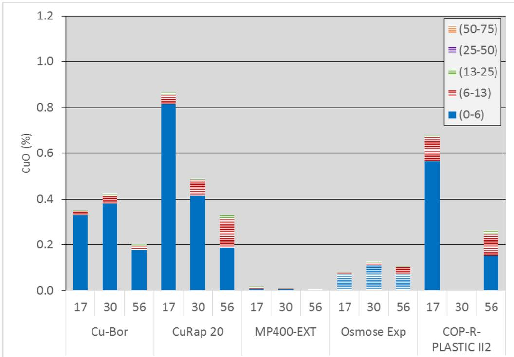
Figure IV-4. Stacked bar graph showing total copper levels in the outer 75 mm of poles 17, 30, or 56 months after application of copper containing preservative pastes. Note that most copper is in the outer assay zone.
