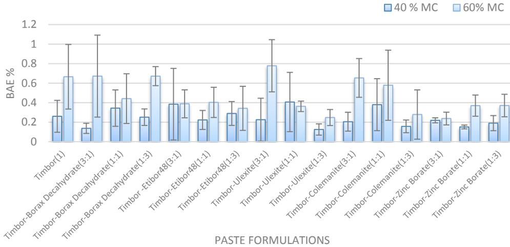
Figure IV-21. Boron levels 6–13 mm from the surface in Douglas-fir blocks conditioned to 40% or 60% MC and then treated with Timbor in 16 different paste formulations and incubated for 6 weeks (BAE = boric acid equivalent).
