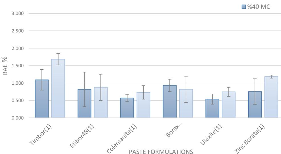
Figure IV-11. Boron levels in the outer 0–6 mm from the treated surface in Douglas-fir sapwood
