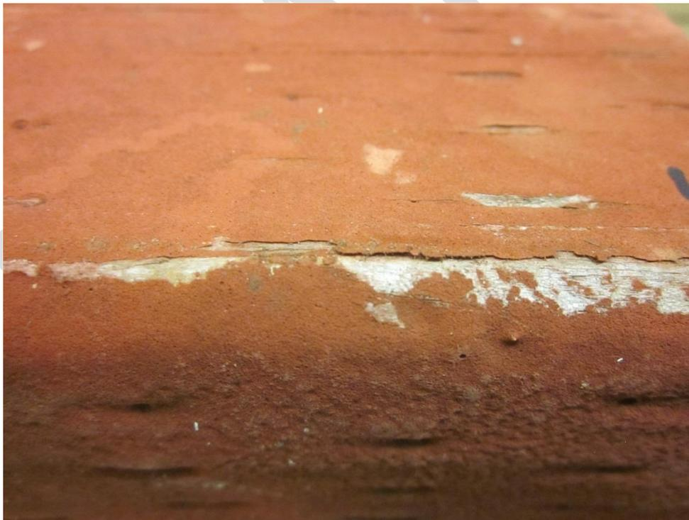
*Figure III-4. Photos of the upper surfaces of coated, non-treated control samples after 6 years of exposure in Hilo, Hawaii showing erosion of the coating and complete loss of coating on the corner.*
