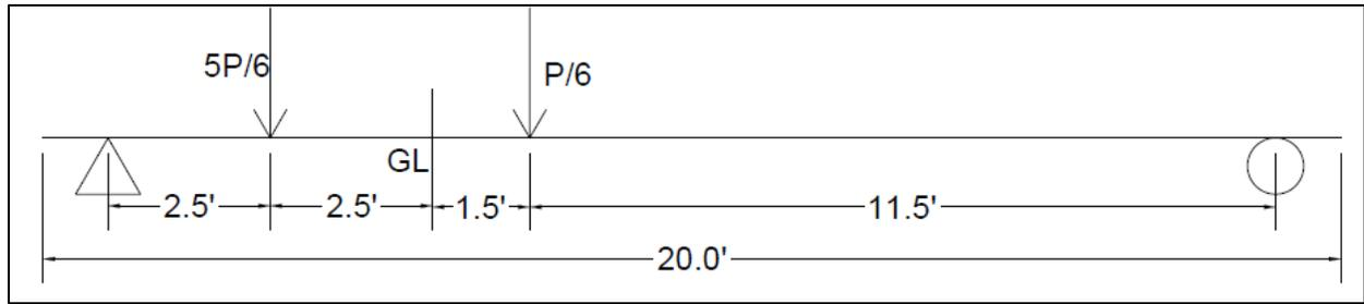
Figure III-6: Diagram of the load distribution in the destructive tests.
