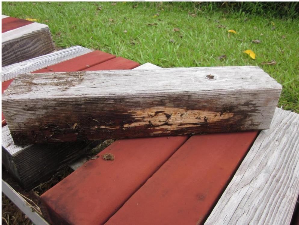
*Figure III-3. Example of a non-treated, non-coated wood sample after 6 years of exposure in Hilo, Hawaii, showing evidence of fungal decay and fruiting bodies.*
