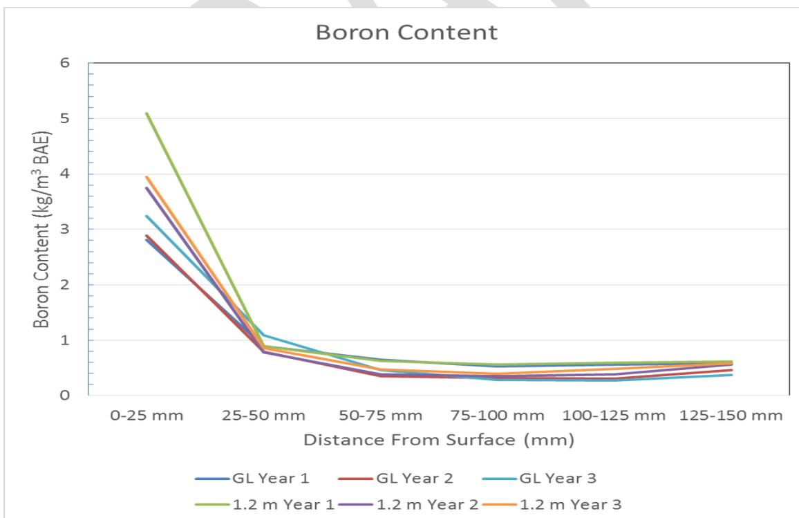
Figure II-2. Boron content at 25 mm increments from Douglas-fir pole surface one to three years after pre-treatment with disodium octaborate tetrahydrate followed by either kiln drying or Boulton seasoning and copper naphthenate treatment. Red line indicates 0.6 kg/m<sup>3</sup> BAE.
