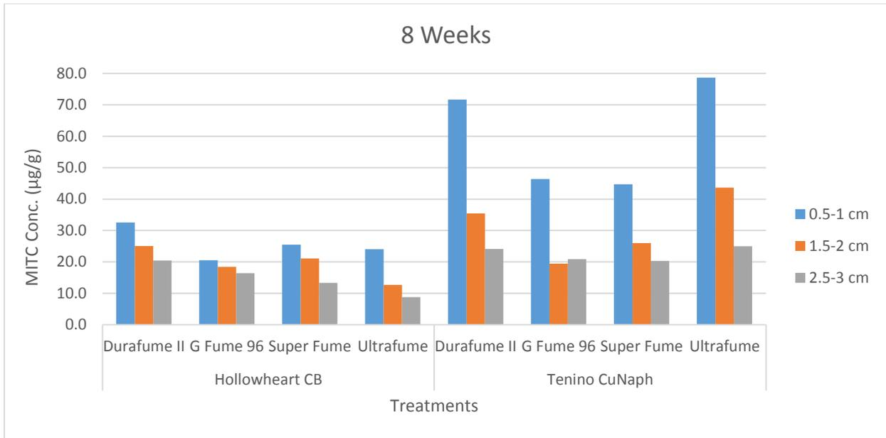
Figure I-3. MITC content above and below a treatment hole 8 weeks after receiving various dazomet formulations with either a micronized copper or copper naphthenate.
