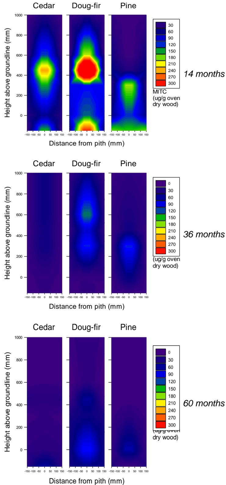
Figure I-18. Diagram showing MITC levels about the groundline in poles 14, 36 or 60 months after application of metam sodium. Red colors indicate elevated levels above the toxic threshold.
