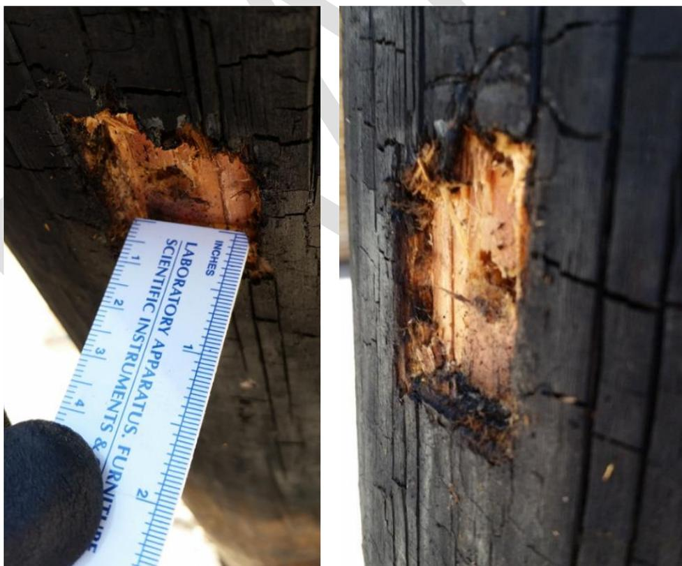
*Figure III-15. Example of char scrapped from the pole surface to reveal non-burned wood beneath.*
