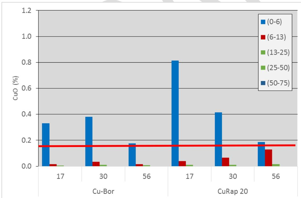
Figure IV-5. Copper levels at selected distances from the surface of poles 17, 30, or 56 months after application of either CuBor or CuRap 20. The horizontal line indicates the presumed protective threshold for the form of copper in these systems.
