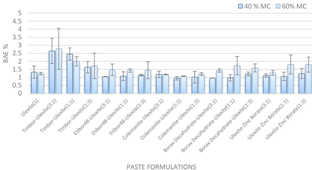
Figure IV-17. Boron levels 0–6 mm from the surface in Douglas-fir blocks conditioned to 40% or 60% MC and then treated with Ulexite in 16 different paste formulations and incubated for 6 weeks (BAE = boric acid equivalent).
