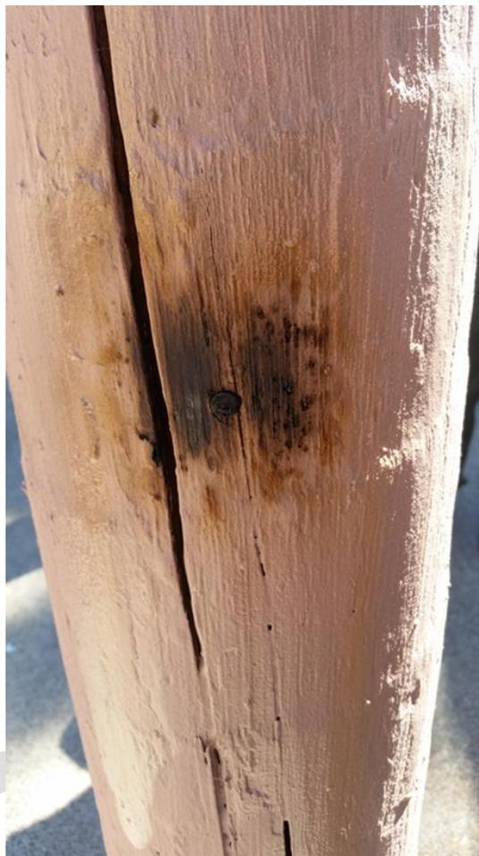
*Figure III-19. Example of a FireGuard treated pole section showing slight charring where the barrier was sacrificed.*
