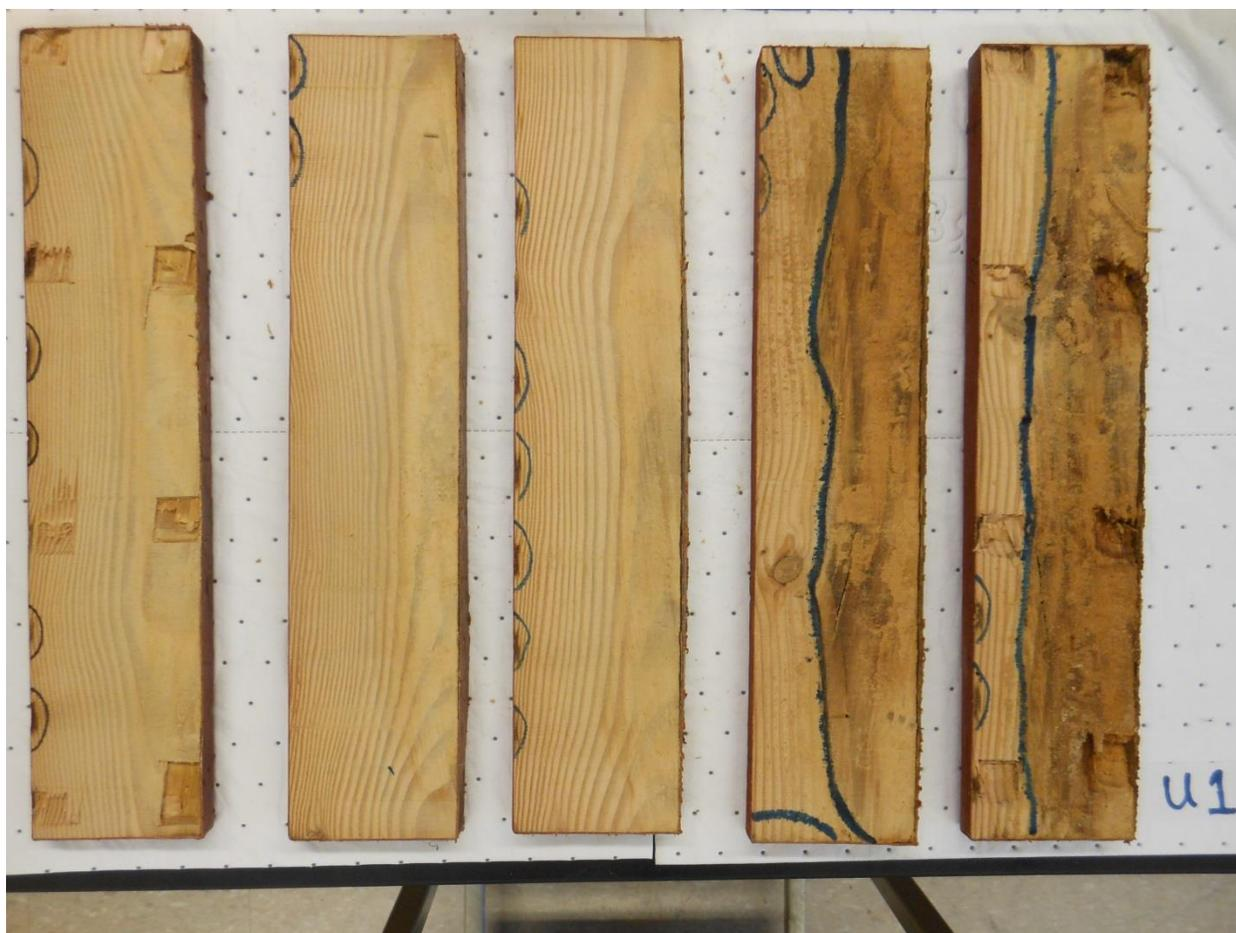
*Figure III-5. Interior of a coated, untreated Douglas-fir section after 6 years of aboveground exposure in Hilo, Hawaii.*
