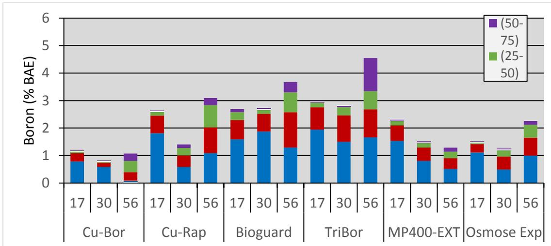
Figure IV-2. Total boron measured in the outer 75 mm of poles 17, 30 or 56 months after treatment with selected boron-containing pastes. Solid bars are above the toxic threshold of 0.275% BAE for the outer zone or 0.10 for the three inner zones.
