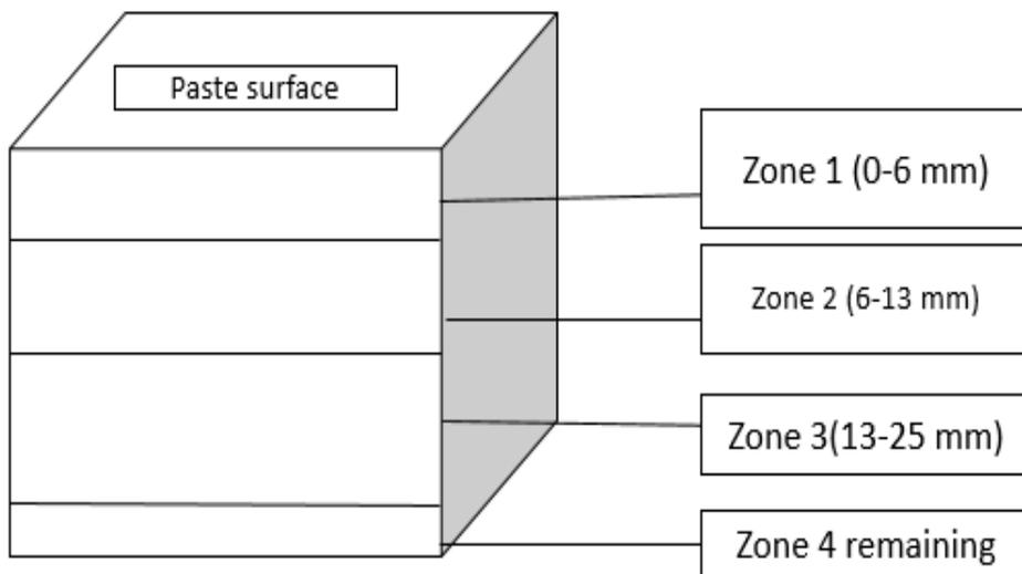
*Figure IV-10. Diagram showing the cutting pattern for examining boron content in Douglas-fir blocks 3 or 6 weeks after the application of various boron pastes.*
