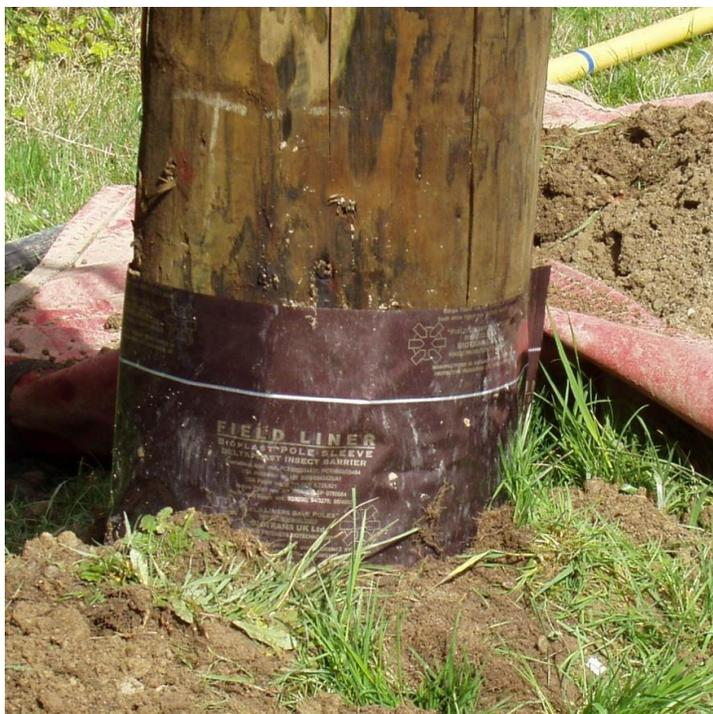
Figure IV-8. Example of a Biotrans liner at the Peavy Arboretum test site.
