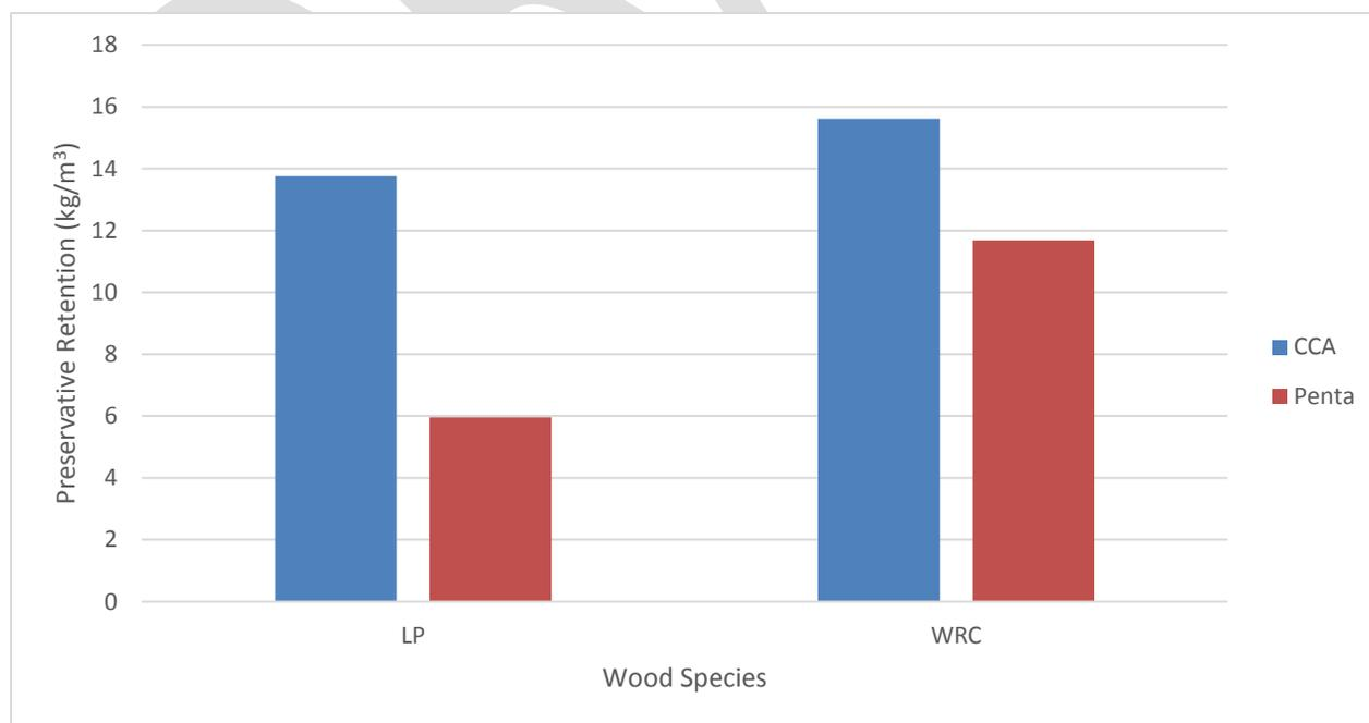
*Figure III-23. Residual penta or CCA retention in lodgepole pine and western redcedar poles. Minimum CSA retention levels for CCA at 9.6 and 16.0 kg/m<sup>3</sup> for lodgepole pine and western redcedar, respectively. Minimum CSA retention levels for penta are 9.6 and 12.8, kg/m<sup>3</sup> respectively, for the same species.*
