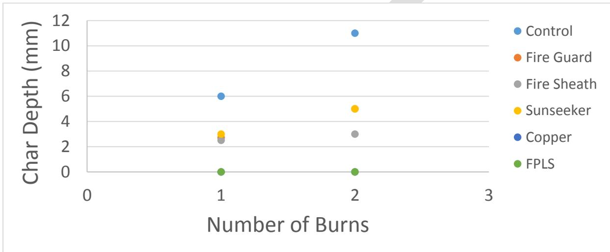
Figure III-20. Char depth on penta treated Douglas-fir pole sections with or without a fire retardant barrier after to two simulated fire exposures.
