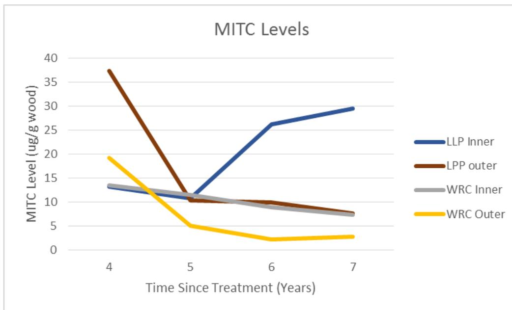
Figure III-25. MITC content in the inner and outer 25 mm of increment cores removed from the groundline of lodgepole pine (LPP) or western redcedar (WRC) poles 4 to 7 years after treatment with metam sodium.
