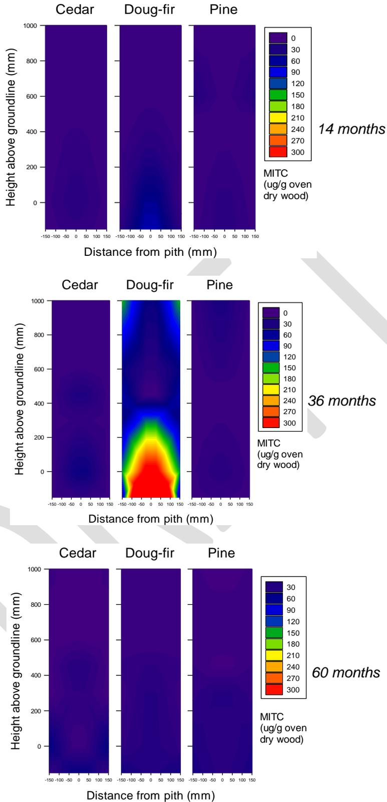
Figure I-19. Diagram showing MITC levels about the groundline in poles 14, 36, or 60 months after application of dazomet without accelerant. Red colors indicate elevated levels above the toxic threshold.
