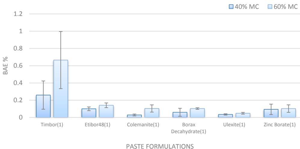
Figure IV-20. Boron levels 6–13 mm from the surface in Douglas-fir sapwood blocks conditioned to 40% or 60% MC and then treated with one of six different paste formulations and incubated for 6 weeks (BAE = boric acid equivalent).
