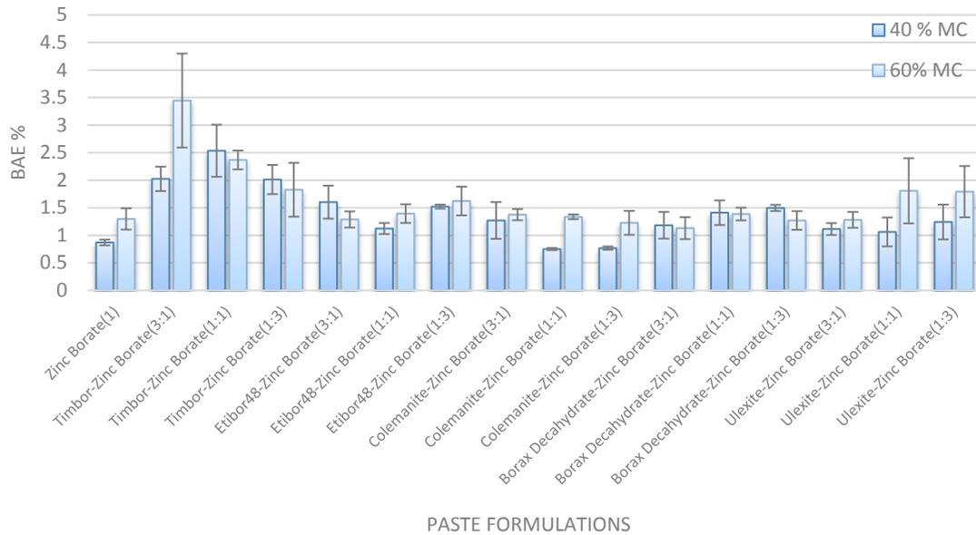
Figure 11V-18. Boron levels 0–6 mm from the surface in Douglas-fir blocks conditioned to 40% or 60% MC and then treated with zinc borate in 16 different paste formulations and incubated for 6 weeks (BAE = boric acid equivalent).
