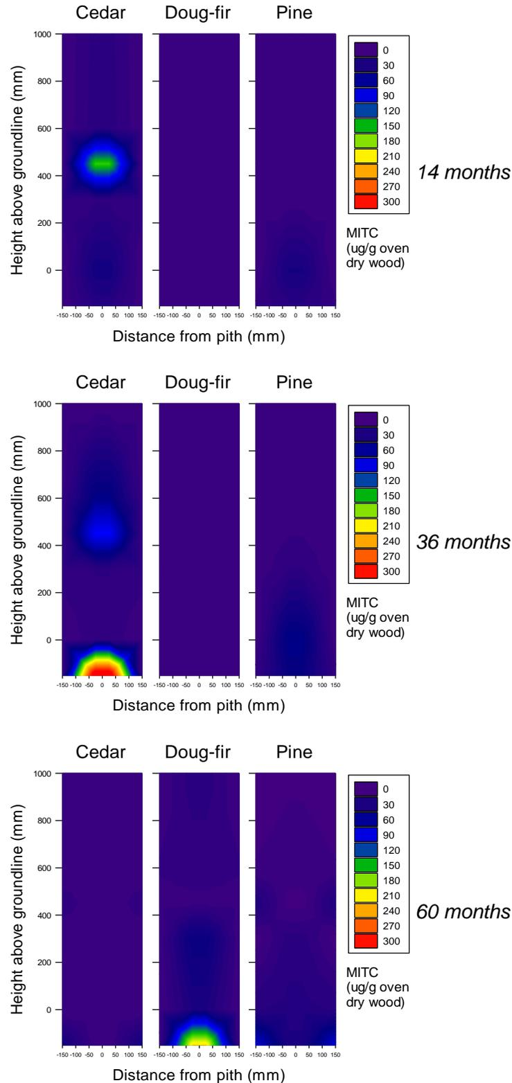
Figure I-20. Diagram showing MITC levels about the groundline in poles 14, 36, or 60 months after application of dazomet with copper naphthenate accelerant. Red colors indicate elevated levels above the toxic threshold.
