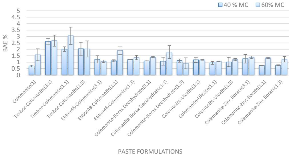
Figure IV-15. Boron levels 0–6 mm from the surface in Douglas-fir blocks conditioned to 40% or 60% MC and then treated with Colemanite in 16 different paste formulations and incubated for 6 weeks (BAE = boric acid equivalent).
