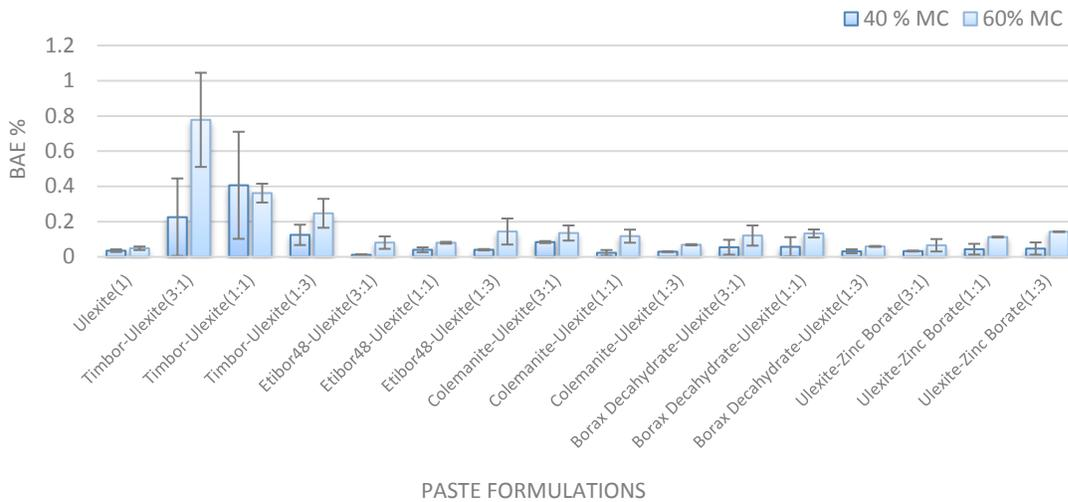
Figure IV-25. Boron levels 6–13 mm from the surface in Douglas-fir blocks conditioned to 40% or 60% MC and then treated with Ulexite in 16 different paste formulations and incubated for 6 weeks (BAE = boric acid equivalent).
