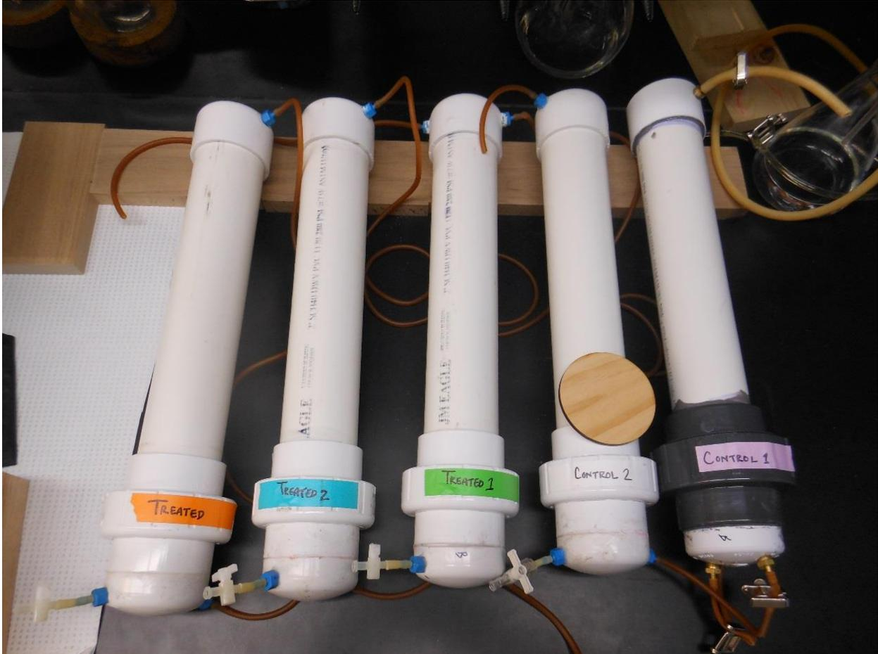
*Figure I-14. Photograph of five of the diffusion apparatus used to assess boron movement through non-treated or diesel oil treated Douglas-fir lumber. A wood sample is resting on the fourth chamber to provide a measure of scale.*
