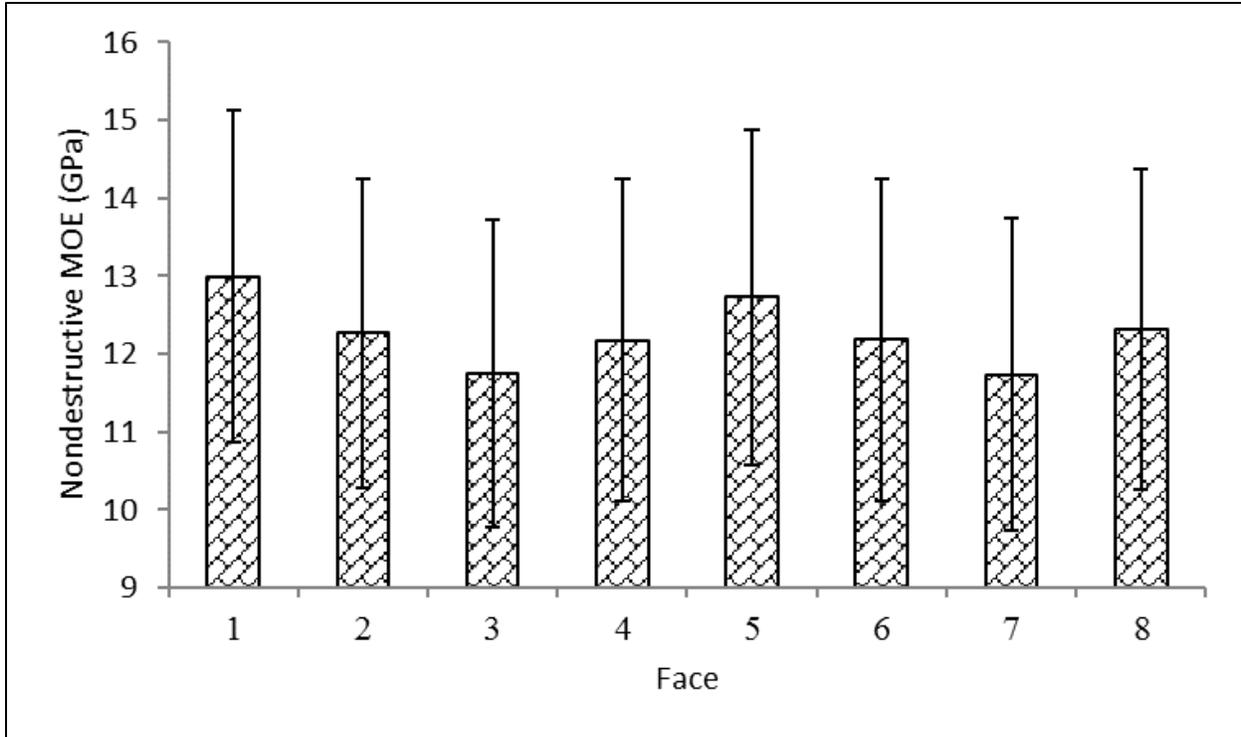
Figure III-8. Average predicted MOE as determined by pre-flexing at the mid-point at 8 equidistant locations around 92 Douglas-fir utility poles.
