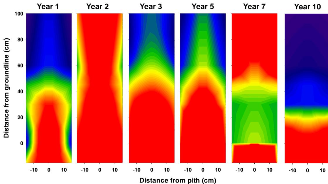
Figure I-6. MITC distribution in Douglas-fir poles 1, 3, 5, 7 and 10 years after treatment with granular dazomet and copper naphthenate accelerant. Values moving from light blue to yellow or red signify MITC levels increasingly above the threshold for fungal protection ( $20 \mu\text{g/g}$  wood).
