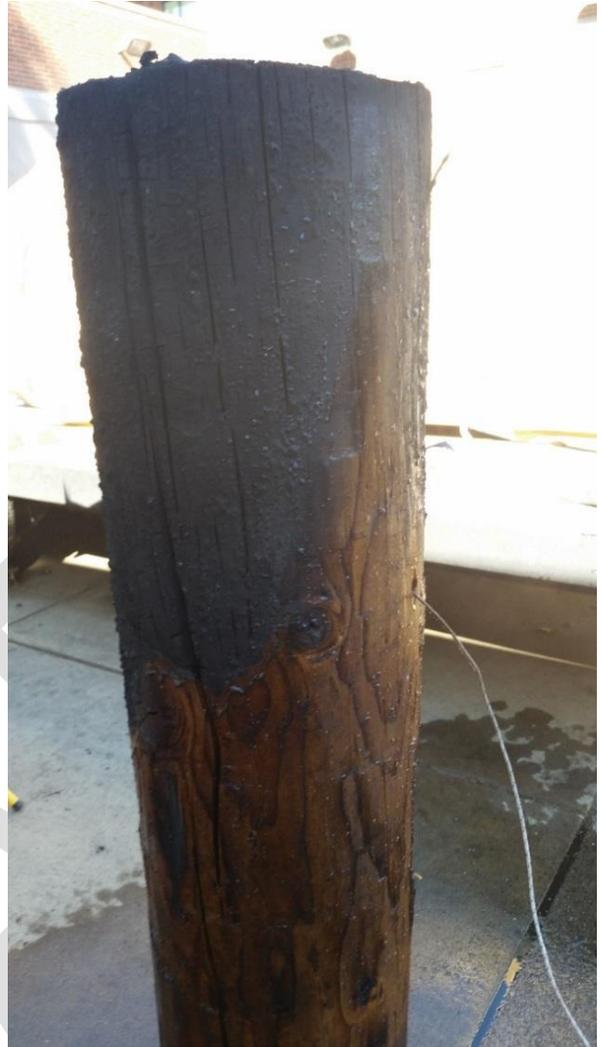
*Figure III-18. Example of SunSeeker fire retardant treated pole on fire and pole condition after the fire*
