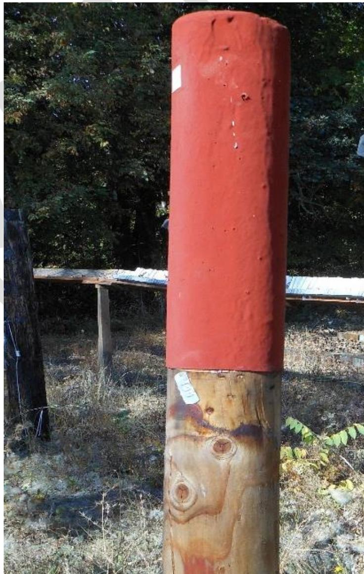
*Table III-7. Moisture content beneath the tops of Douglas-fir poles with and without a water-shedding polyurea coating.*
