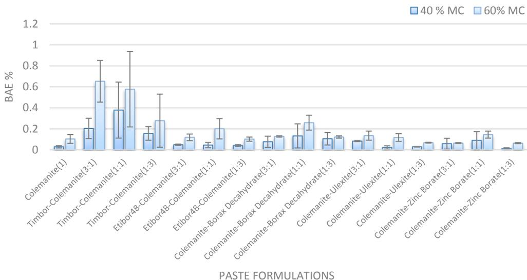
Figure IV-23. Boron levels 6–13 mm from the surface in Douglas-fir blocks conditioned to 40% or 60% MC and then treated with Colemanite in 16 different paste formulations and incubated for 6 weeks (BAE = boric acid equivalent).
