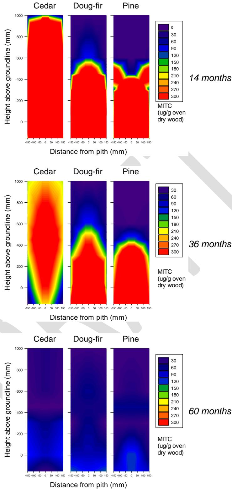
Figure I-17. Diagram showing MITC levels about the groundline in poles 14, 36 or 60 months after application of MITC-FUME. Red colors indicate elevated levels above the toxic threshold.
