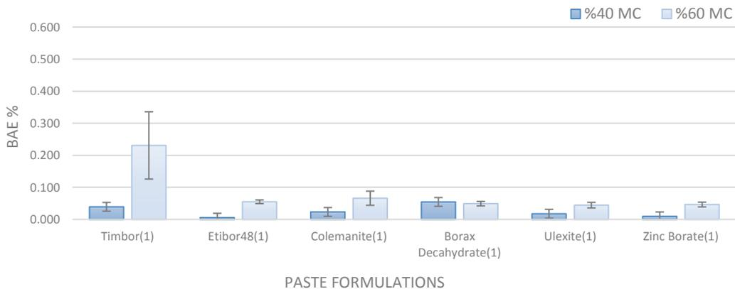
Figure IV-19. Boron levels 6–13 mm from the surface in Douglas-fir sapwood blocks conditioned to 40% or 60% MC and treated with one of six different paste formulations and incubated for 3 weeks (BAE = boric acid equivalent).
