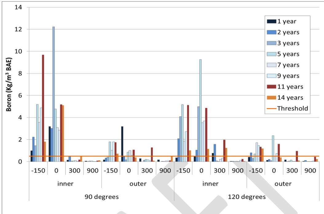
Figure I-11. Boron levels at selected locations above or below groundline in Douglas-fir poles 1 to 14 years after treatment with 4 boron rods. The elevated values at 300 mm in the inner zone of poles treated using a 120 degree spacing likely reflect one very high value from a sample removed immediately adjacent to the original treatment hole.
