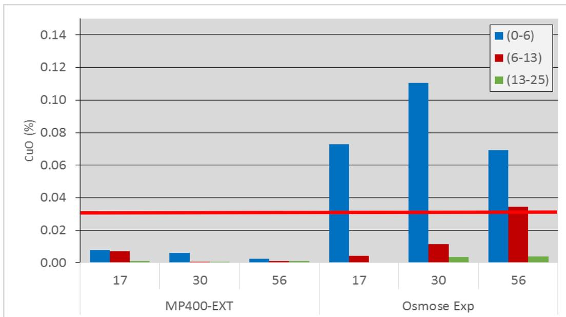
Figure IV-6. Copper levels at selected distances from the surface of poles 17, 30, or 56 months after application of either MP-400-EXT or Osmose Experimental paste. The horizontal line indicates the presumed protective threshold for the form of copper in these systems.
