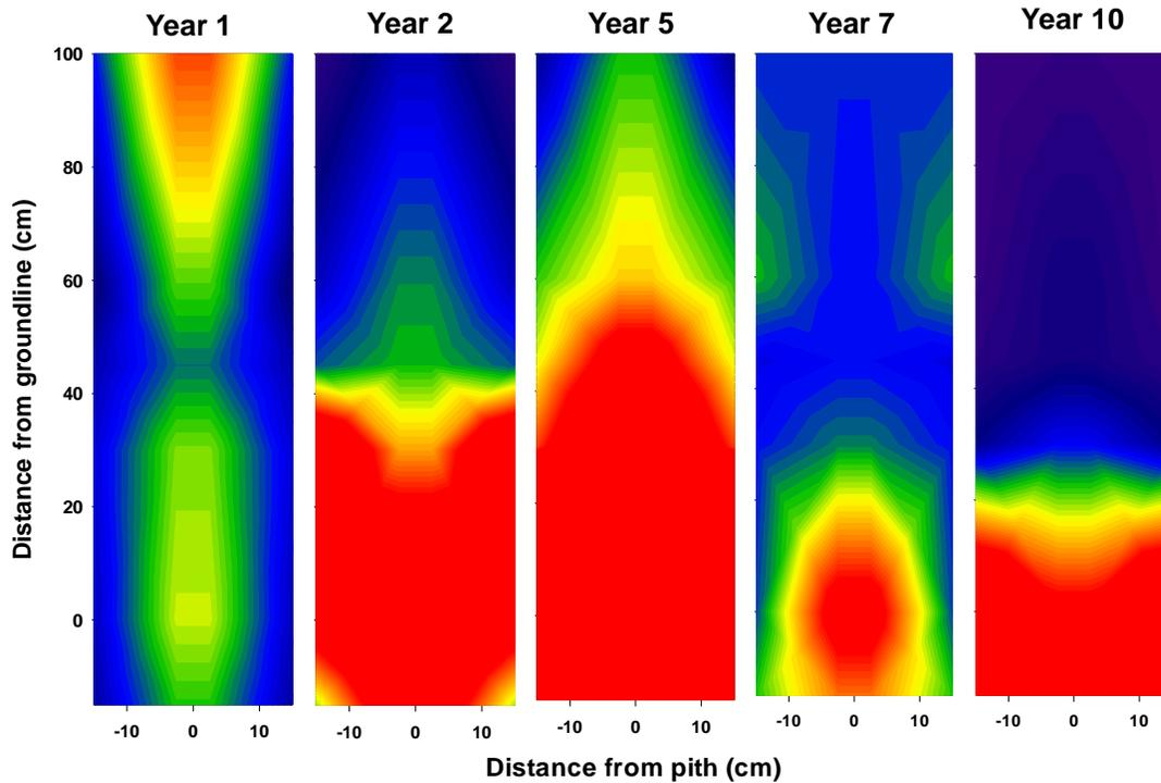
Figure I-9. MITC distribution in Douglas-fir poles 1 to 10 years after treatment with dazomet in a plastic tube followed by a copper naphthenate accelerant. Values moving from light blue to yellow or red signify MITC levels increasingly above the threshold for fungal protection (20 µg/g wood).
