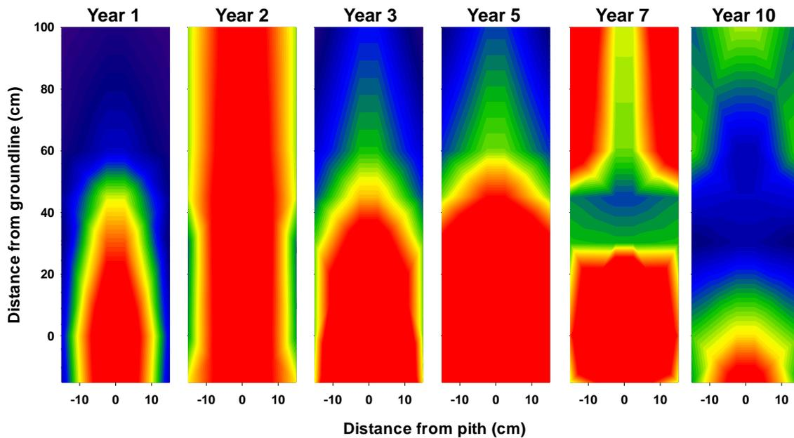
Figure I-7. MITC distribution in Douglas-fir poles 1, 3, 5, 7 and 10 years after treatment with dazomet in a cardboard tube with no additional copper naphthenate accelerant. Values moving from light blue to yellow or red signify MITC levels increasingly above the threshold for fungal protection ( $20 \mu\text{g/g}$  wood).
