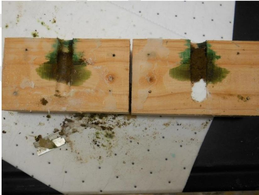
*Figure I-1. Example of a 200 mm long block used to assess copper naphthenate distribution patterns in dazomet treatment holes showing copper naphthenate penetration limited to the upper zone of the treatment hole.*
