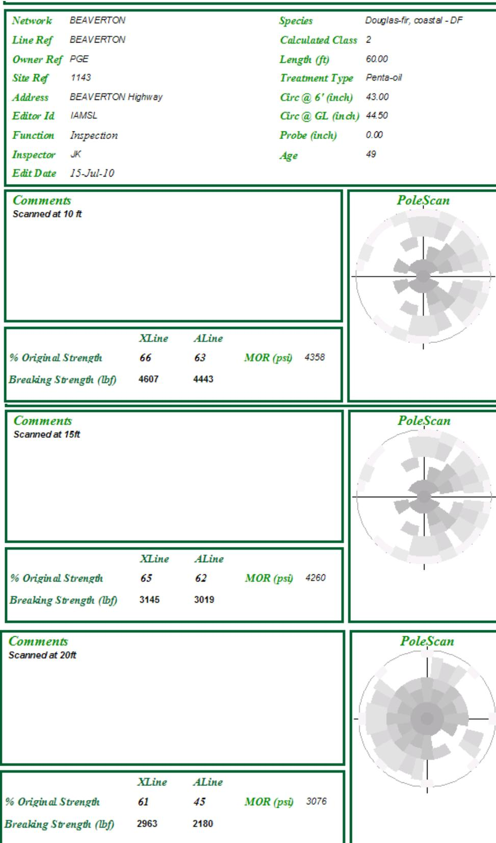
Figure III-12 continued. PoleScan output from above ground inspection of poles within the PGE system showing internal pole condition.
