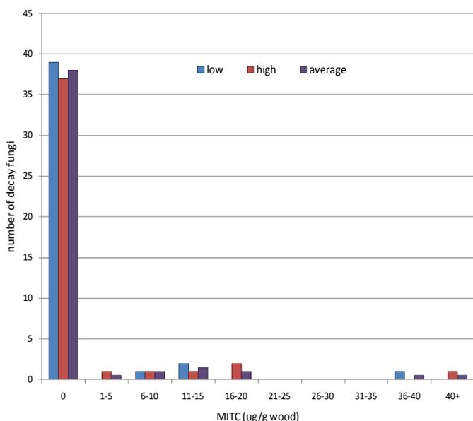
Figure I-1. High, low and average MITC values associated with decay fungi isolated from the same increment core removed from Douglas-fir poles 1 to 15 years after treatment with various MITC based internal treatments.
