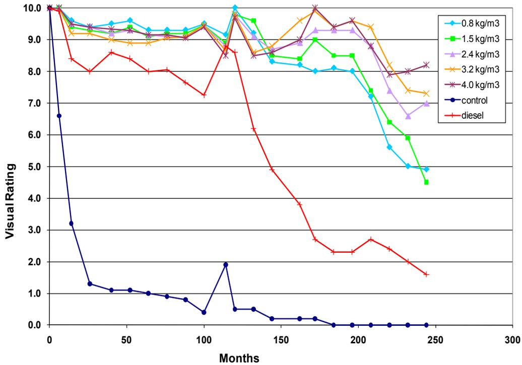
Figure V-1. Condition of freshly sawn western redcedar sapwood stakes treated with selected retentions of copper naphthenate in diesel oil and exposed in a soil bed for 244 months.
