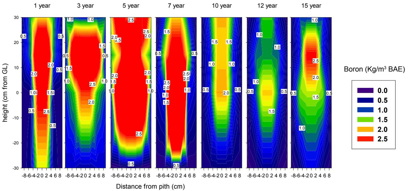
Figure I-14. Boron distribution (Kg/m<sup>3</sup> BAE) in Douglas-fir poles 1 to 15 years after treatment with fused boron rods and Boracare.
