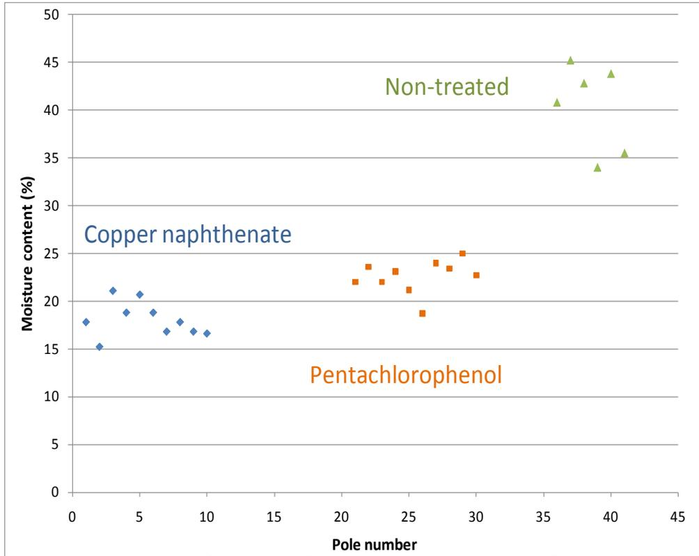
Figure III-15. Moisture contents of Douglas-fir pole sections shortly after treatment with copper naphthenate or pentachlorophenol or left without treatment.
