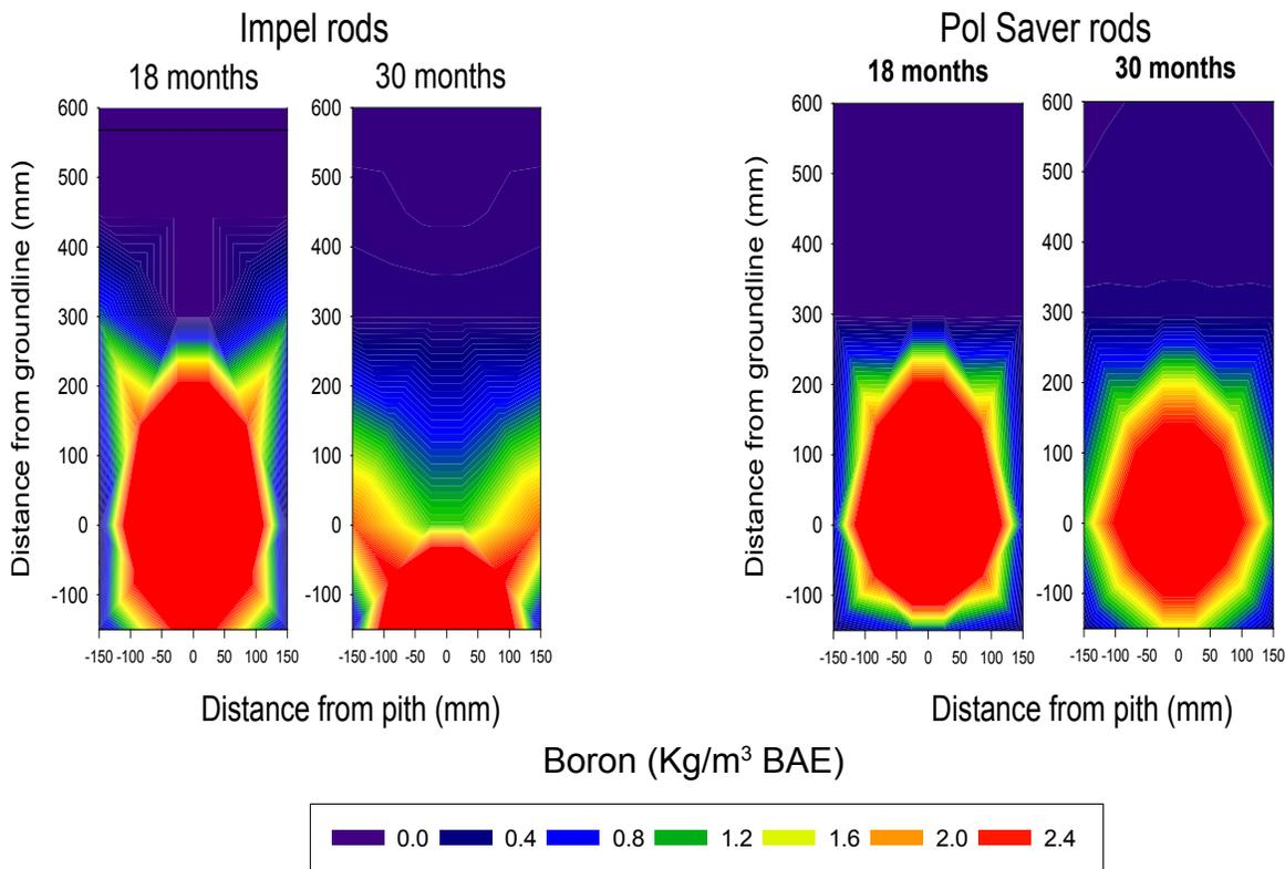
Figure I-24. Boron distribution in Douglas-fir poles 18 and 30 months after application of Impel or Pol Saver rods.
