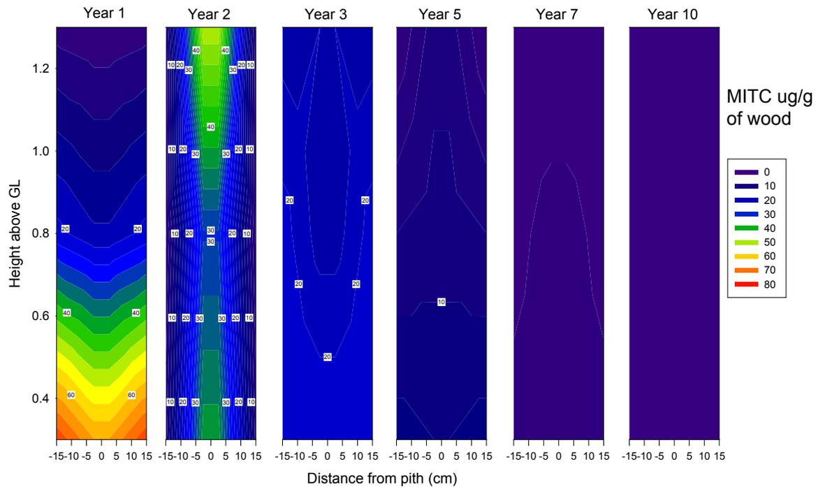
Figure I-4. Residual MITC in Douglas-fir poles 1 to 10 years after treatment with metam sodium.
