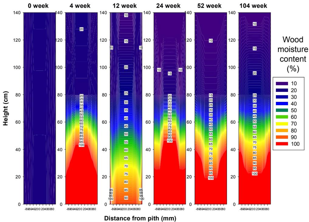
Figure IV-7. Moisture contents of non-treated western redcedar poles immersed in moist soil for 0 to 104 weeks.
