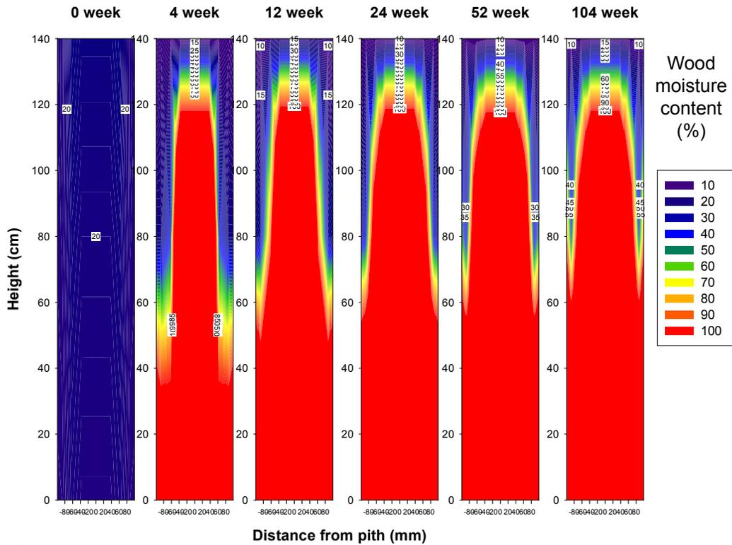
Figure IV-6. Moisture contents of non-treated western redcedar poles immersed in water for 0 to 104 weeks.
