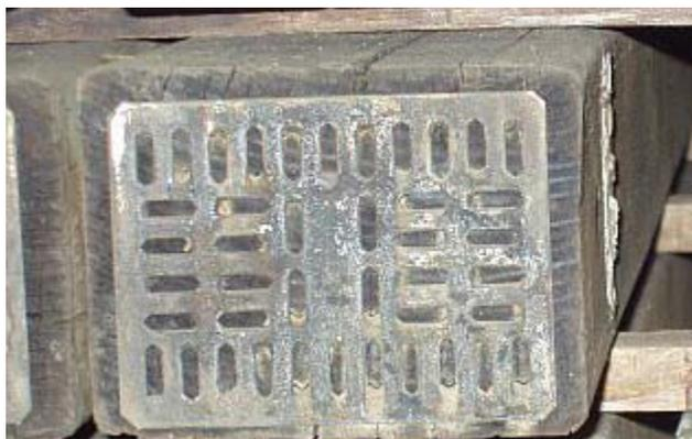
Figure III-6. Example of an end-plate on a penta treated Douglas-fir cross arm.
