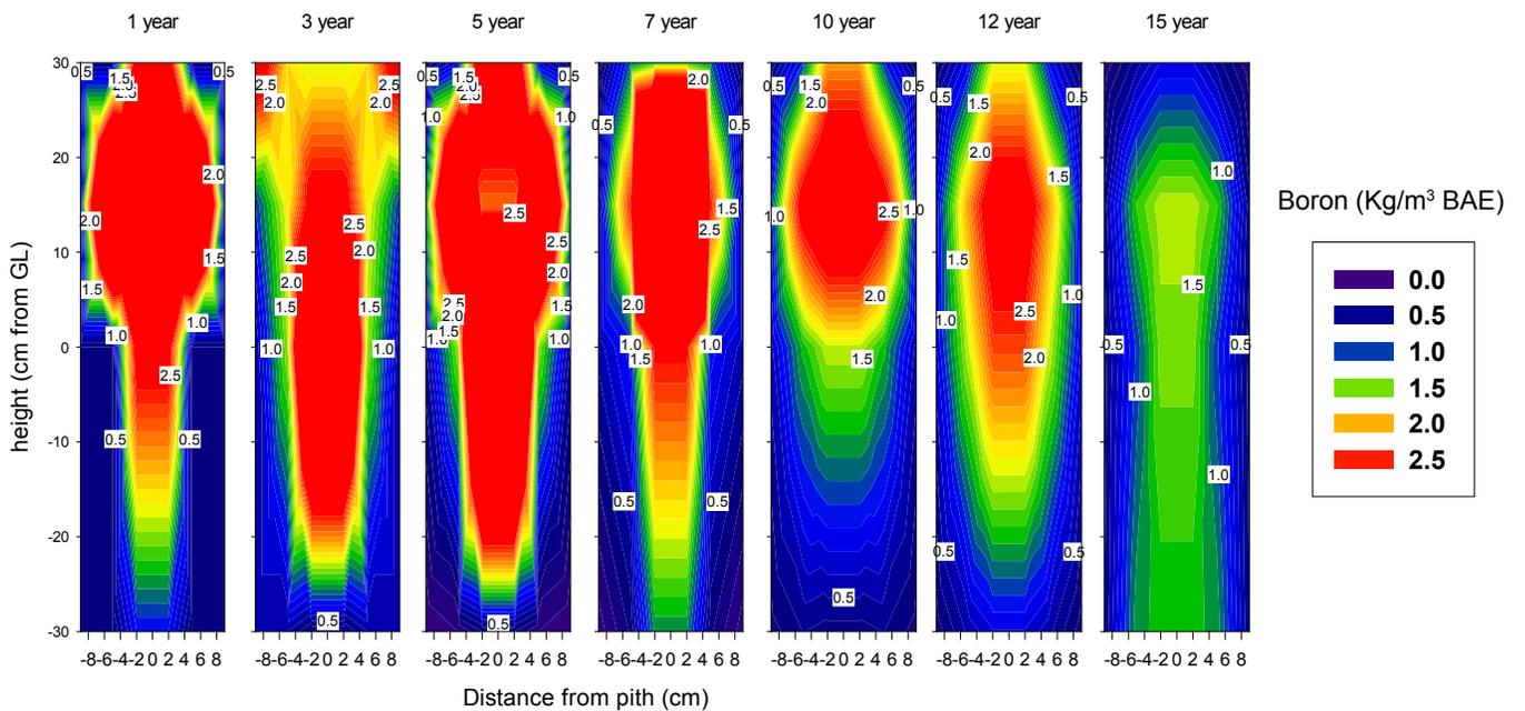
Figure I-18. Boron distribution (Kg/m<sup>3</sup> BAE) in Douglas-fir poles 1 to 15 years after treatment with fused boron rods and Timbor solution.
