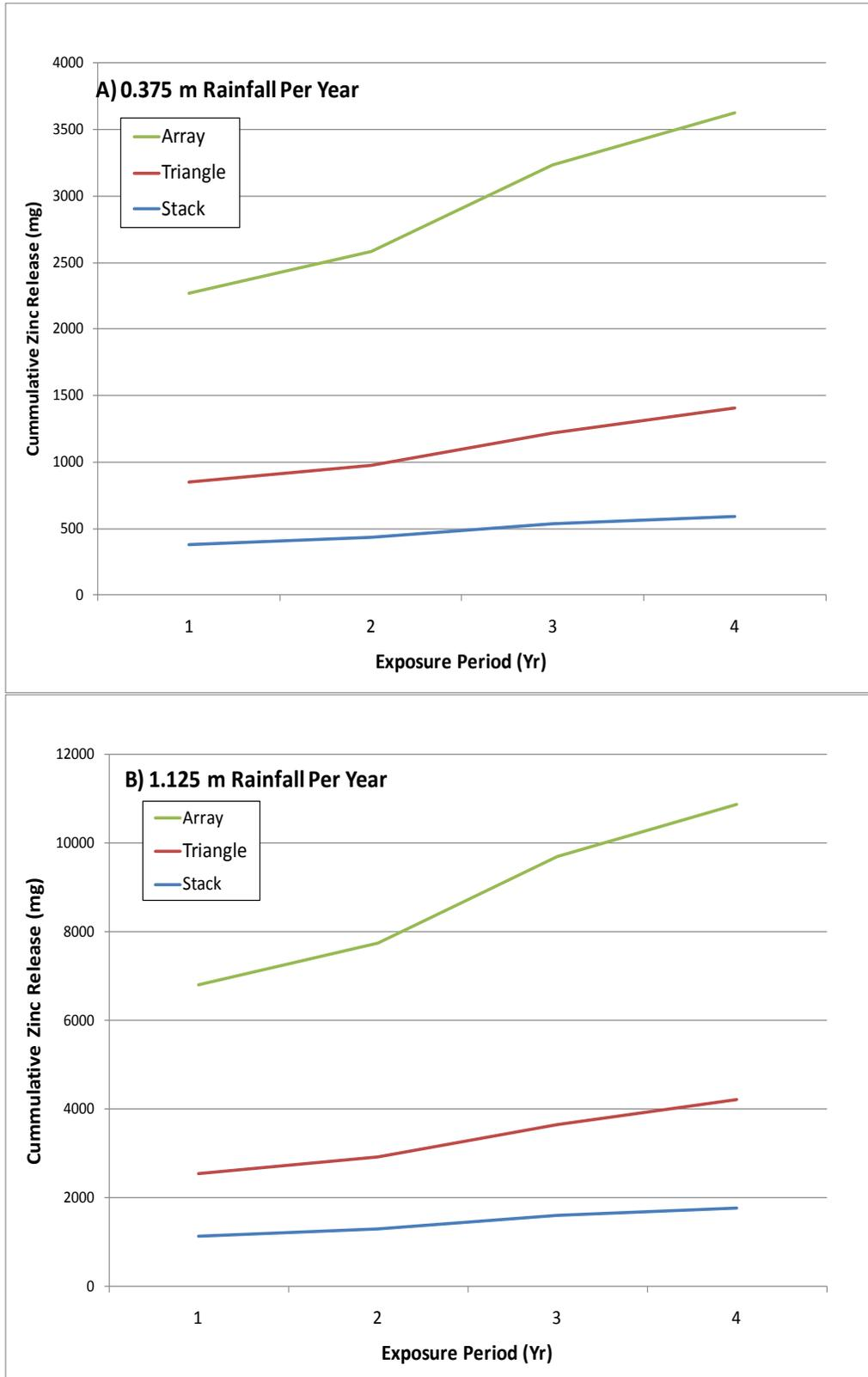
Figure VI- 9. Predicted zinc releases from 15 ACZA treated Douglas-fir poles stored for 4 years in one of three configurations and subjected to A.) low or B.) high rainfall.
