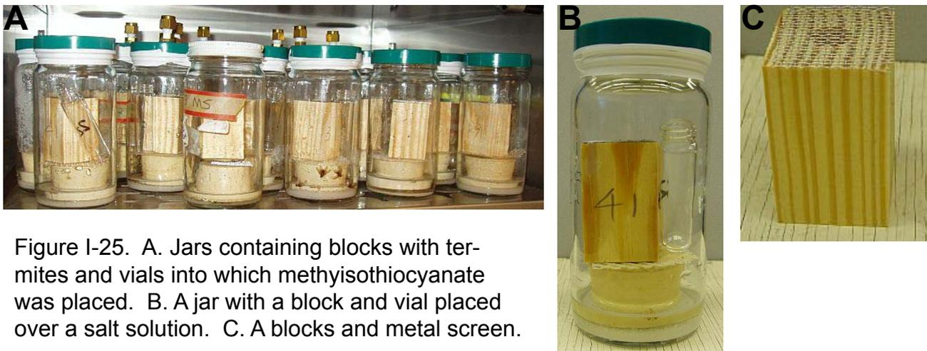
Figure I-25. A. Jars containing blocks with termites and vials into which methyisothiocyanate was placed. B. A jar with a block and vial placed over a salt solution. C. A blocks and metal screen.
