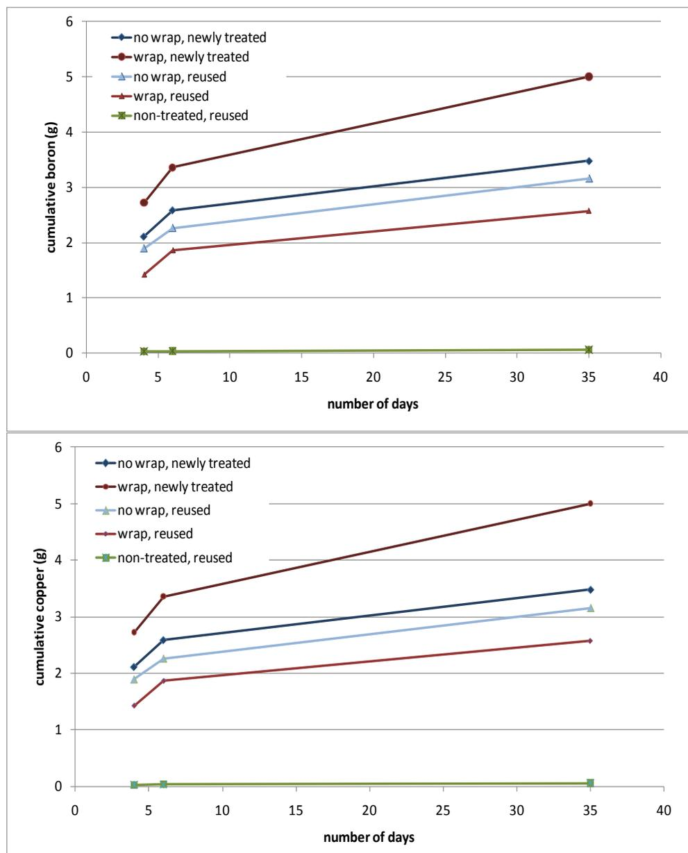
Figure IV-5. Boron and copper levels in rainfall runoff from posts treated with a boron/copper naphthenate paste with or without pasture wrap.
