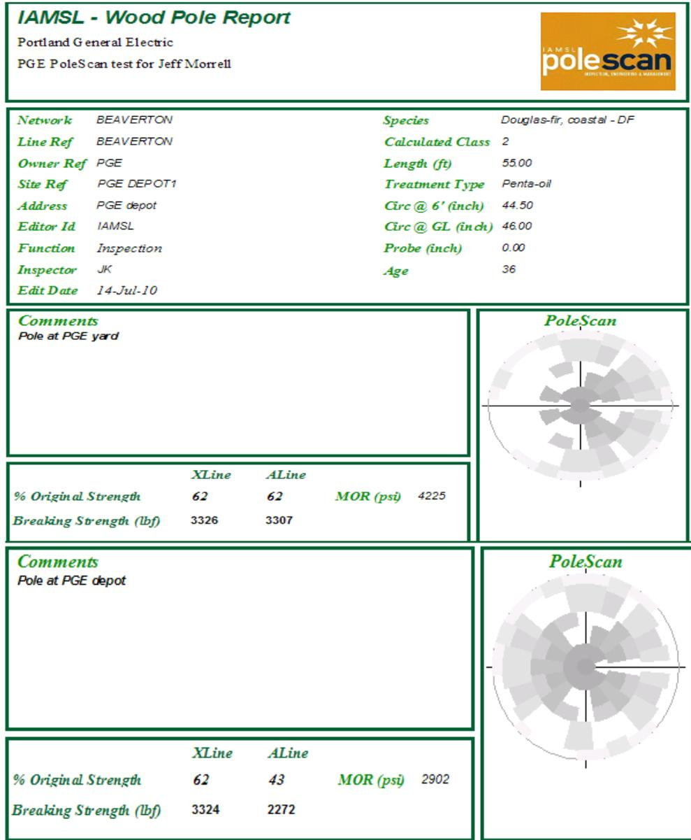
Figure III-12 continued. PoleScan output from above ground inspection of poles within the PGE system showing internal pole condition.
