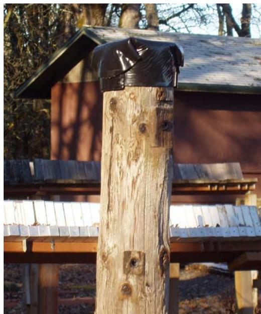
Figure III-13. Example of a capped pole (Osmose Pole Topper) used to assess the effects of capping on wood moisture content.
