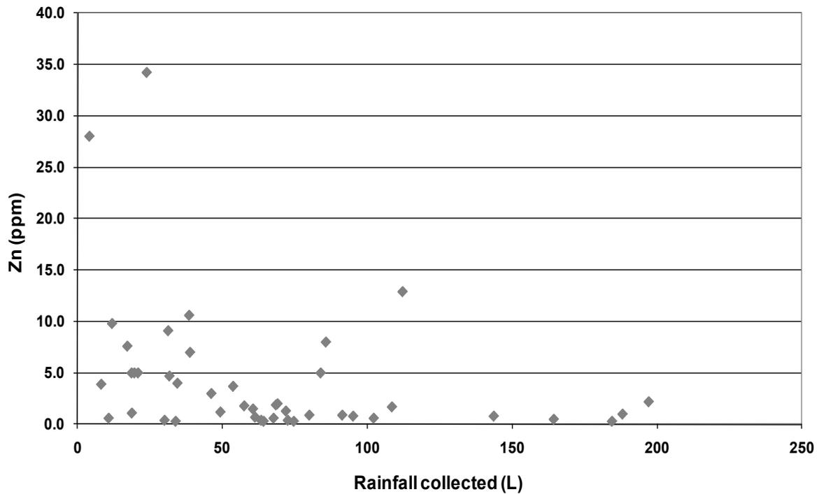
Figure VI-4. Zinc and copper levels in rainwater runoff from poles treated with ammoniacal copper zinc arsenate as a function of total rainfall collected.
