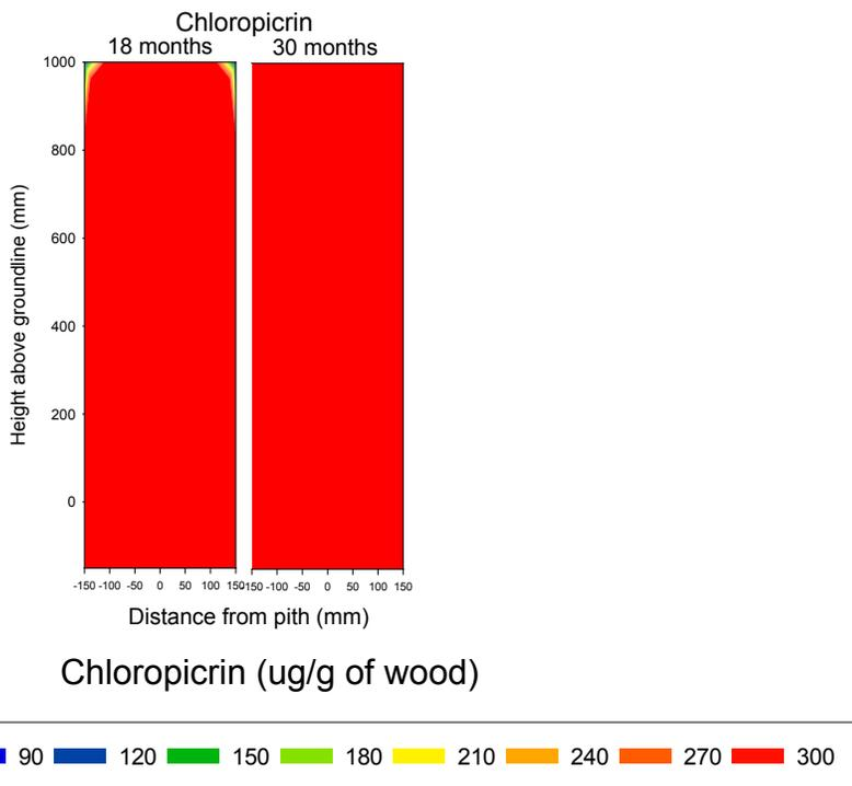
Figure I-23 Distribution of chloropicrin in Douglas-fir poles sections 18 and 30 months after treatment.
