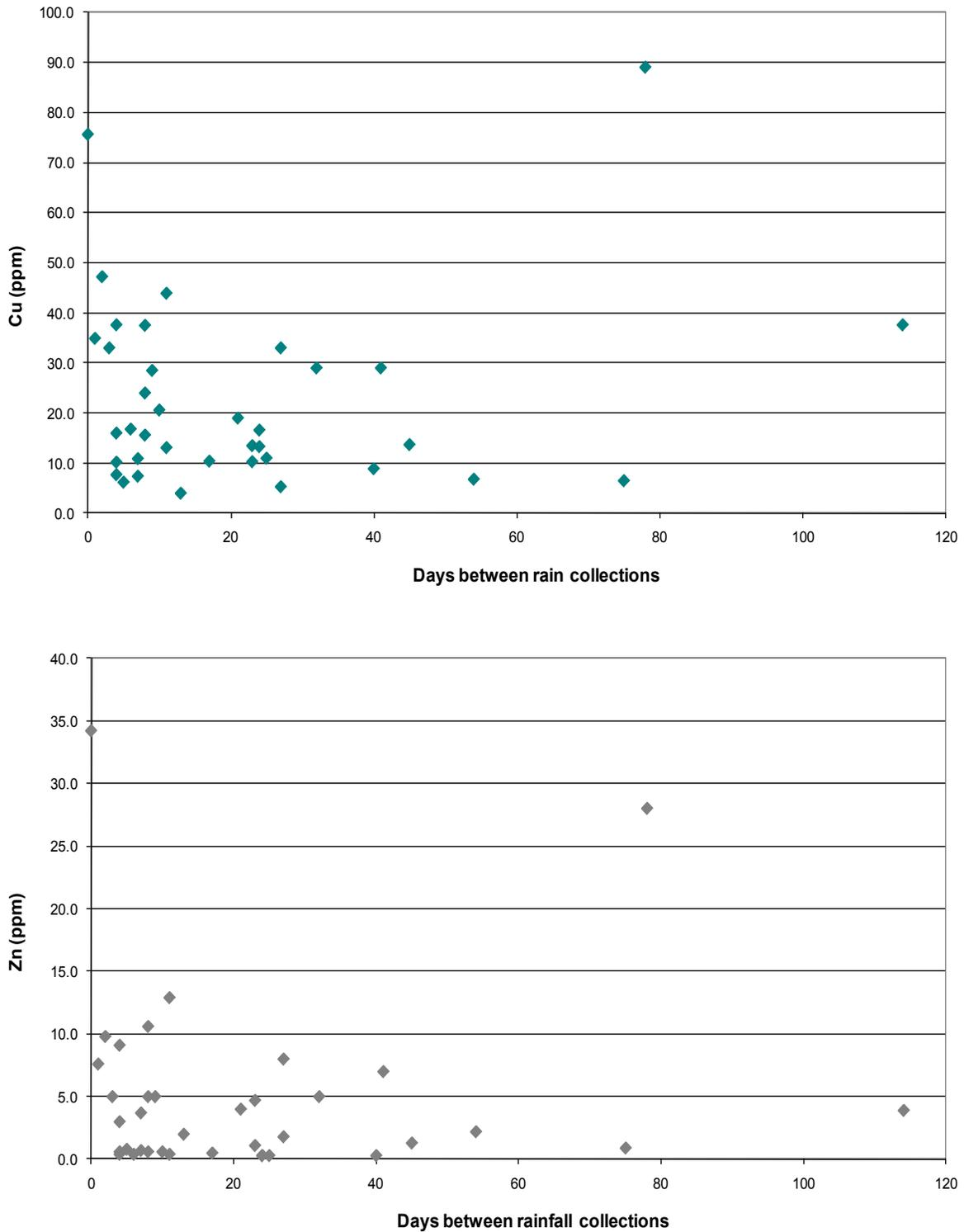
Figure VI-5. Zinc and copper levels in rainwater runoff from poles treated with ammoniacal copper zinc arsenate as a function of days between rainfall collections.
