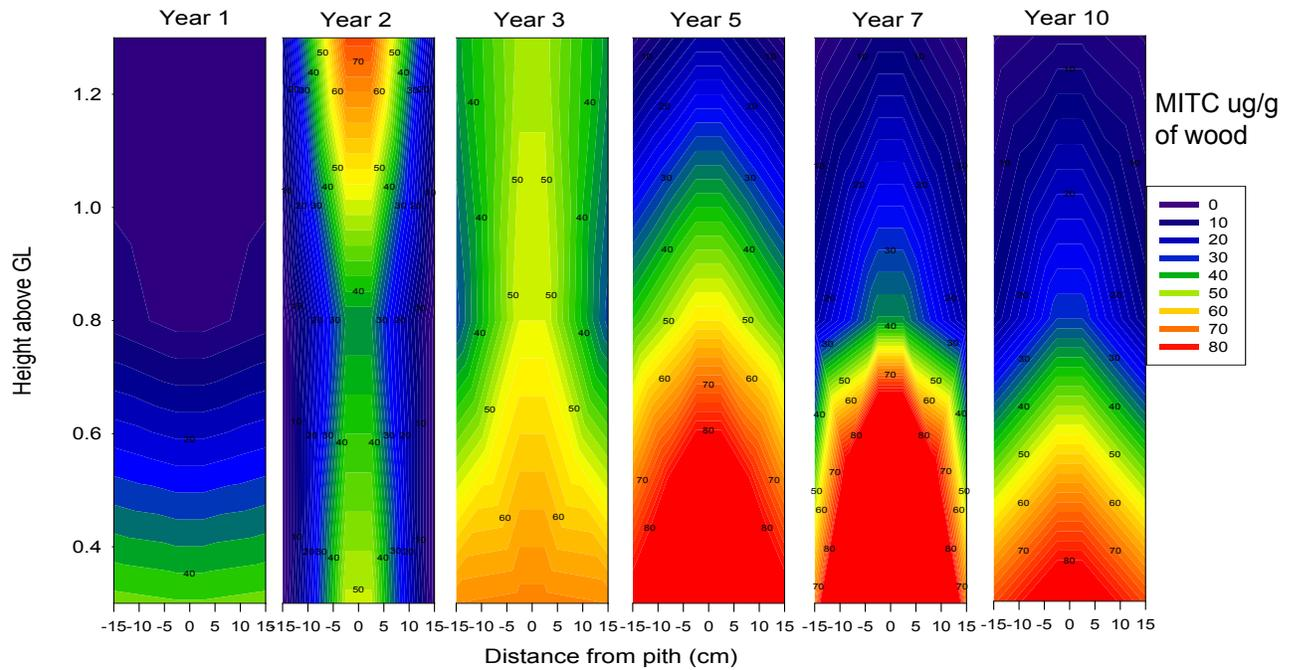
Figure I-6. Residual MITC in Douglas-fir poles 1 to 10 years after treatment with 6 dazomet rods (107 g) plus 100 g of copper naphthenate (2 % as Cu).
