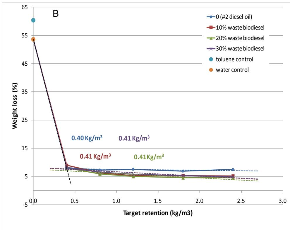
Figure V-6. Effect of waste oil-based biodiesel concentration in # 2 diesel on weight losses of A. weathered and B. non-weathered copper naphthenate treated blocks exposed to *G. trabeum* in an AWPA E10 soil block test.
