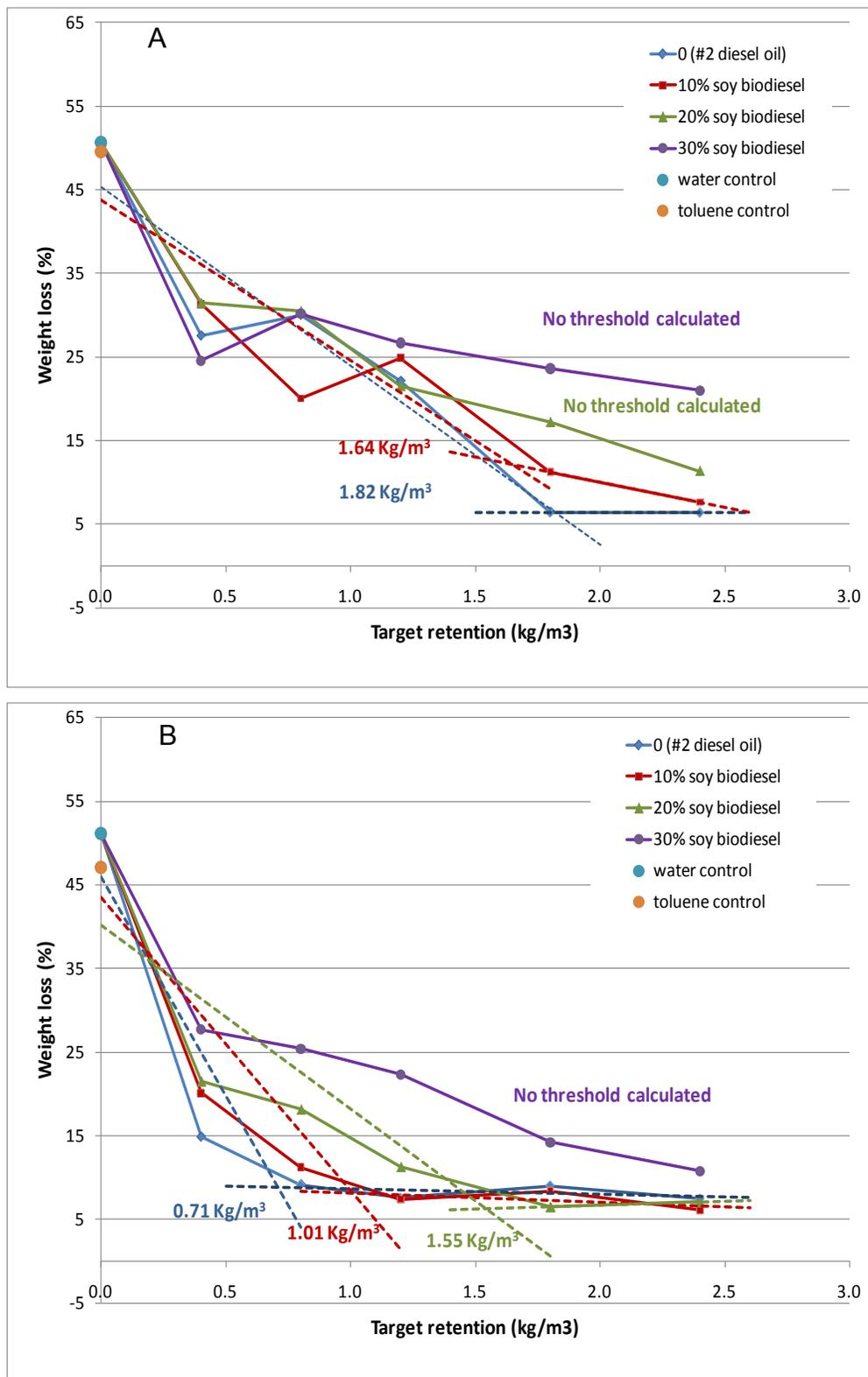
Figure V-3. Effect of soy-based biodiesel concentration in # 2 diesel on weight losses of A. weathered and B. non-weathered copper naphthenate treated blocks exposed to *P. placenta* in an AWWA E10 soil block test.
