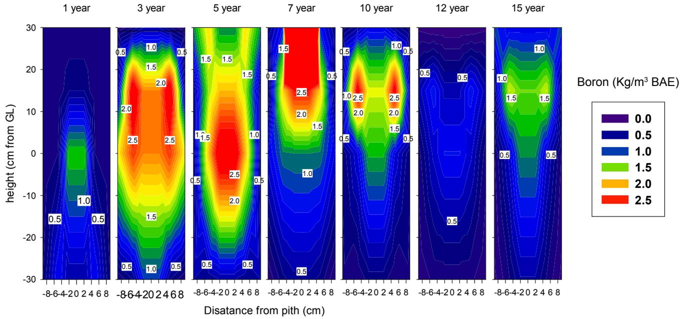
Figure I-13. Boron distribution (Kg/m<sup>3</sup> BAE) in Douglas-fir poles 1 to 15 years after treatment with fused boron rods.
