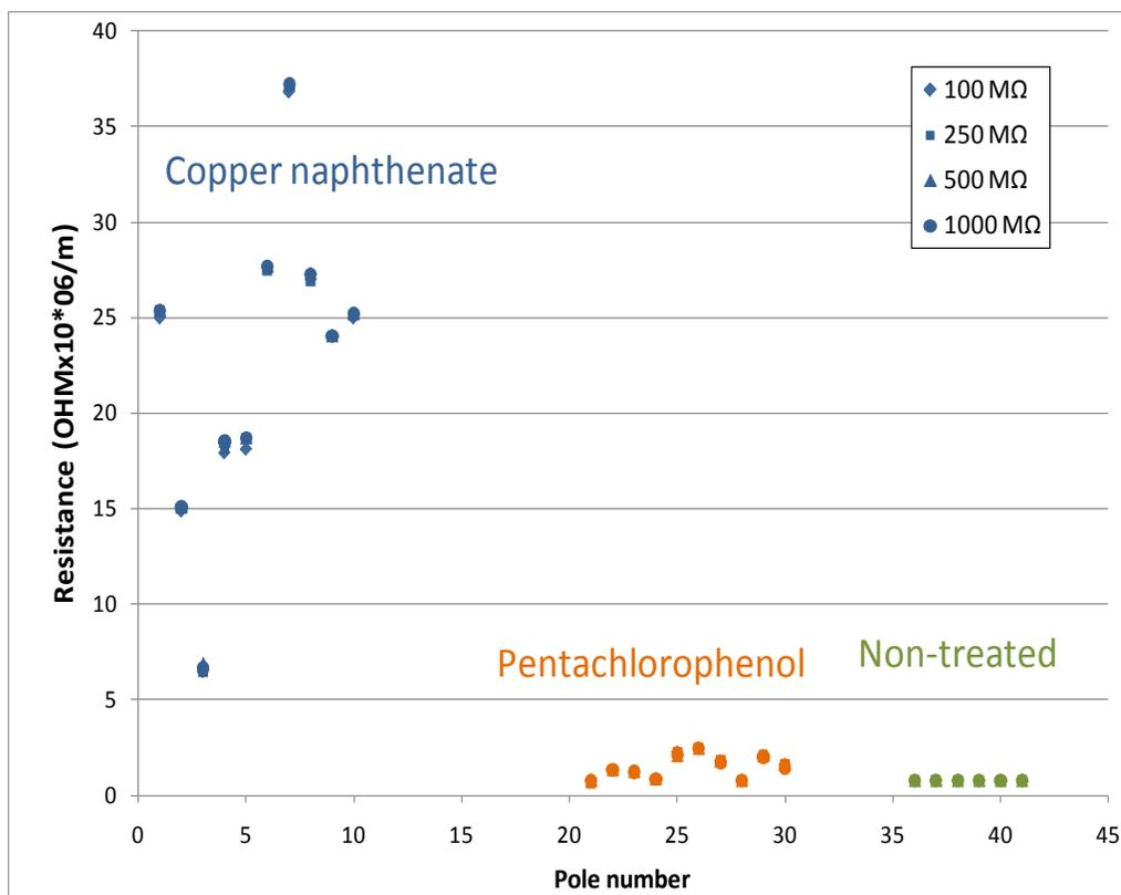
Figure III-17. Electrical resistance across Douglas-fir pole sections tested untreated or shortly after treatment with copper naphthenate or pentachlorophenol.
