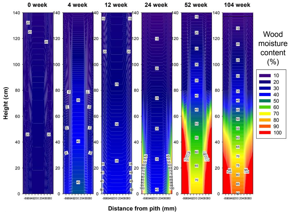
Figure IV-8. Moisture contents of copper naphthenate treated western redcedar poles wrapped with a UPC liner from the butt to the groundline and immersed in water for 0 to 104 weeks.
