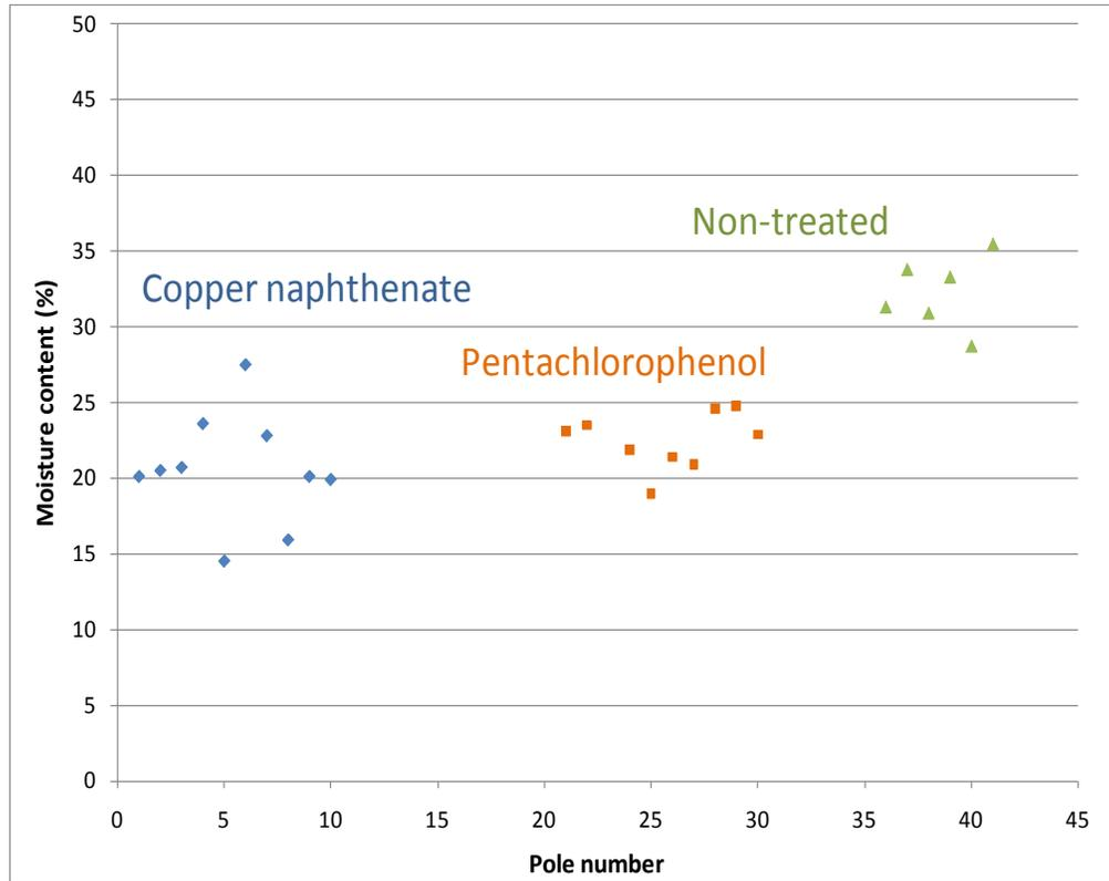
Figure III-18. Moisture contents vs voltages drops of Douglas-fir poles shortly treated with copper naphthenate or pentachlorophenol or left untreated and stored outdoors for 3 months.
