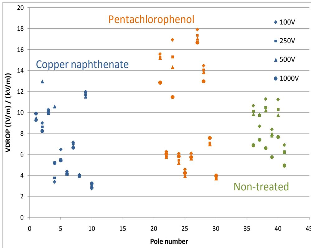
Figure III-19. Voltage drops across Douglas-fir pole sections that were untreated or treated with copper naphthenate or pentachlorophenol and stored outdoors for 3 months.
