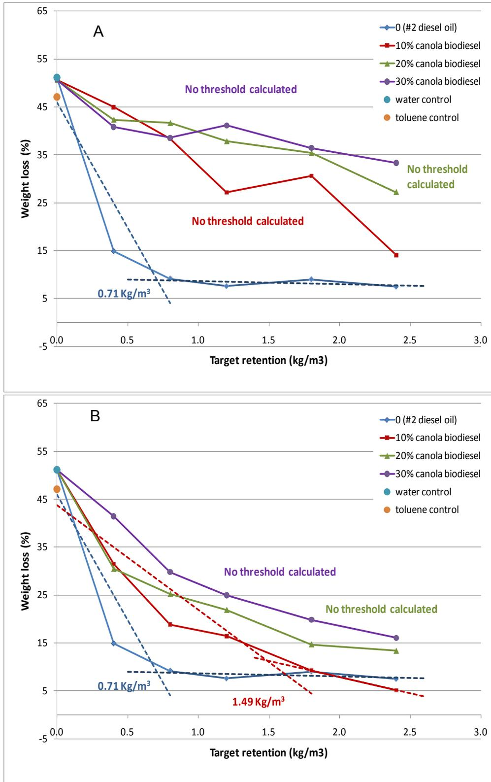
Figure V-7. Effect of canola oil-based biodiesel concentration in # 2 diesel on weight losses of A. weathered and B. non-weathered copper naphthenate treated blocks exposed to *P. placenta* in an AWPA E10 soil block test.
