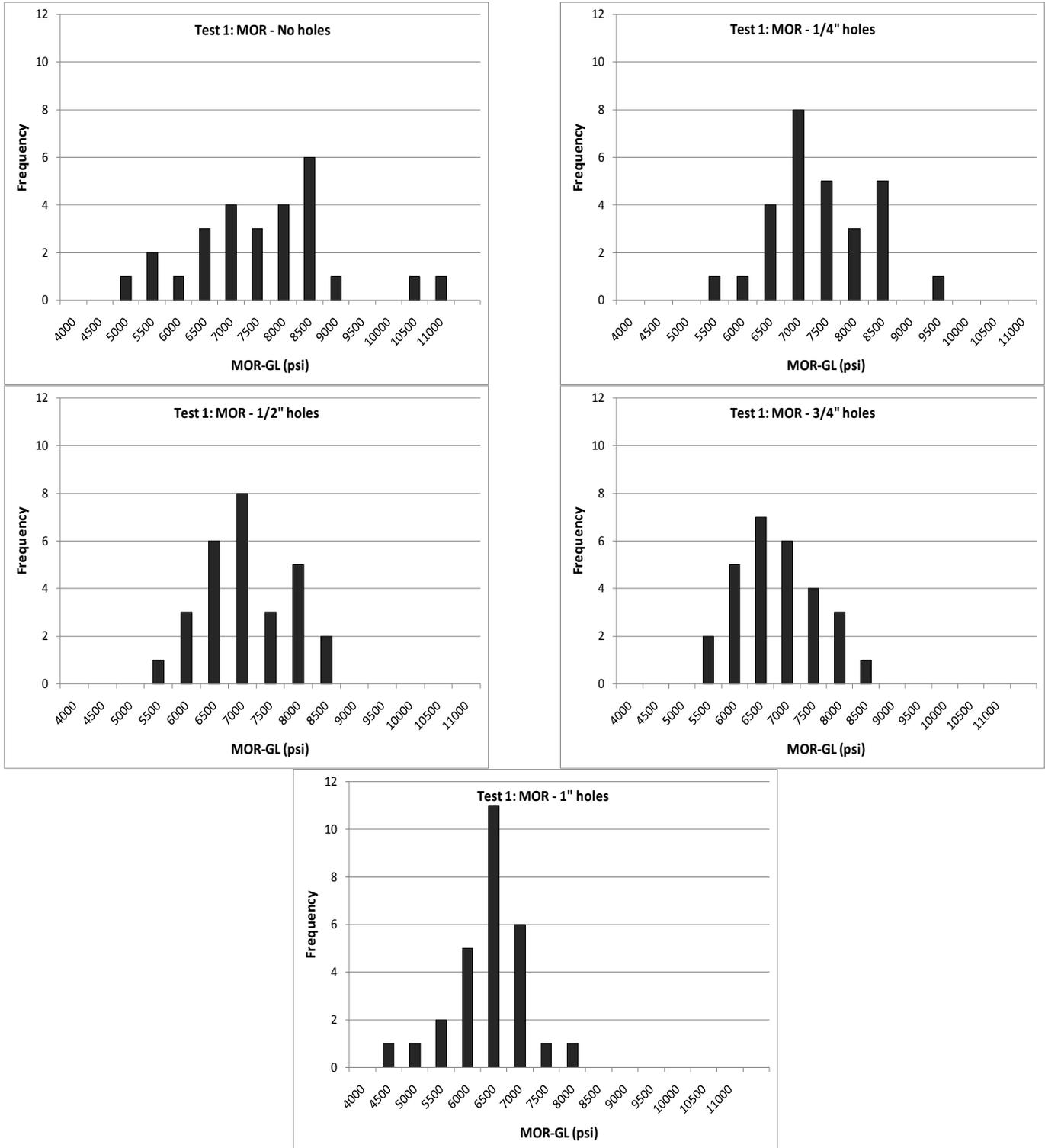
Figure III-3 MOR-GL distribution in Douglas-fir poles with or without 0.25, 0.50, 0.75 or 1.00 inch diameter through-boring holes in the groundline region.
