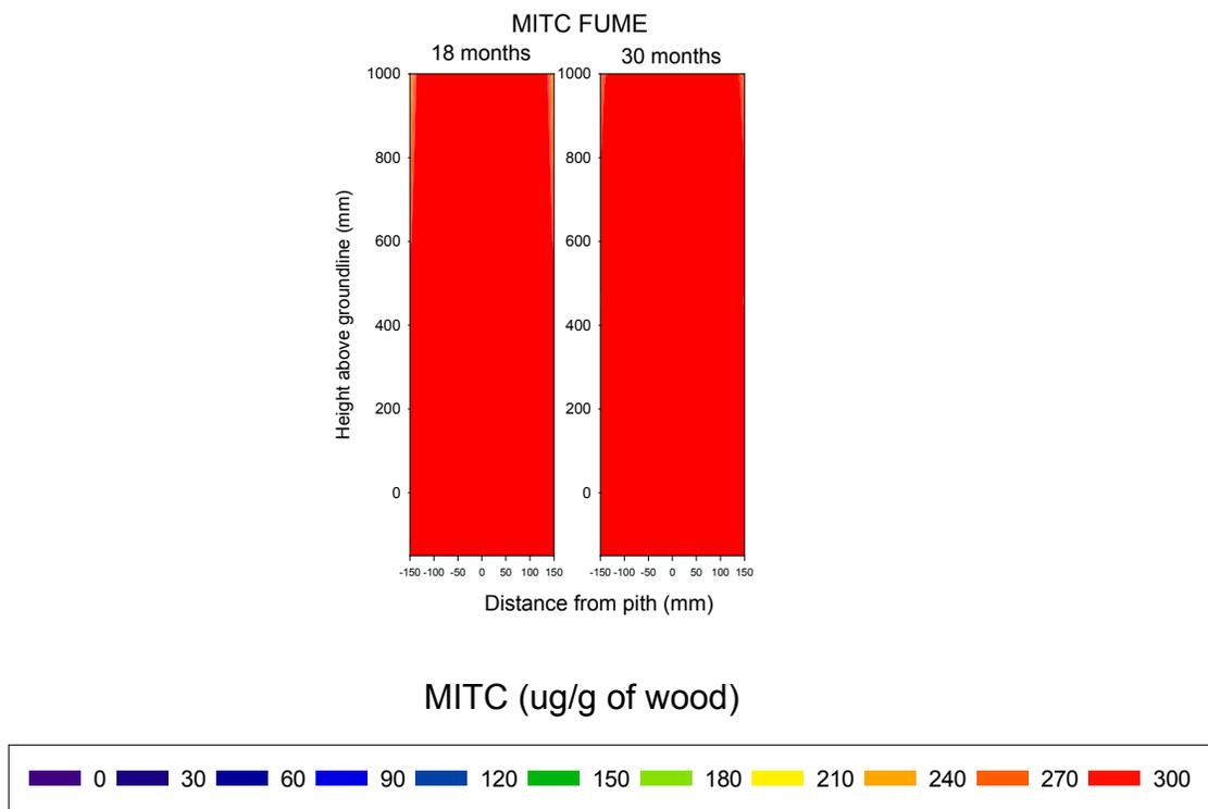
Figure I-21 Distribution of MITC in Douglas-fir poles sections 18 and 30 months after treatment with MITC-FUME.
