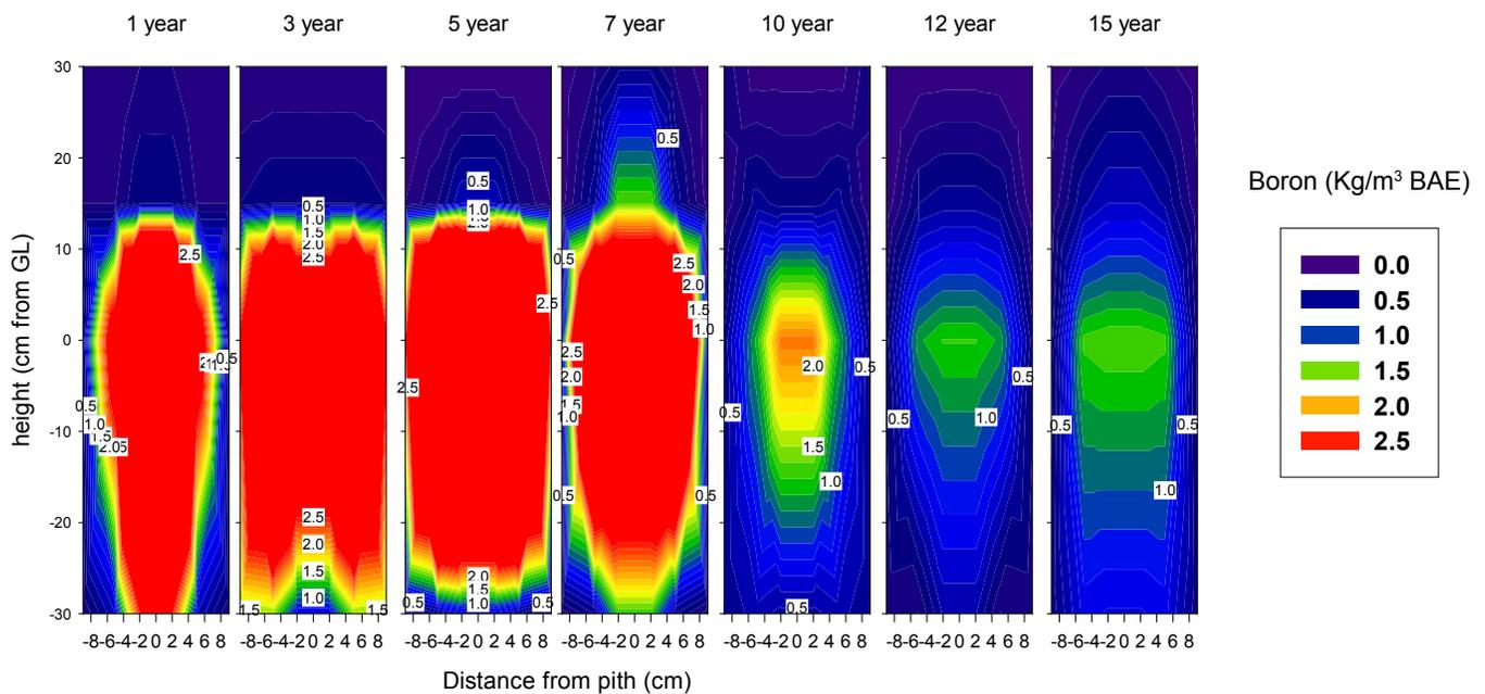
Figure I-16. Boron distribution (Kg/m<sup>3</sup> BAE) in Douglas-fir poles 1 to 15 years after treatment with fused boron rods and Boracol 40.
