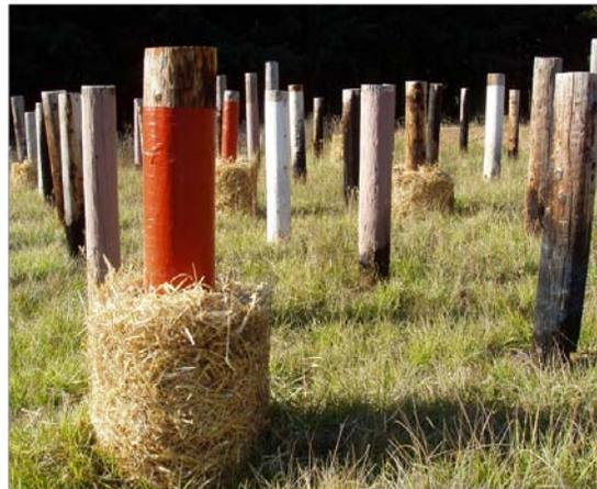
Figure III-5. Example of a pole section with straw fuel in a wire cage prior to ignition.
