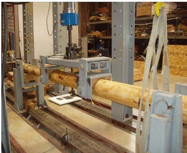
Figure III-1. Photograph showing a pole in the test set-up.
