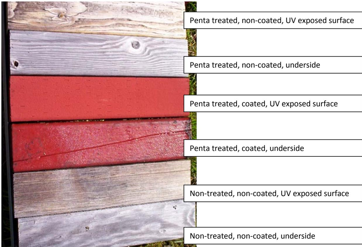
Figure III-7. Examples of coated and non-coated Douglas-fir cross arm sections after 1 year of exposure near Hilo, Hawaii.
