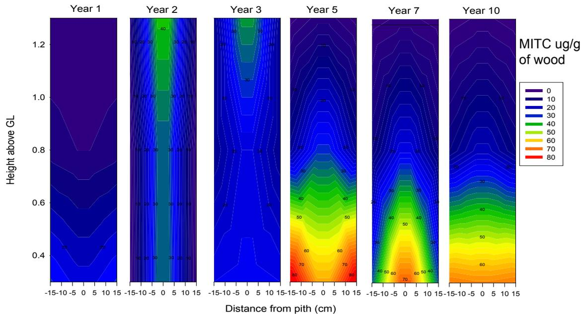
Figure I-9. Residual MITC in Douglas-fir poles 1 to 10 years after treatment with 9 dazomet rods (160 g) plus 100 g of water .
