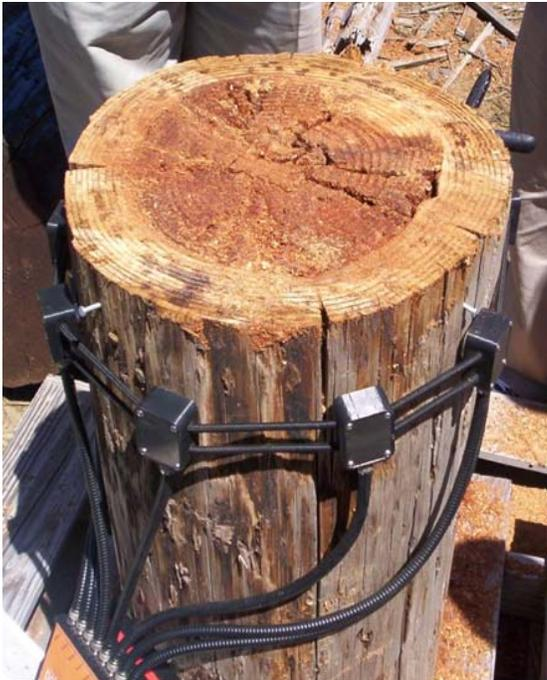
Figure III-11. PoleScan device attached to a Douglas-fir pole section showing the multiple sampling points as well as a large internal decay pocket.
