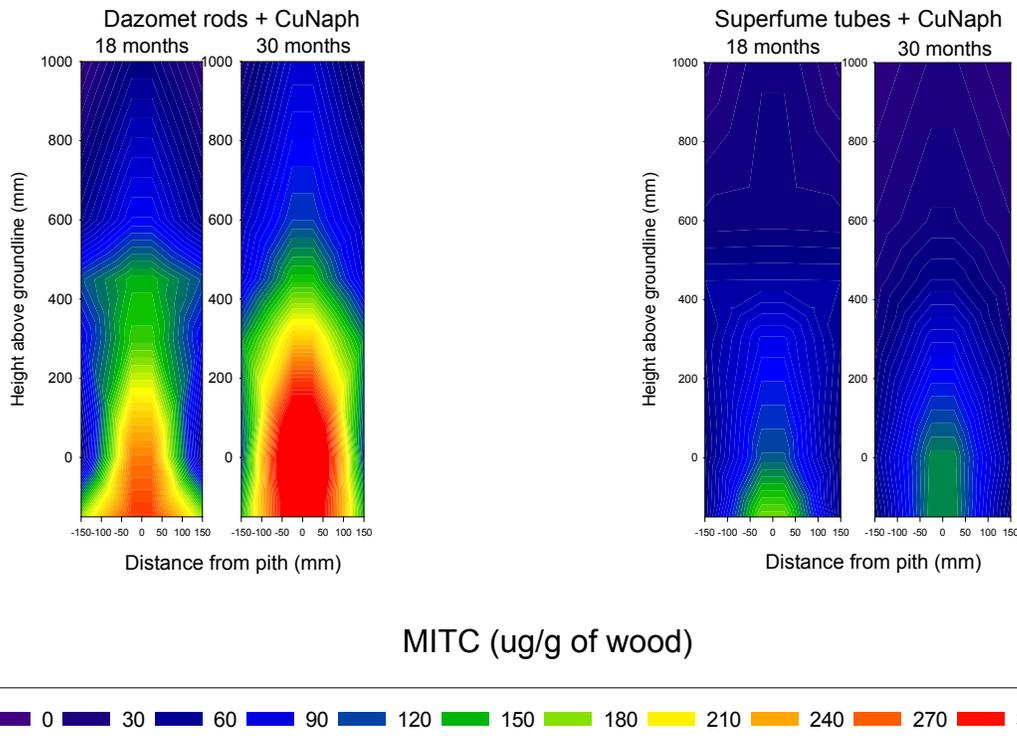
Figure I-20. Distribution of MITC in Douglas-fir poles sections 18 and 30 months after treatment with dazomet rods plus copper naphthenate or SUPER-FUME tubes plus copper naphthenate.
