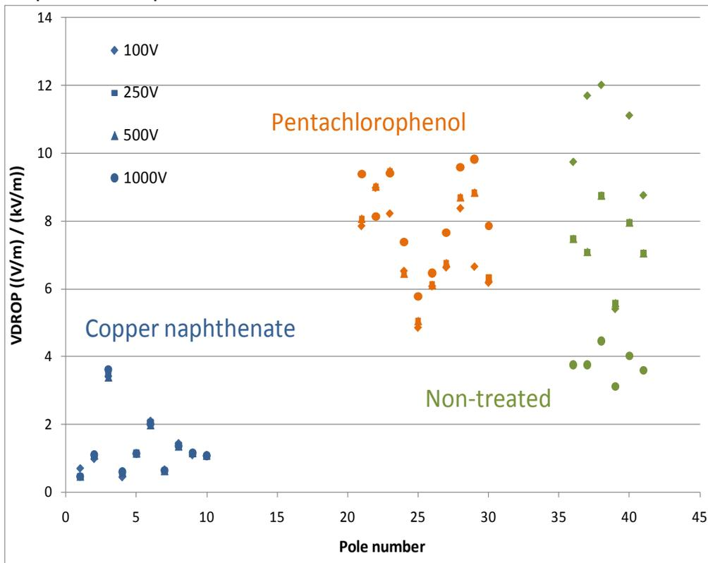
Figure III-16. Voltage drops across Douglas-fir pole sections tested untreated or shortly after treatment with copper naphthenate or pentachlorophenol.
