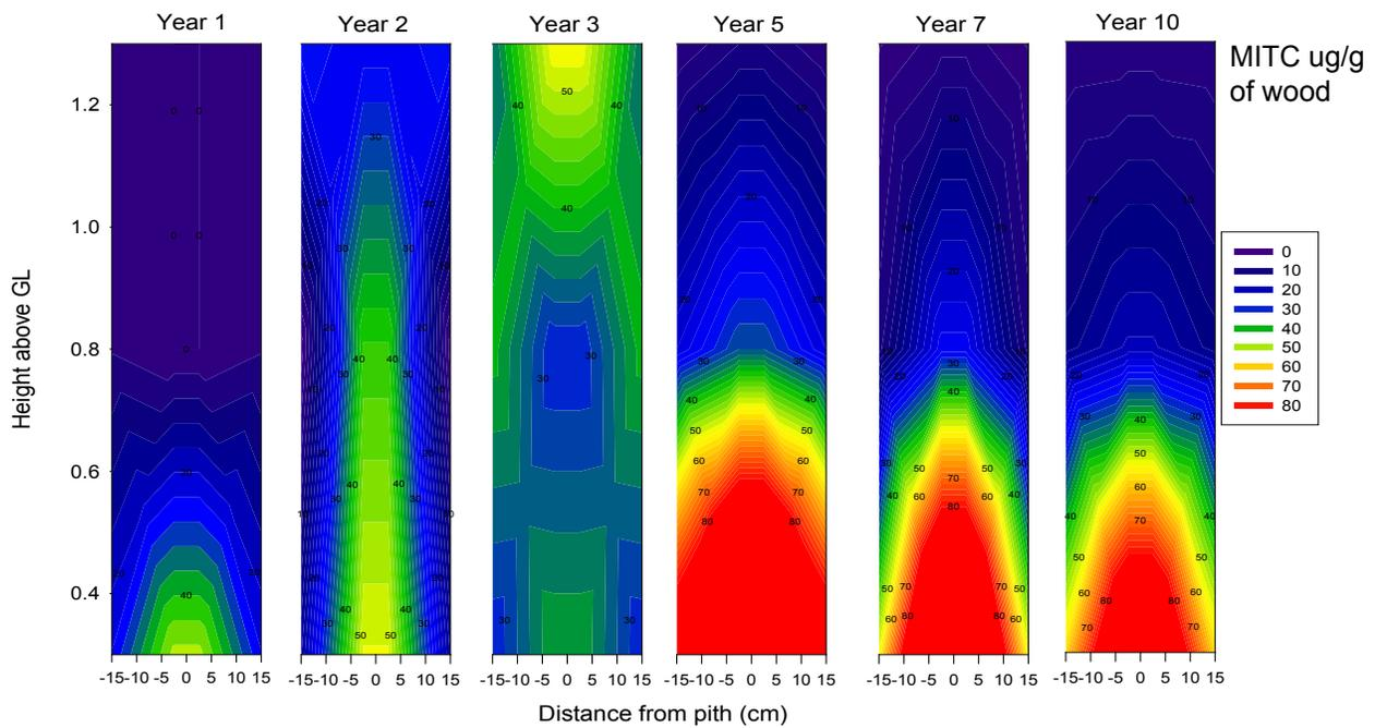
Figure I-5. Residual MITC in Douglas-fir poles 1 to 10 years after treatment with 160 g of powdered dazomet.
