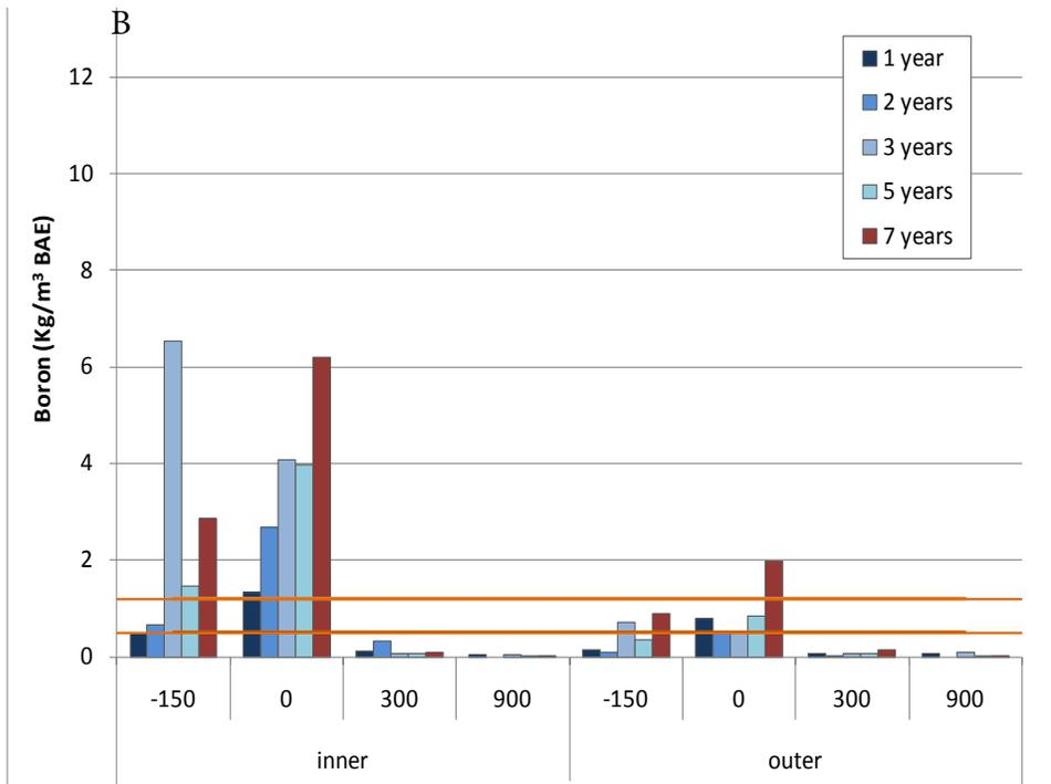
Figure I-11 Residual boron levels in Douglas-fir poles 1 to 7 years after application of A. 4 or B. 8 fused borate/copper rods in treatment holes spaced at 90 degree intervals around each pole.
