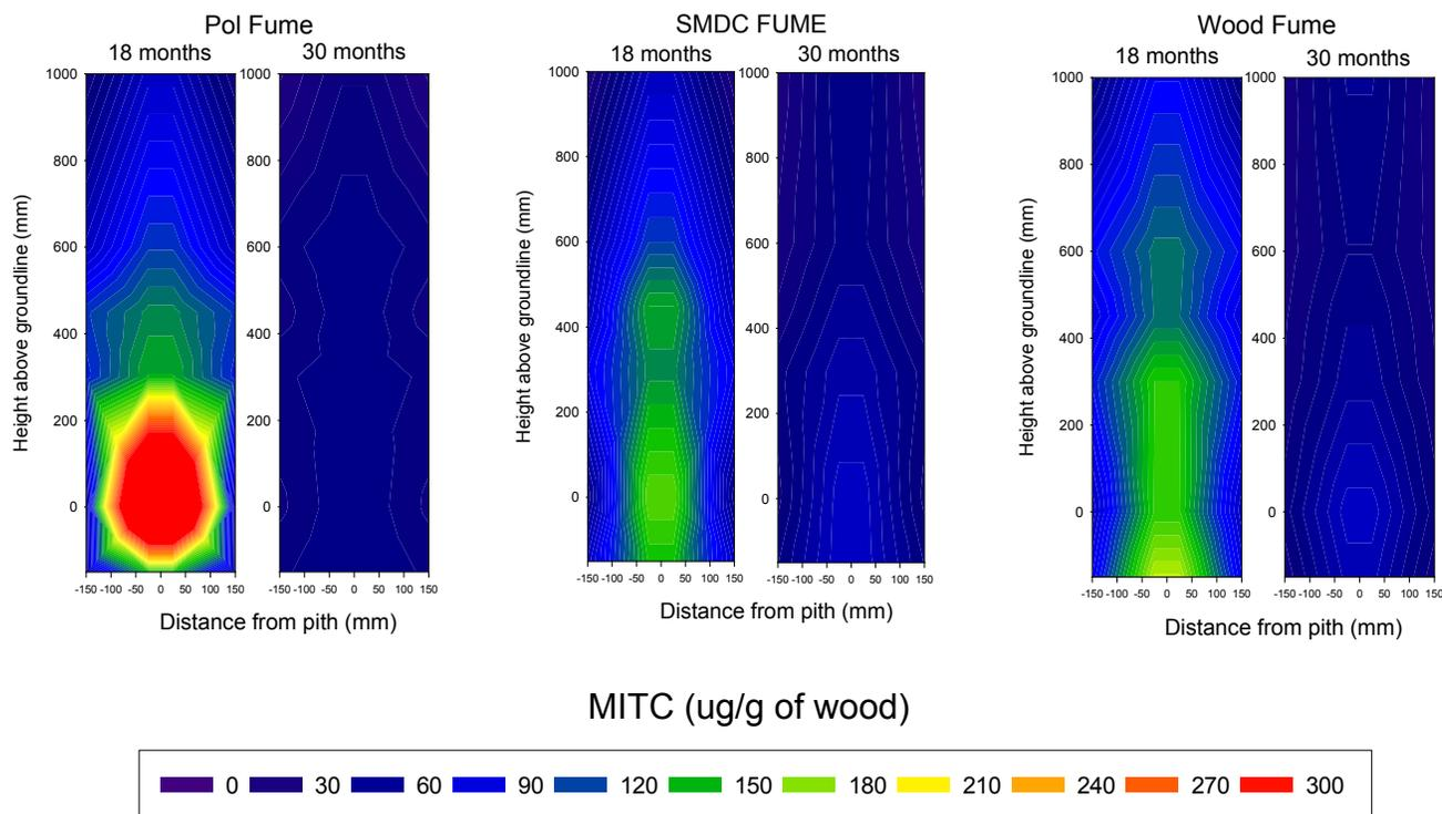
Figure I-22. Distribution of MITC in Douglas-fir poles sections 18 and 30 months after treatment with Pol-Fume, SMDC-Fume, or WoodFume.
