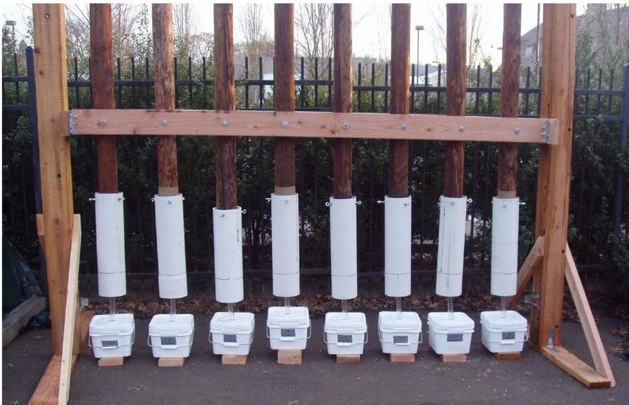
Figure IV-4 Assembly used to capture water running down post sections treated with a boron/copper naphthenate preservative paste.
