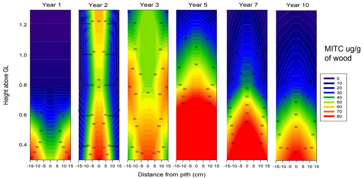
Figure I-8. Residual MITC in Douglas-fir poles 1 to 10 years after treatment with 9 dazomet rods (160 g) plus 100 g of copper naphthenate.
