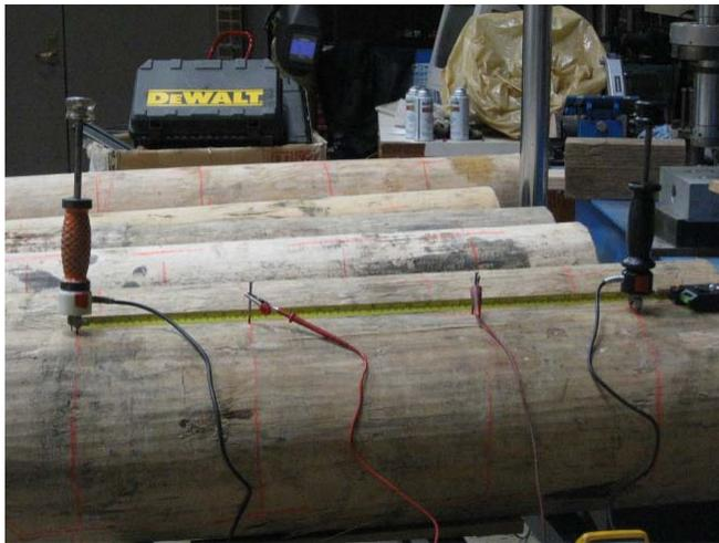
Figure III-14. Locations of moisture meter pins and nails used to measure conductivity and resistance, respectively, in Douglas-fir pole sections treated with pentachlorophenol or copper naphthenate.
