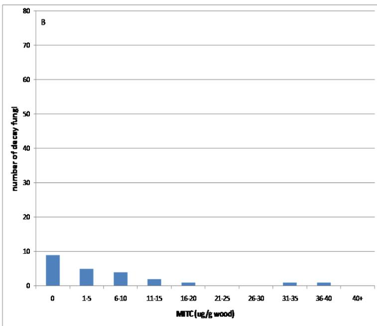
Figure I-2. Comparison between the lowest MITC value obtained from a core and the frequency of isolation of a decay fungus from A. Douglas-fir or B. southern pine poles treated with met-tam sodium or varying levels of MITC-FUME in the original MITC-FUME test.
