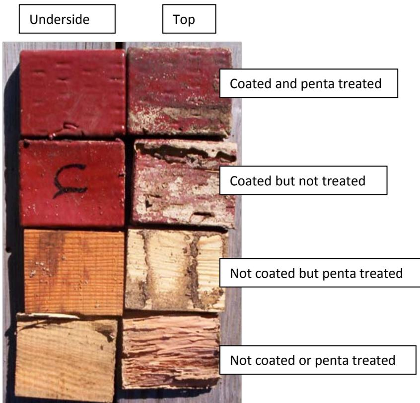
Figure III-8. Examples of undersides (top) and upper surfaces of coated and non-coated Douglas-fir lumber with and without penta treatment.
