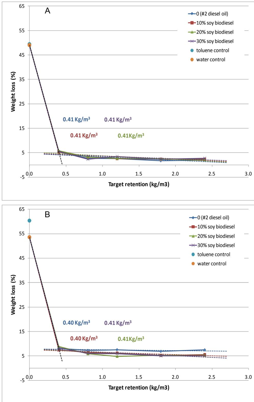
Figure V-4. Effect of soy-based biodiesel concentration in # 2 diesel on weight losses of A. weathered and B. non-weathered copper naphthenate treated blocks exposed to *G. trabeum* in an AWPA E10 soil block test.
