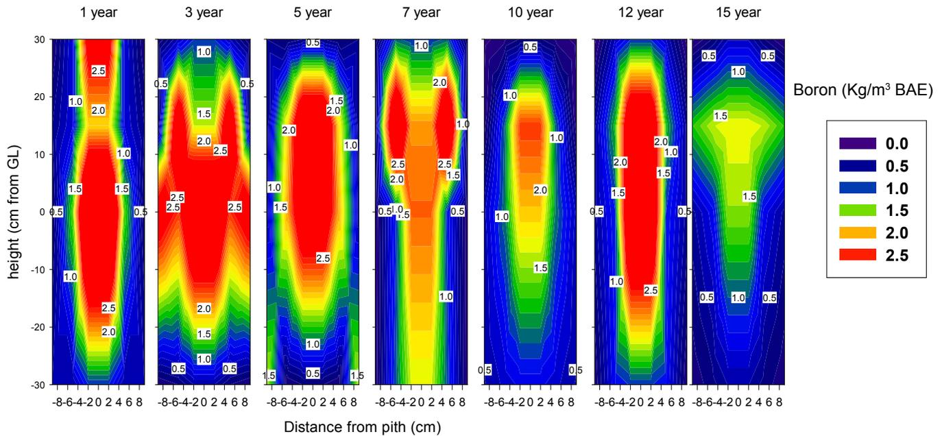
Figure I-15. Boron distribution (Kg/m<sup>3</sup> BAE) in Douglas-fir poles 1 to 15 years after treatment with fused boron rods and Boracol 20.
