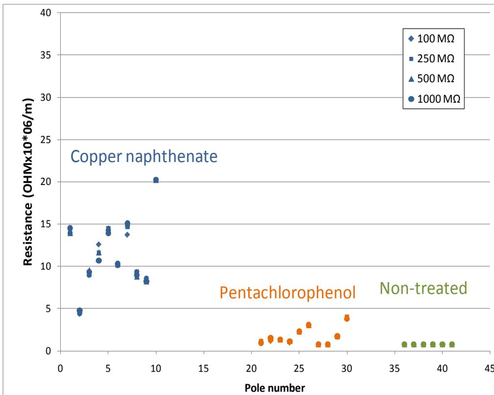
Figure III-20. Electrical resistance across Douglas-fir pole sections untreated or treated with copper naphthenate or pentachlorophenol and stored outdoors for 3 months.
