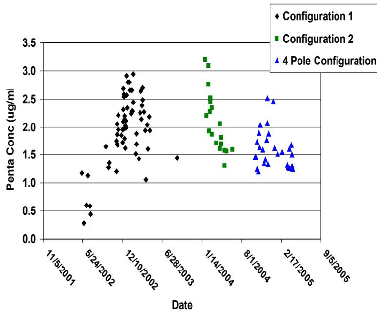
Figure VI-2. Penta concentrations as a function of sampling date in leachate collected from penta treated Douglas-fir poles following rainfall events over a 4.5 year exposure period showing data for three stacking configurations of poles.
