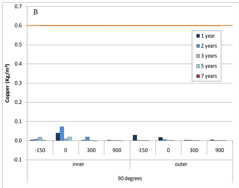
Figure I-12. Residual copper levels in Douglas-fir poles 1 to 7 years after application of A. 4 or B. 8 fused borate/copper rods in treatment holes spaced at 90 degree intervals around each pole.
