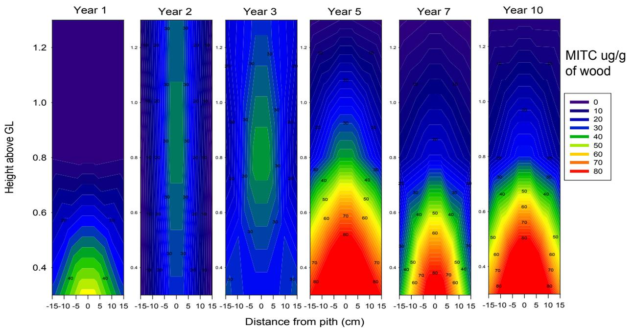
Figure I-7. Residual MITC in Douglas-fir poles 1 to 10 years after treatment with 9 dazomet rods (160 g).
