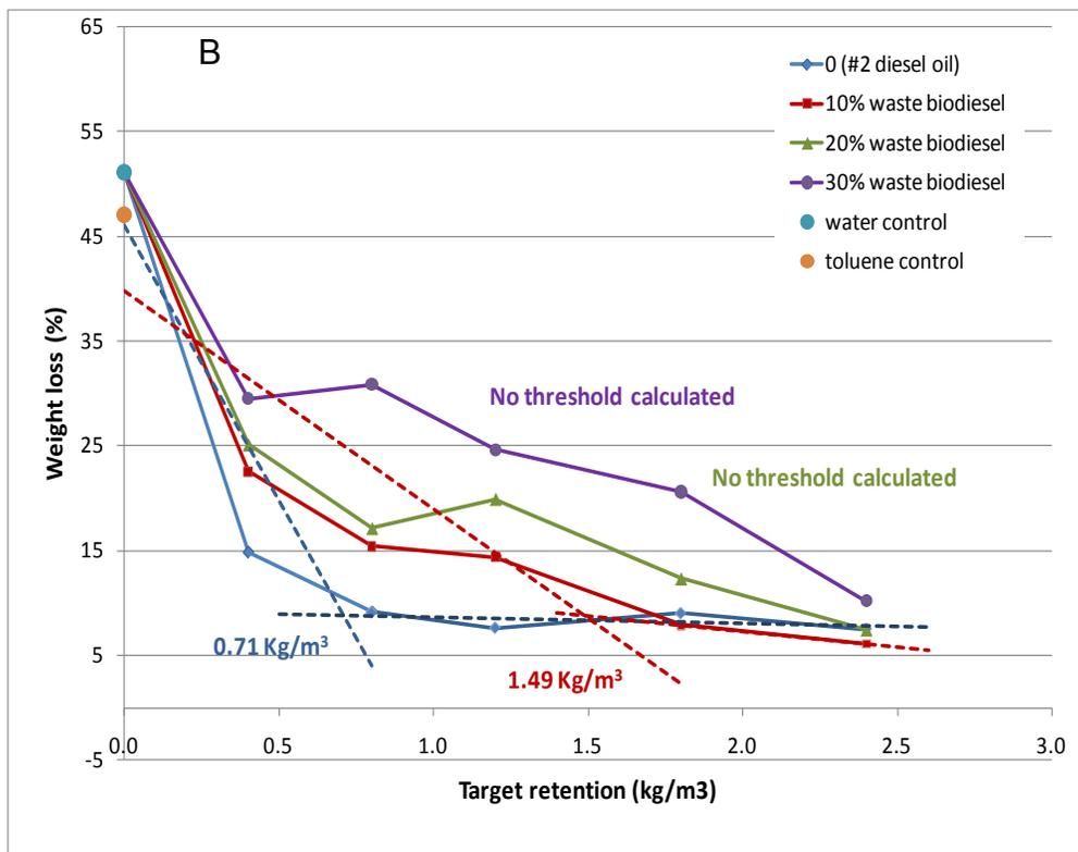
Figure V-5. Effect of waste oil-based biodiesel concentration in # 2 diesel on weight losses of A. weathered and B. non-weathered copper naphthenate treated blocks exposed to *P. placenta* in an AWPA E10 soil block test.
