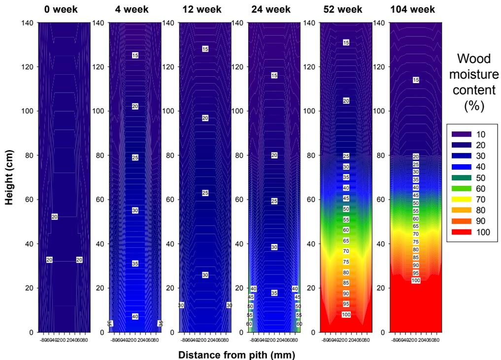
Figure IV-9. Moisture contents of copper naphthenate treated western redcedar poles wrapped with a UPC liner from the butt to the groundline and immersed in moist soil for 0 to 104 weeks.
