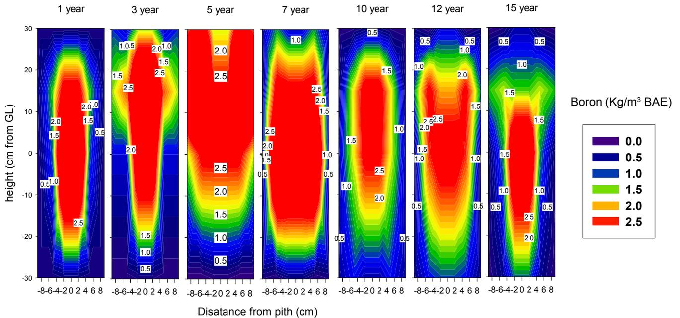
Figure I-17. Boron distribution (Kg/m<sup>3</sup> BAE) in Douglas-fir poles 1 to 15 years after treatment with fused boron rods and glycol.
