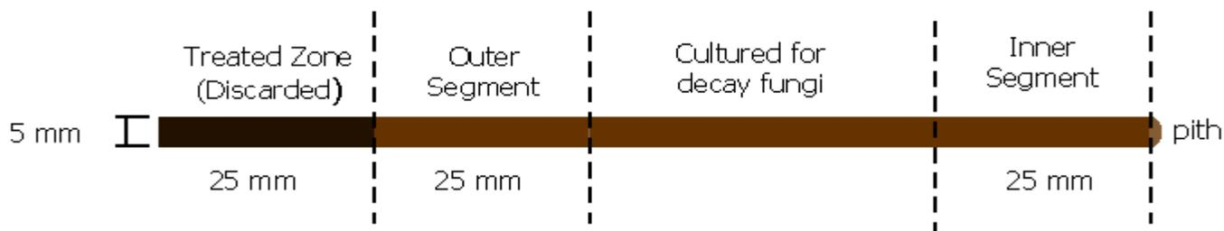
Figure I-3. Representation of increment core showing inner and outer 25 mm segments analyzed for fumigant content. The length of the segment cultured for decay fungi varies in length depending on the size of the pole.
