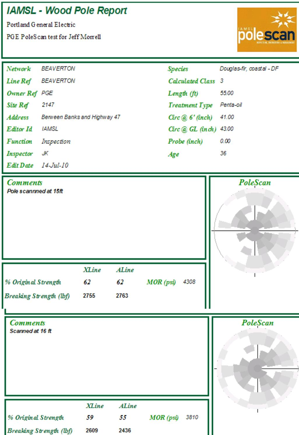
Figure III-12. PoleScan output from above ground inspection of poles within the PGE system showing internal pole condition.
