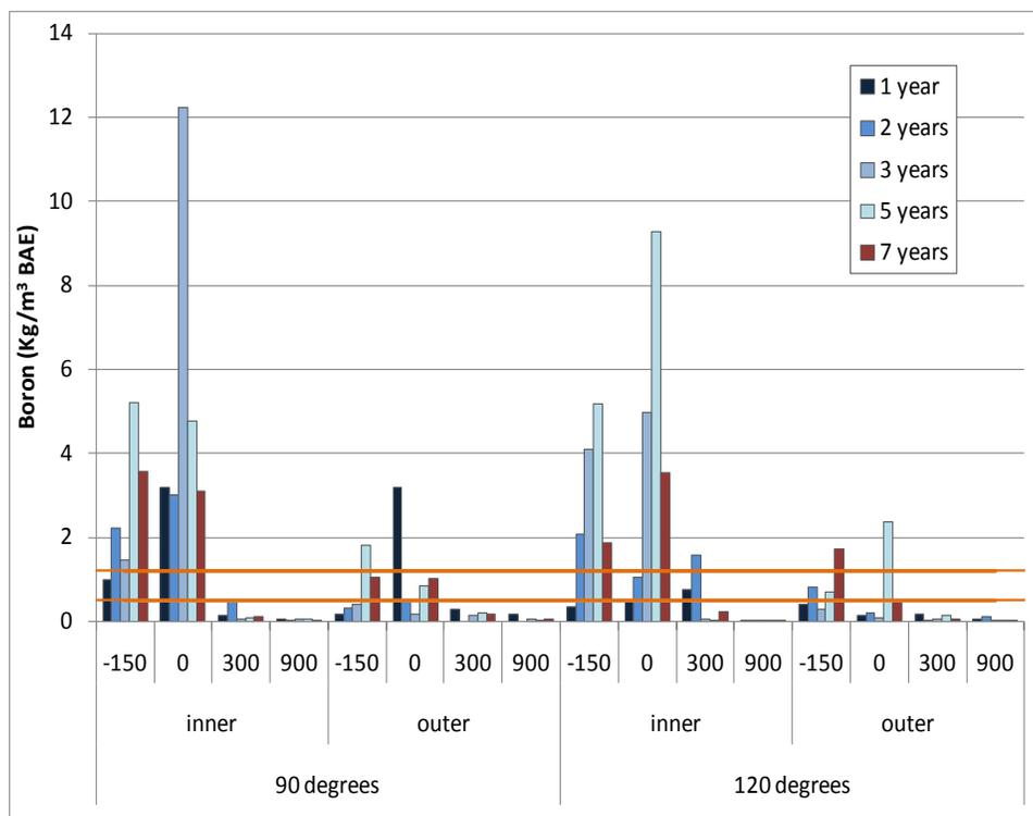
Figure I-10 Residual boron levels in Douglas-fir poles 1 to 7 years after application of 4 fused boron rods in treatment holes spaced at either 90 or 120 degree intervals around each pole.
