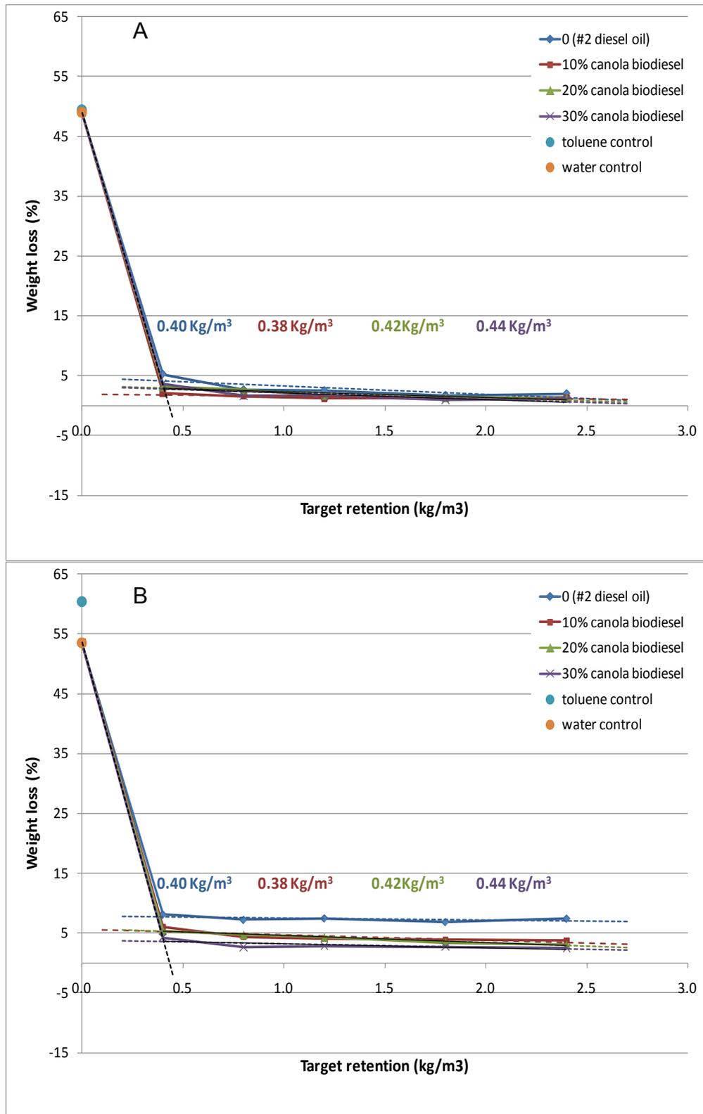
Figure V-8. Effect of canola oil-based biodiesel concentration in # 2 diesel on weight losses of A. weathered and B. non-weathered copper naphthenate treated blocks exposed to *G. trabeum* in an AWP A E10 soil block test.
