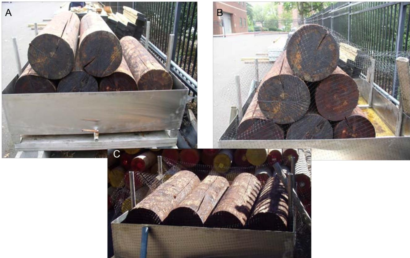
Figure VI-1. Photo showing the two six-pole configurations. A. configuration 1, B. configuration 2, and C. the four pole configuration in our small scale preservative migration chamber.
