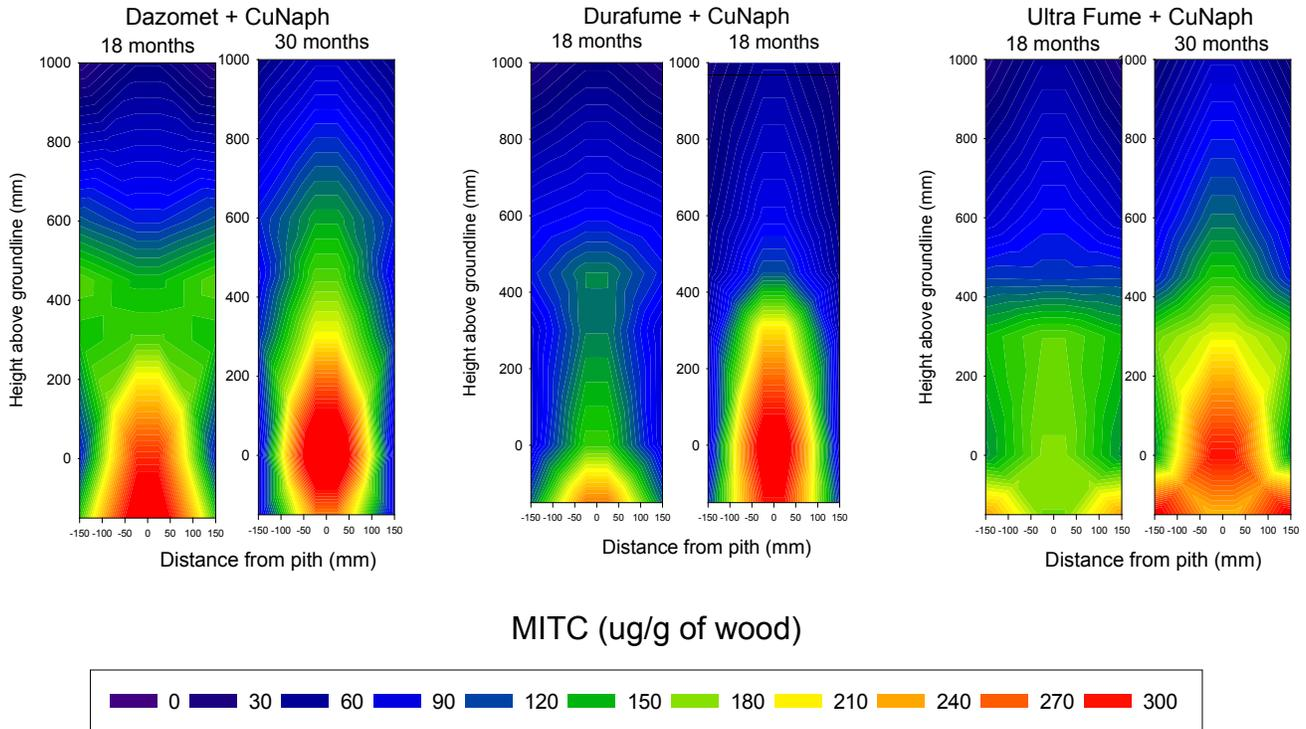
Figure I-19. Distribution of MITC in Douglas-fir poles sections 18 and 30 months after treatment with dazomet plus copper naphthenate, DuraFume plus copper naphthenate or UltraFume plus copper naphthenate.
