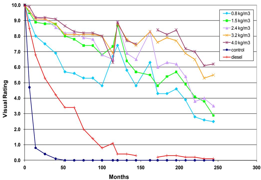
Figure V-2. Condition of weathered western redcedar sapwood stakes treated with selected retentions of copper naphthenate in diesel oil and exposed in a soil bed for 244 months.
