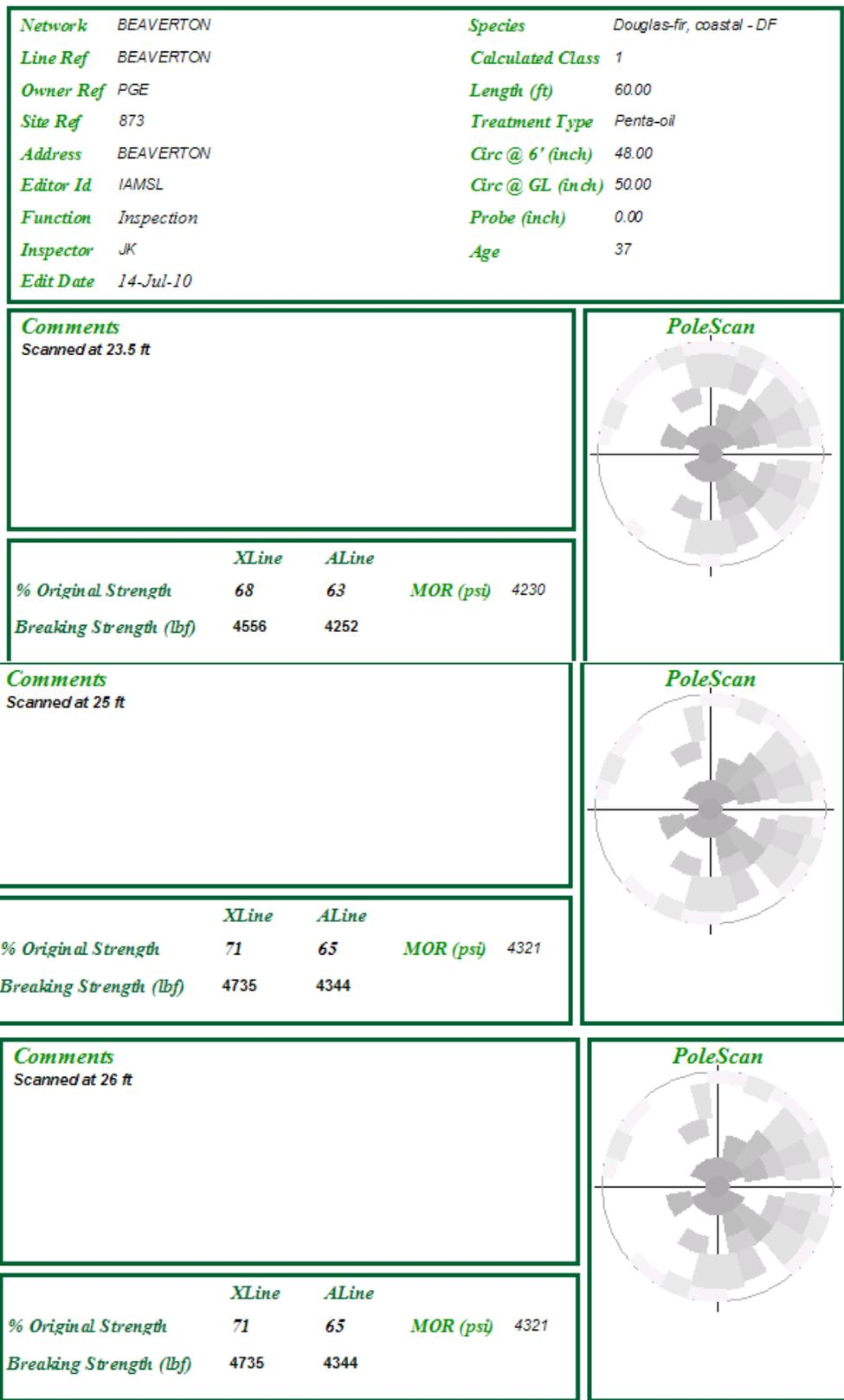
Figure III-12 continued. PoleScan output from above ground inspection of poles within the PGE system showing internal pole condition.
