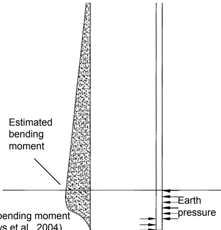
Figure III-2. Estimated true bending moment for an embedded pole (Crews et al., 2004).
