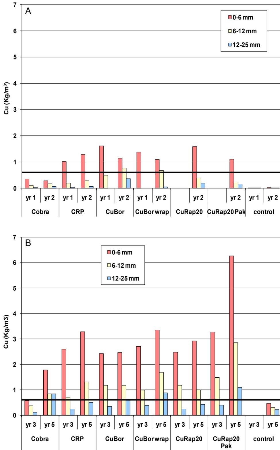
Figure IV-1. Copper levels in southern pine poles A. 1 and 2 and B. 3 and 5 years after application of various external supplemental preservatives.
