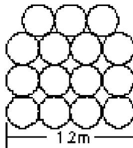
Figure VI-7. Configurations of 15 Class 4 forty foot long poles used to model predicted copper and zinc concentrations in soil beneath ACZA treated poles as a result of rainwater runoff. Poles were configured as 15 individual poles, poles in a triangular stack and poles in four courses with stickers in between each course.
