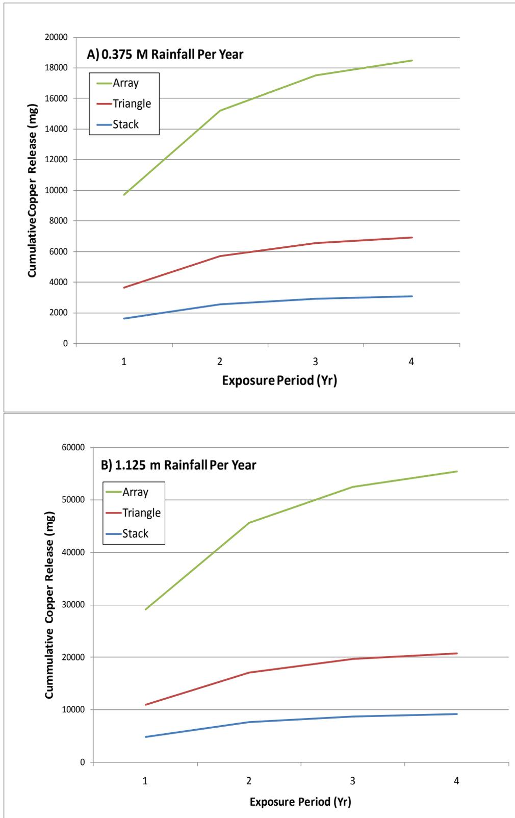
Figure VI-8. Predicted copper releases from 15 ACZA treated Douglas-fir poles stored for 4 years in one of three configurations and subjected to A.) low or B.) high rainfall.
