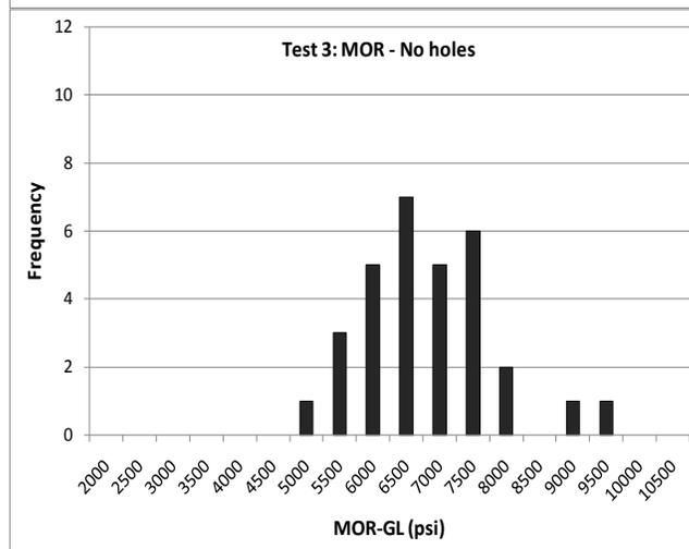
Figure III-4. MOR-GL distribution for Douglas-fir poles tested with the through-boring holes parallel or perpendicular to the loading direction, radial drilling or no holes in Test # 3.
