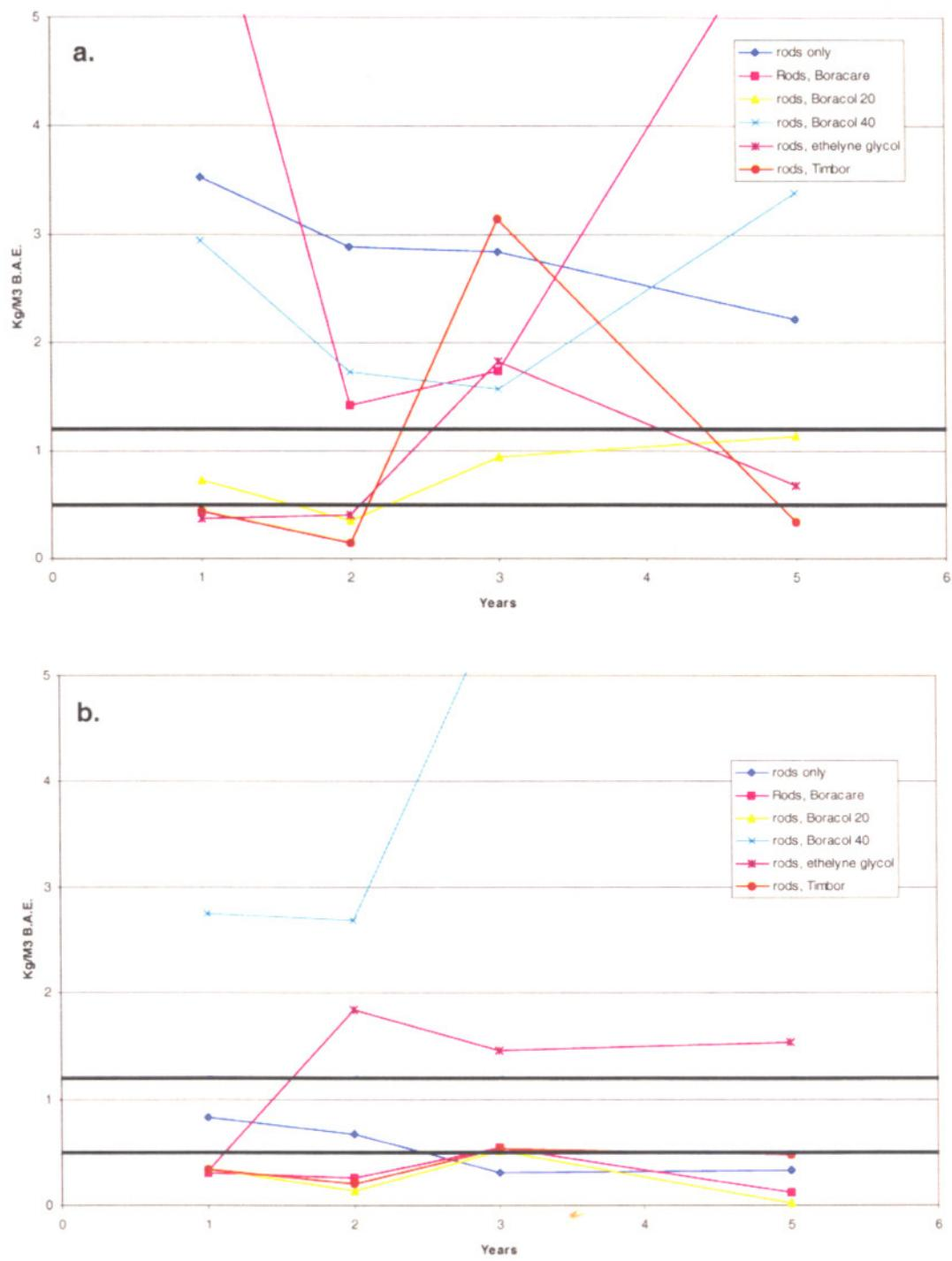
Figure 1-10. Boron levels in the outer (a), middle (b), and inner (c) zones of increment cores removed 300 mm above groundline from Douglas-fir poles sections 1 to 5 years after treatment with fused boron rods with or without various diffusion enhancers.
