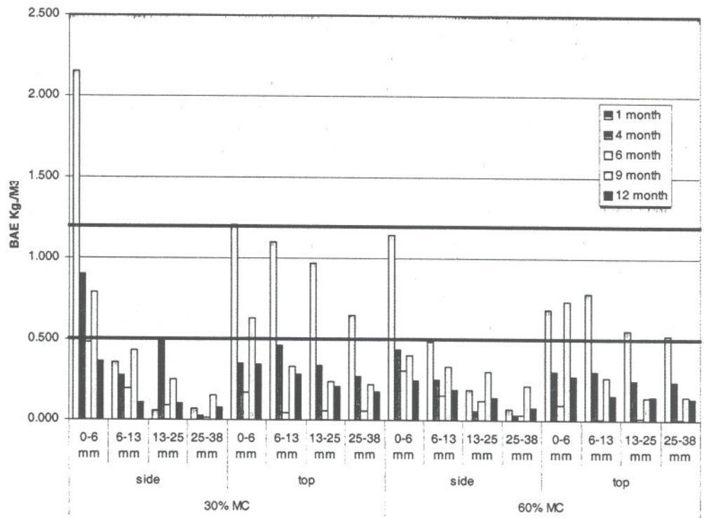
Figure IV-5. Boron levels at selected distances from the surface of Douglas-fir heartwood blocks at 30 or 60 % MC 1 to 12 months after application of a copper/boron/fluoride bandage.
