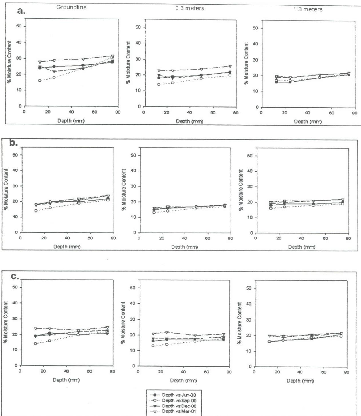
Figure III-3. Seasonal wood moisture contents in through-bored Douglas-fir poles treated with a) pentachlorophenol, b) creosote or c) copper naphthenate.
