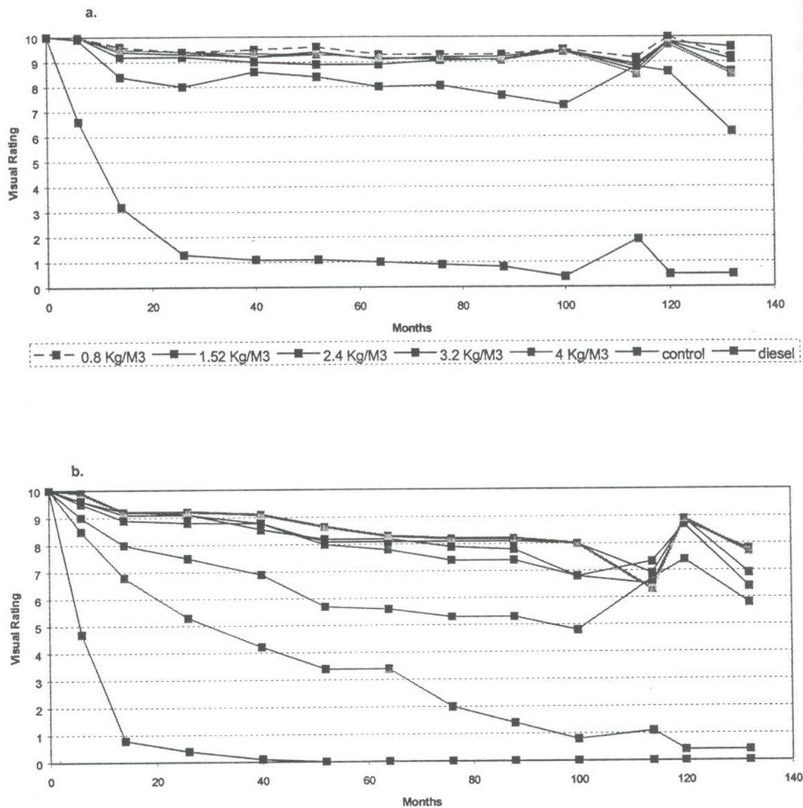
Figure IV-1. Conditions of a) freshly harvested and b) weathered western redcedar sapwood stakes treated with selected retentions of copper naphthenate and exposed for 132 months in a fungus cellar.
