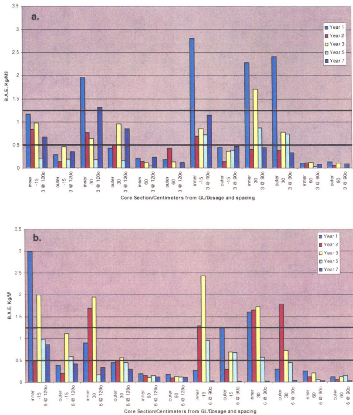
Figure 1-12. Residual levels of boron in Douglas-fir poles 1 to 7 years after treatment with a) three or b) six fluoride/boron rods distributed in holes spaced 90 or 120 degrees around the pole.
