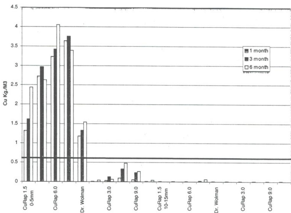
Figure IV-1. Copper levels at selected depths in Douglas-fir sapwood blocks 1, 3, and 6 months after application of either a copper/boron/fluoride bandage or varying thicknesses of a copper/boron paste.
