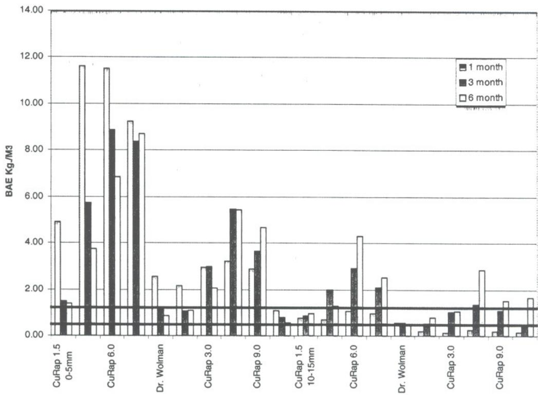
Figure IV-2. Boron levels at selected depths in Douglas-fir sapwood blocks 1, 3, and 6 months after application of either a copper/boron/fluoride bandage or varying thicknesses of a copper/boron paste.
