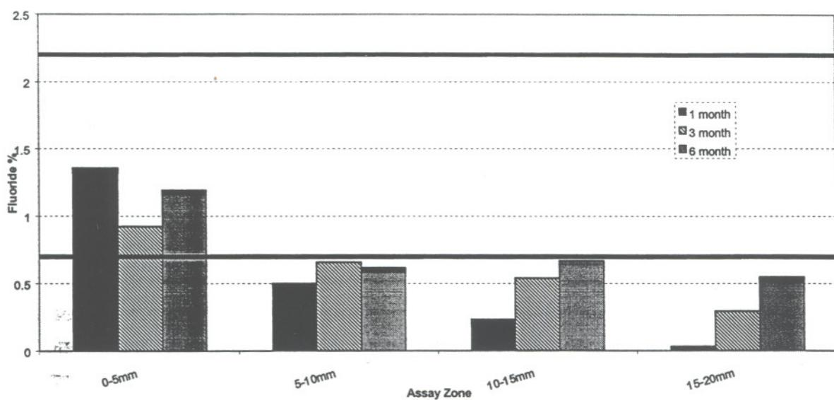
Figure IV-3. Fluoride levels at selected depths in Douglas-fir sapwood blocks 1, 3, and 6 months after application of a copper/boron/fluoride bandage.
