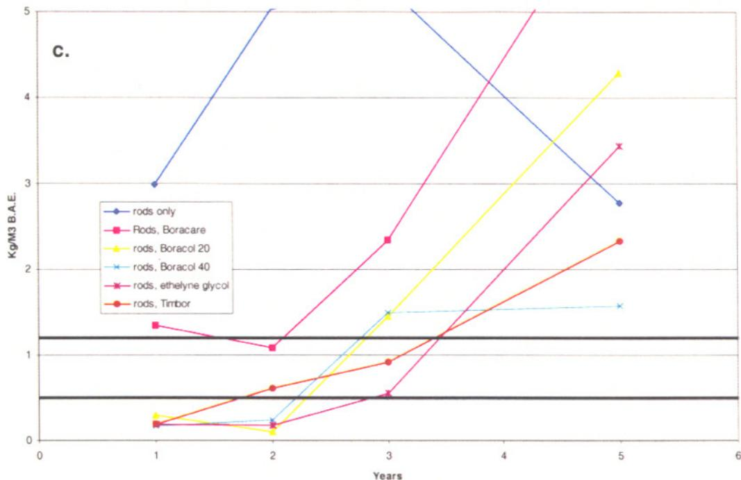
Figure 1-10 cont. Boron levels in the outer (a), middle (b), and inner (c) zones of increment cores removed 300 mm above groundline from Douglas-fir poles sections 1 to 5 years after treatment with fused boron rods with or without various diffusion enhancers.
