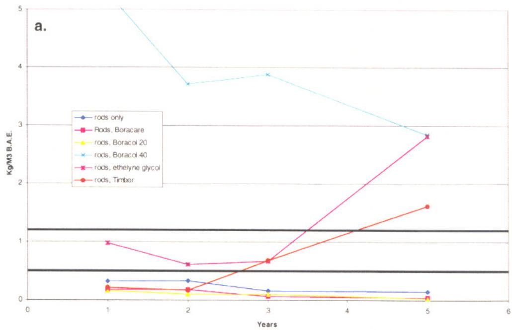
Figure 1-9. Boron levels in the outer (a), middle (b), and inner (c) zones of increment cores removed 150 mm above groundline from Douglas-fir poles sections 1 to 5 years after treatment with fused boron rods with or without various diffusion enhancers
