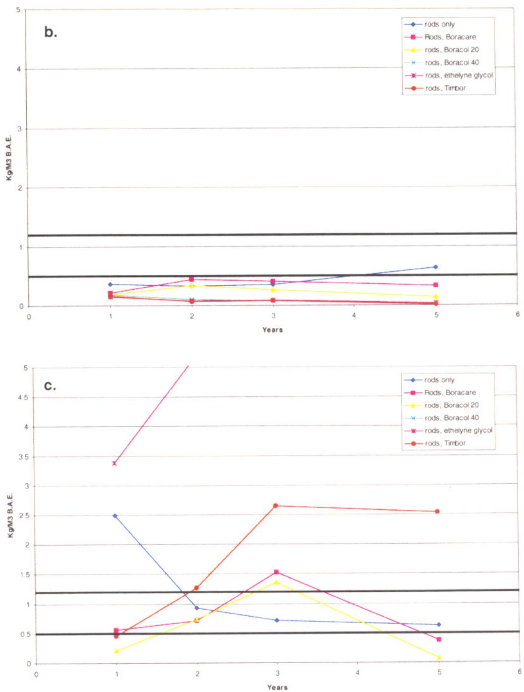
Figure 1-9. Boron levels in the outer (a), middle (b), and inner (c) zones of increment cores removed 150 mm above groundline from Douglas-fir poles sections 1 to 5 years after treatment with fused boron rods with or without various diffusion enhancers.
