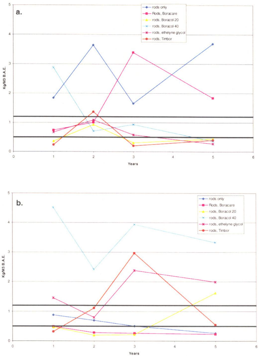
Figure 1-8. Boron levels in the outer (a), middle (b), and inner (c) zones of increment cores removed at groundline from Douglas-fir poles sections 1 to 5 years after treatment with fused boron rods with or without various diffusion enhancers.
