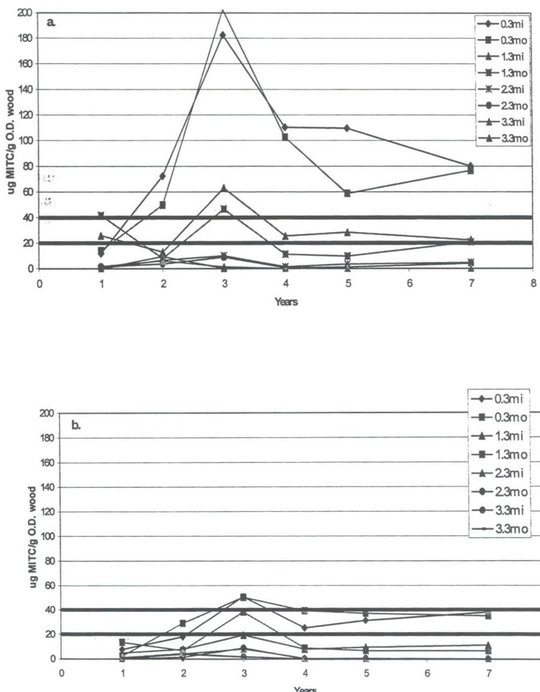
Figure I-2. MITC levels at selected distances above the groundline in Douglas-fir transmission poles 1 to 7 years after treatment with 200 g of basamid a) with or b) without copper sulfate
