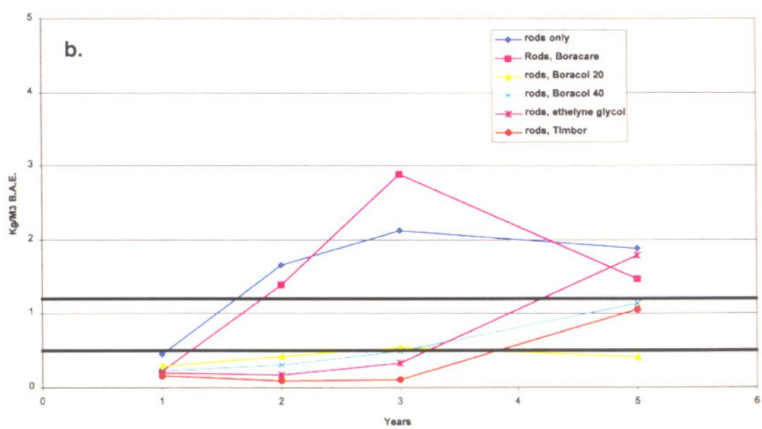
Figure 1-7. Boron levels in the outer (a), middle (b), and inner (c) zones of increment cores removed 300 mm below groundline from Douglas-fir poles sections 1 to 5 years after treatment with fused boron rods with or without various diffusion enhancers.
