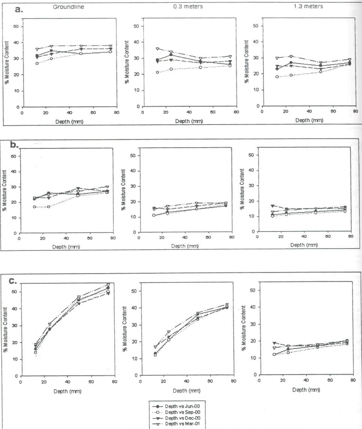
Figure 111-4. Seasonal wood moisture contents in a) through-bored and densely incised pentachlorophenol treated poles, b) western red cedar poles that were full length treated with pentachlorophenol or c) western red cedar poles that were butt-treated with creosote.
