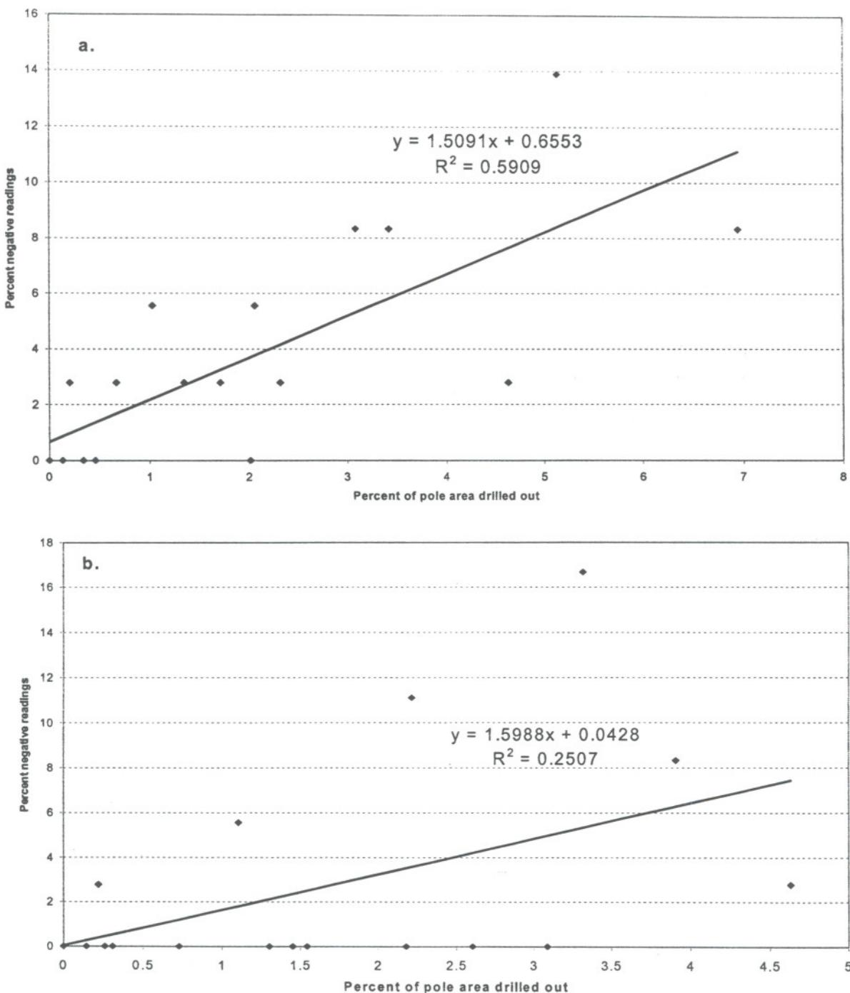
Figure III-19. Frequency of negative readings from the Purl inspection device on Douglas-fir pole sections with increasing amounts of wood removal a) to one side of the pole or b) from the center of the pole.
