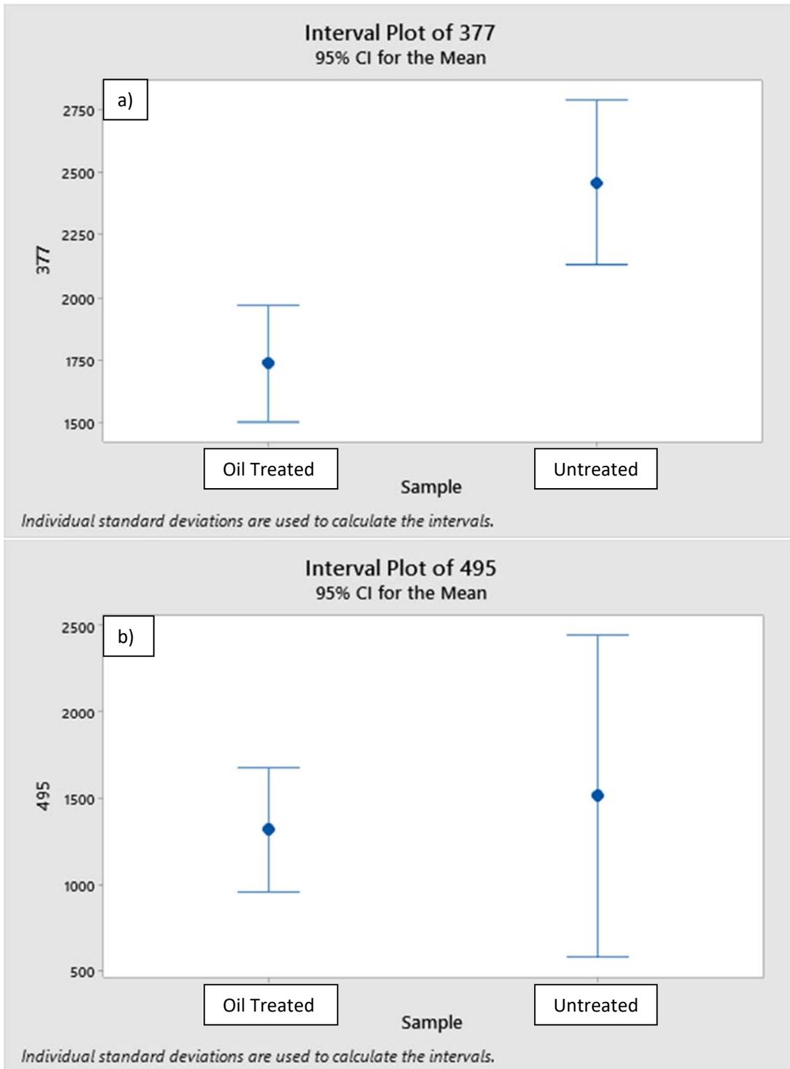
Figure I-13. Boron concentration variation on the receiving end of diffusion tests to highlight seal leakage. Panel a) significantly decreased boron diffusion across oil-borne preservative-treated shells. Panel b) no difference in boron concentration after seal leaks.
