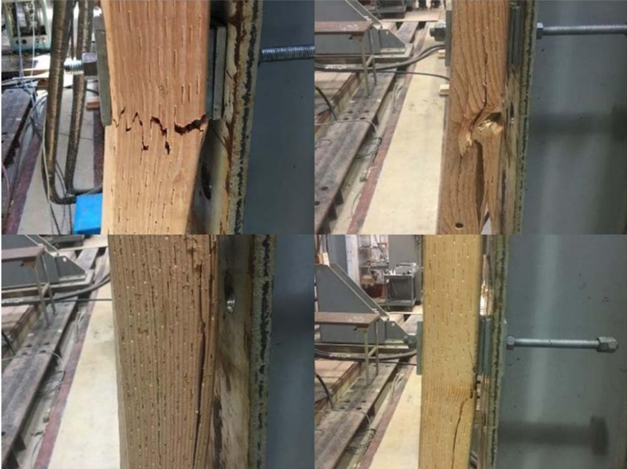
*Figure III-22a. Examples of various failures of Douglas-fir crossarms tested to failure in bending.*
