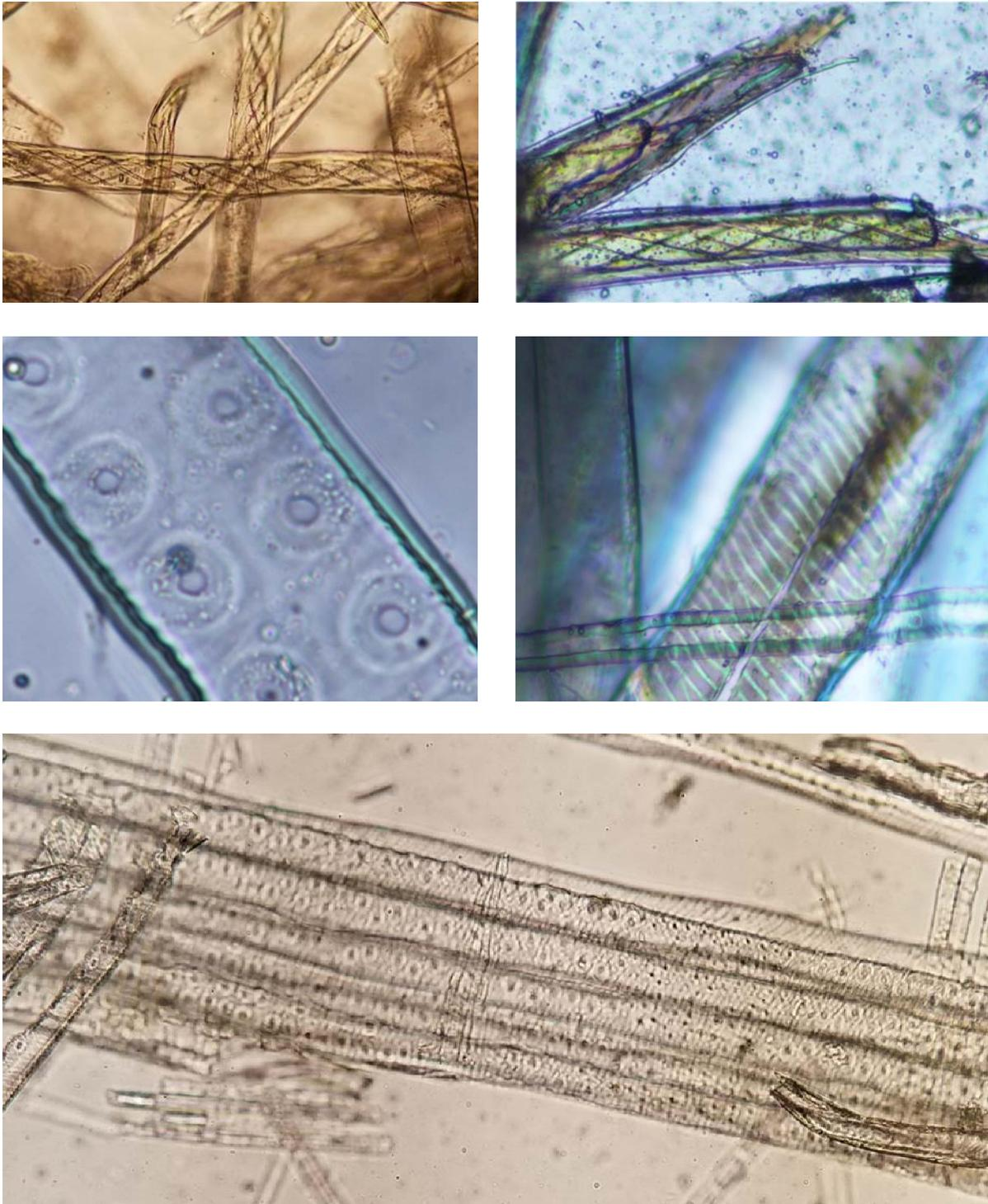
*Figure V-6. Examples of Douglas-fir tracheids removed from the outer surfaces of poles showing bordered pits and the spiral thickenings typical of this species (bottom) and diamond-shaped soft-rot cavities (top row).*
