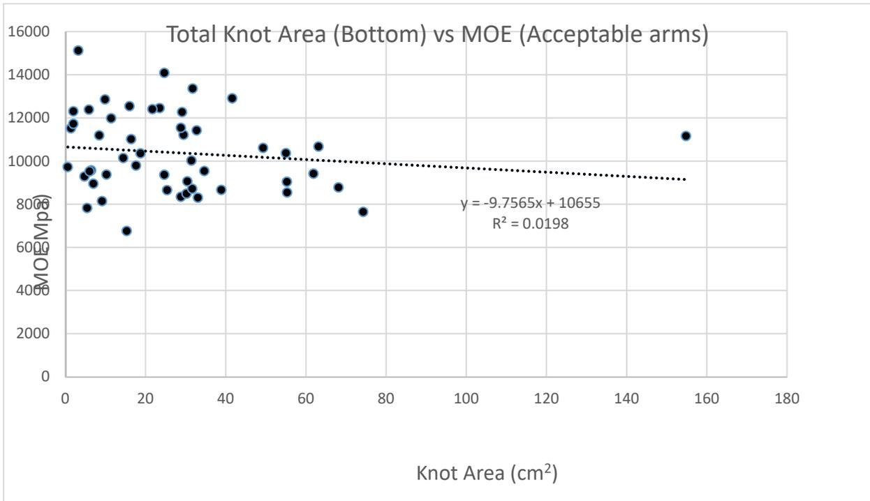
Figure III-27. Relationship between total knot area and MOE for accepted and rejected Douglas-fir crossarms.
