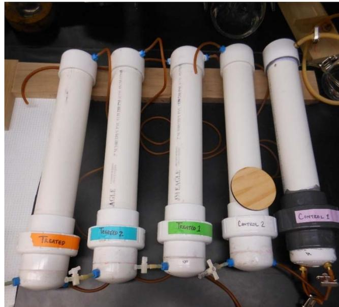
Figure I-10. Photograph of five of the diffusion apparatuses used to assess boron movement through non-treated or diesel oil-treated Douglas-fir lumber. A 25 mm diameter wood sample is resting on the fourth chamber to provide a measure of scale.
