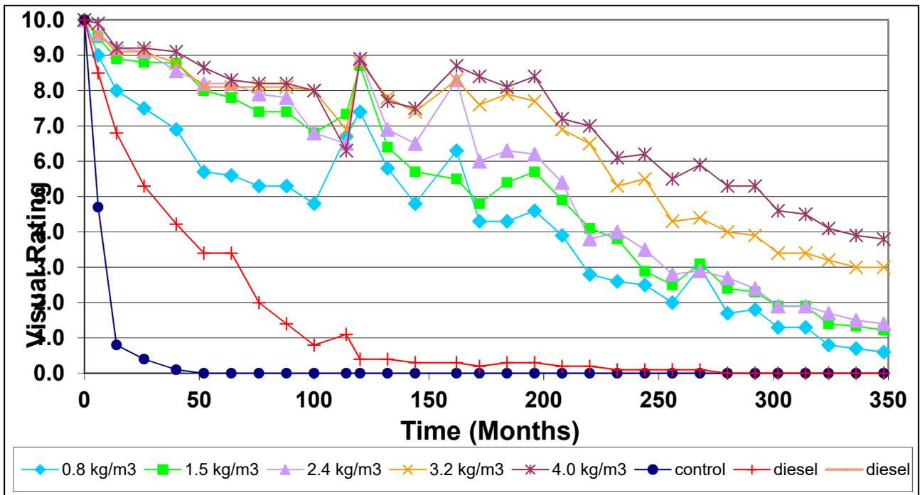
Figure V-2. Condition of weathered western redcedar sapwood stakes treated with selected retentions of copper naphthenate in diesel oil and exposed in a soil bed for 348 months.
