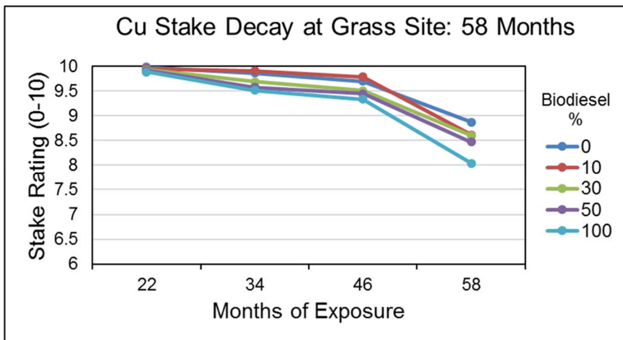
Figure III-15. Average ratings of Douglas-fir sapwood stakes at the grass site treated with copper naphthenate in mixtures of petroleum and bio-based diesel over 58 months of exposure in soil showing the relationship between increased biodiesel content and increased decay. These data combined all of the Cu retentions for each individual biodiesel level and are therefore not representative of industry treatment standards.
