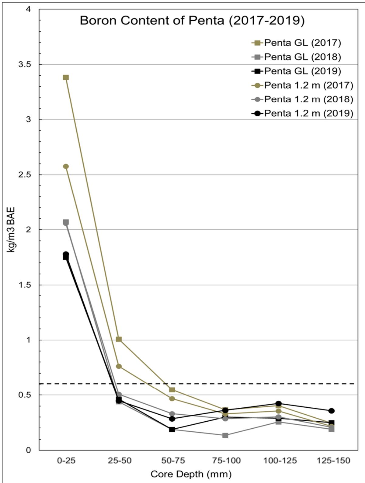
Figure II-9. Boron levels in Douglas-fir poles subjected to a boron pre-treatment followed by over-treatment with Pentachlorophenol after 3 years. Dotted black line indicates 0.6 kg/m<sup>3</sup> BAE, the threshold for decay prevention.
