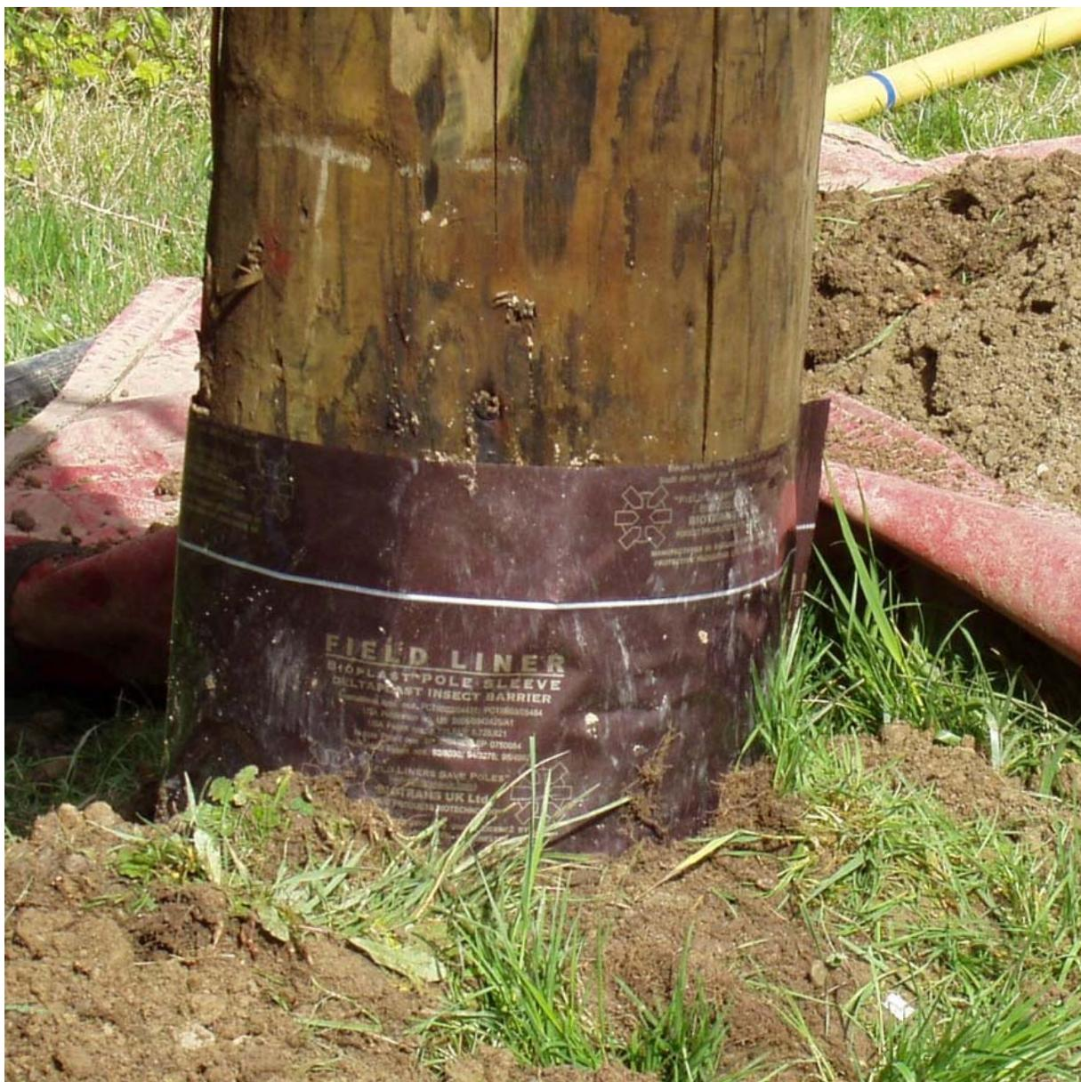
Figure IV-1. Example of a Biotrans liner at the OSU Peavy Arboretum test site.
