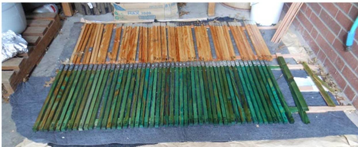
*Figure III-10. Stakes drying under cover after treatment with copper naphthenate (bottom) or penta (top).*
