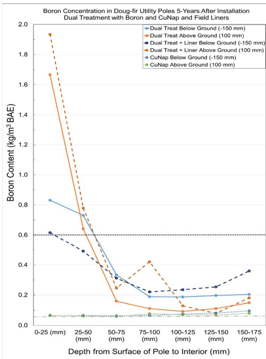
*Figure II-12. Average boron concentrations in Doug-fir utility poles 5-years after installation. Treatments and proximity of groundline are differentiated. Dotted black line indicates 0.6 kg/m<sup>3</sup> BAE, the threshold for fungal decay prevention. Dashed gray line indicates 0.07 kg/m<sup>3</sup> BAE, the average background boron levels identified in CuNap-treated poles.*
