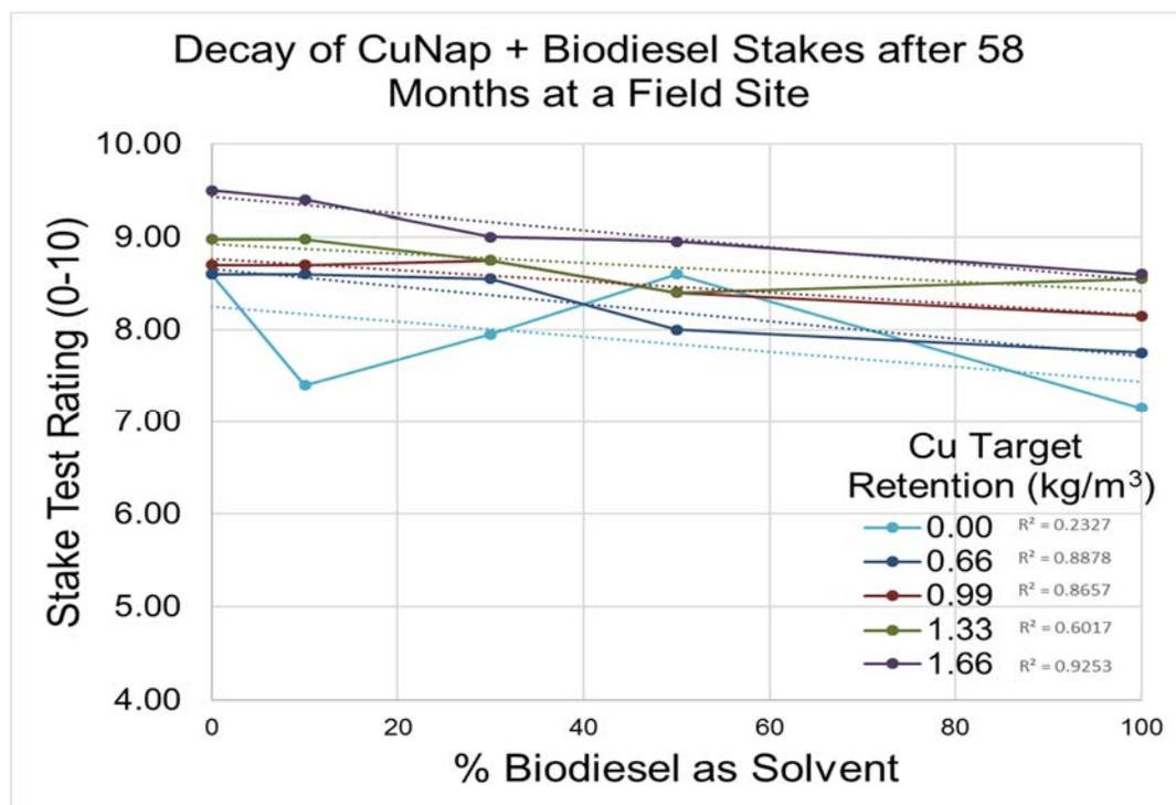
Figure III-12. Average ratings of Douglas-fir sapwood stakes at the field site treated with copper naphthenate in mixtures of petroleum and bio-based diesel after 58 months of exposure in soil.
