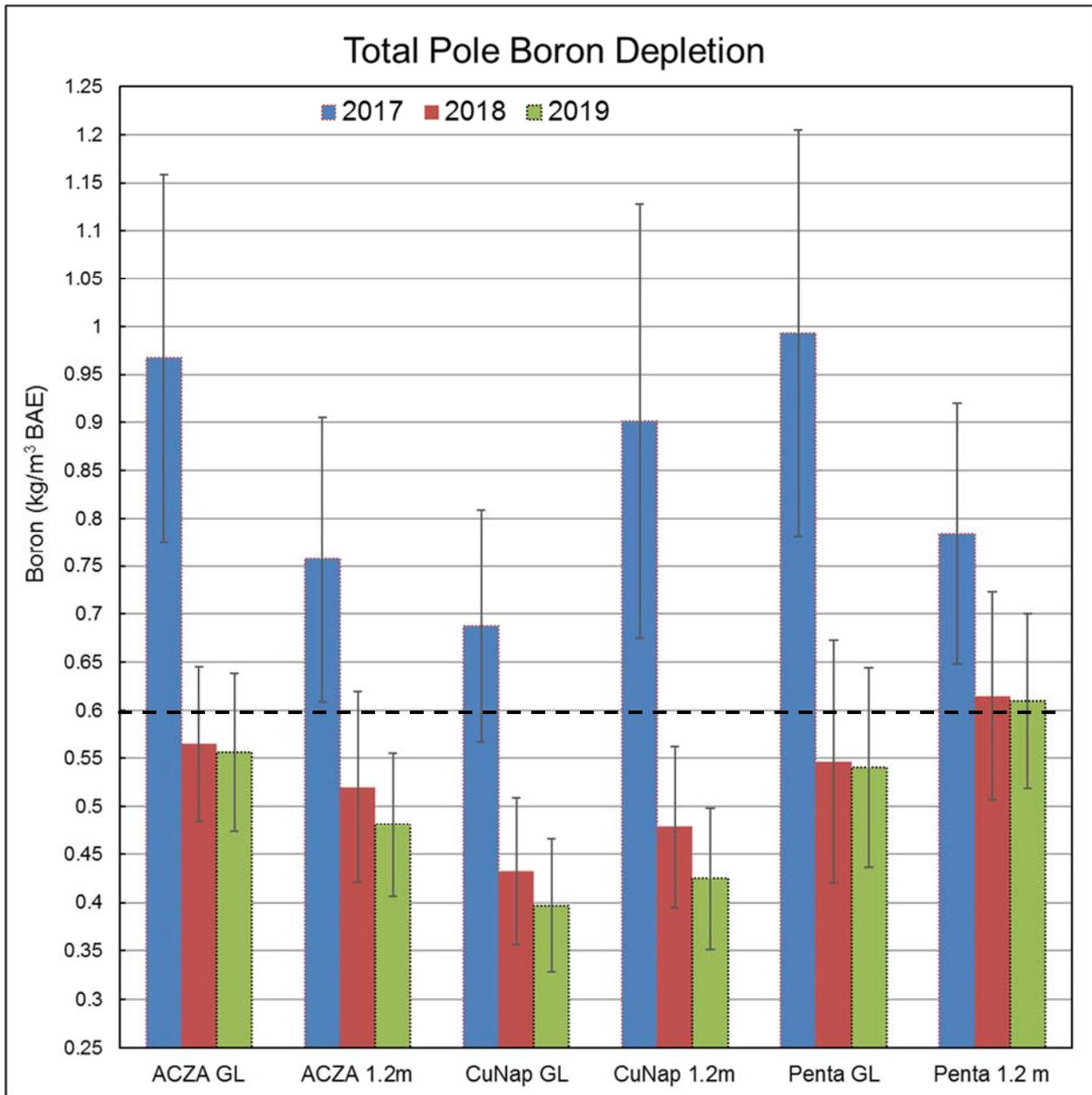
Figure II-11. Average of total pole boron content of Douglas-fir poles subjected to either a boron pre-treatment followed by over-treatment with copper naphthenate or pentachlorophenol, or an ACZA/boron pressure treatment after 3 years. Dotted black line indicates 0.6 kg/m<sup>3</sup> BAE, the threshold for decay prevention. Initial average pole boron concentrations after treatment are unknown. Values for 2017 represent 1-year exposed in the field. Bars represent standard error.
