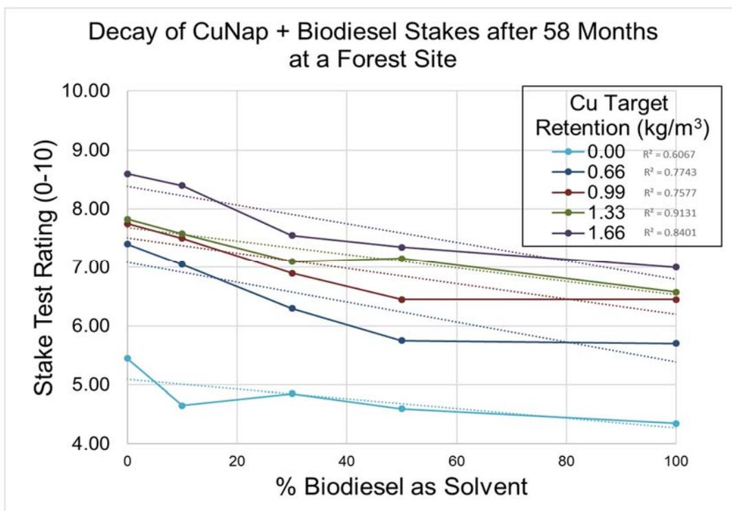
Figure III-11. Average ratings of Douglas-fir sapwood stakes at the forest site treated with copper naphthenate in mixtures of petroleum and bio-based diesel after 58 months of exposure in soil showing the relationship between increased biodiesel content and increased decay.
