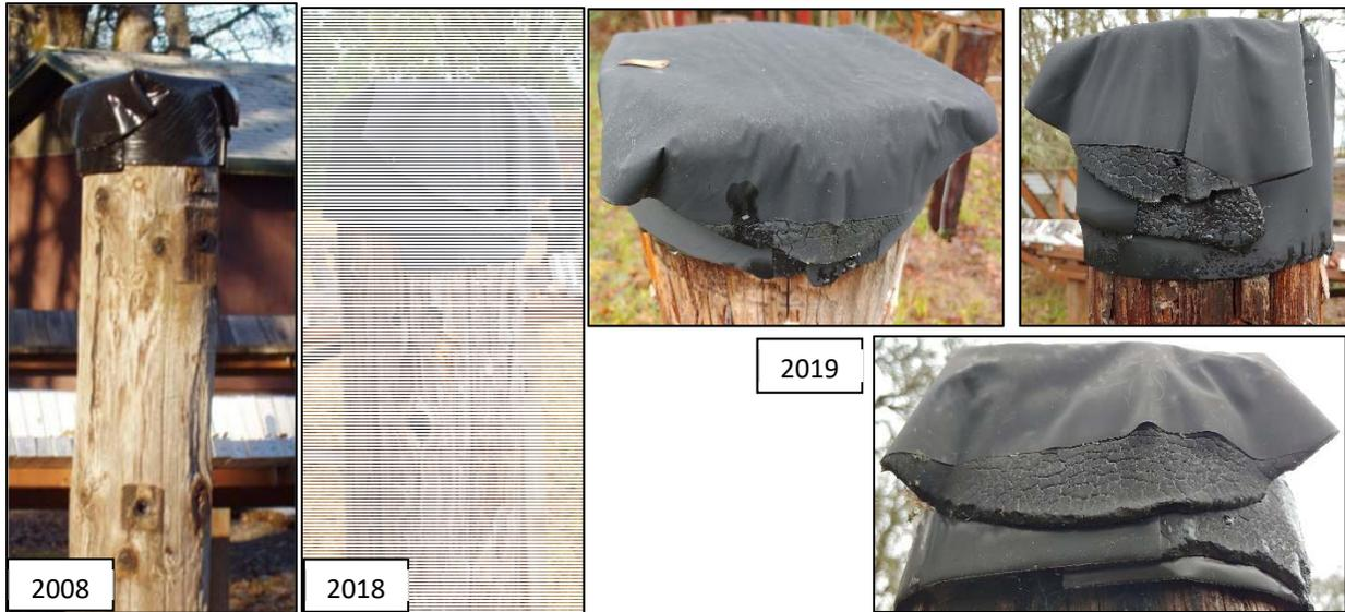
Figure III-1. Example of the condition of water-shedding caps at the start of exposure and after 142 months of exposure in Corvallis, OR.
