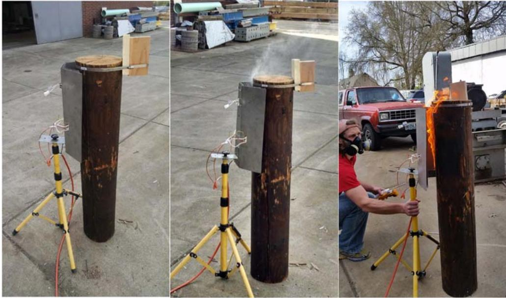
Figure III-7. Example of the fire test apparatus being applied to a penta-treated Douglas-fir pole showing initial heating, the beginning of combustion with smoke and finally, the pole on fire.
