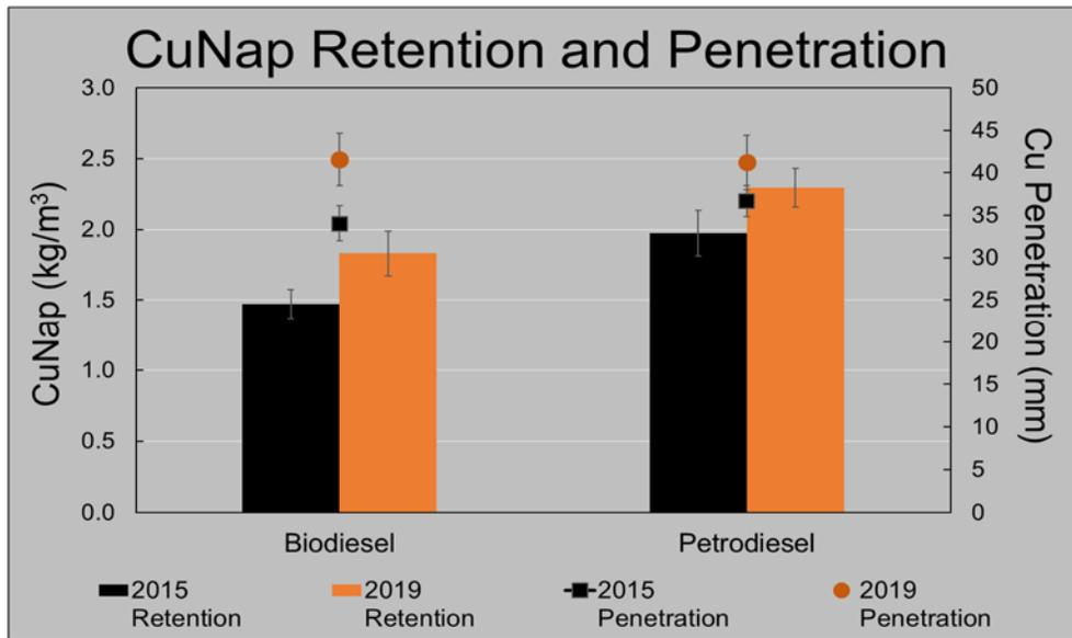
Figure V-4: Copper retention levels and copper penetration levels measured in cores from 65 copper naphthenate-treated utility poles using biodiesel or petrodiesel as a carrier. Data presented are from the 2015 and 2019 sampling. Error bars represent standard error.
