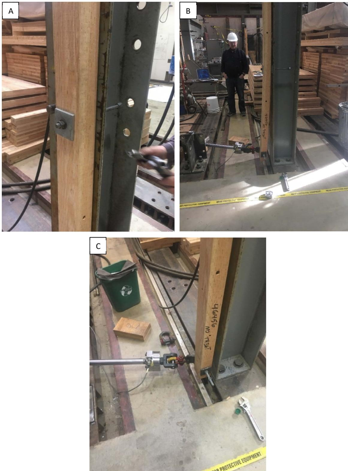
Figure III-21. Photos of the test set up used to assess crossarm properties showing: A) an arm bolted to the steel bracket, B) an arm showing deflection under load as it is tested, and C) the hydraulic rod used to pull the arm.
