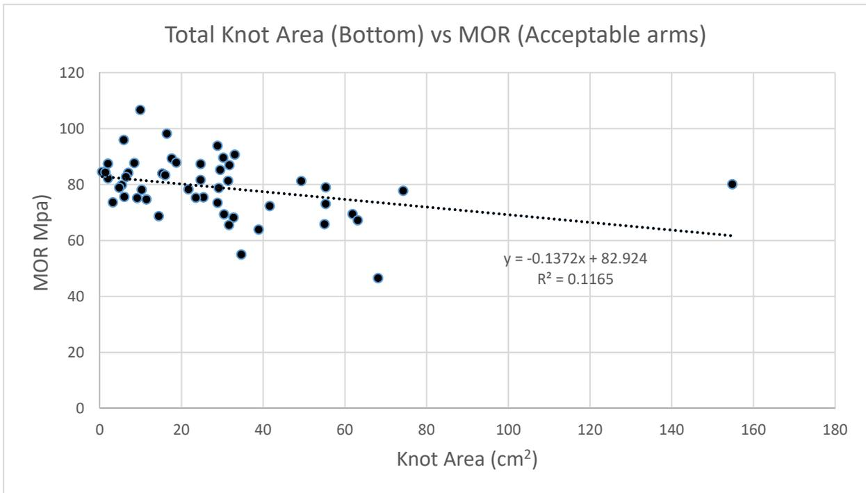
Figure III-26. Relationship between total knot area on the bottom (tension) face and MOR for accepted and rejected Douglas-fir crossarms.
