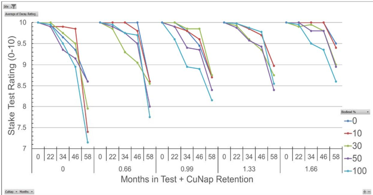
Figure III-14. Average ratings of Douglas-fir sapwood stakes at the grass site treated with copper naphthenate in mixtures of petroleum and bio-based diesel after 22, 34, 46, and 58 months of exposure in soil.
