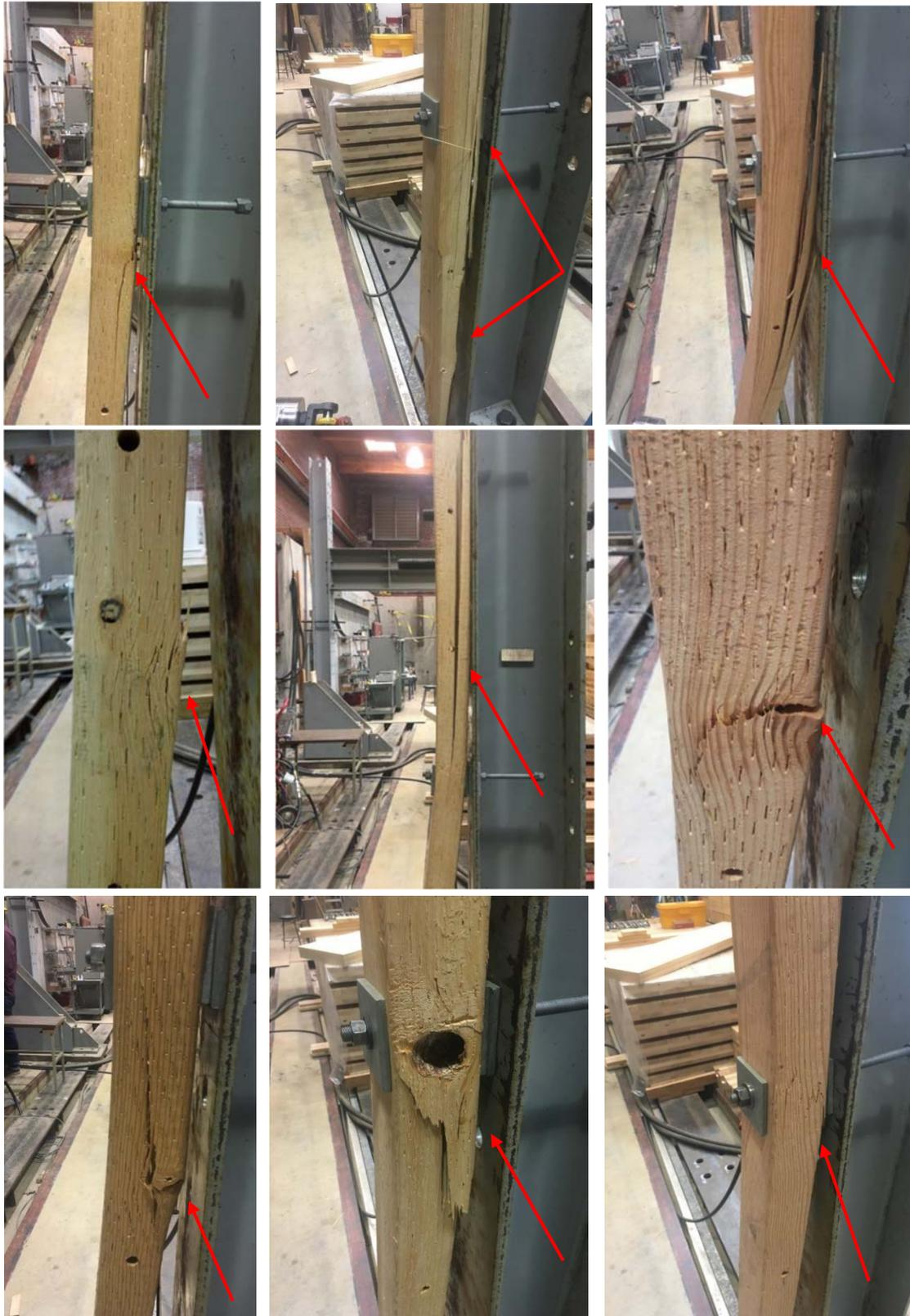
Figure III-22b. Examples of crossarm failures (red arrows) following full-scale flexural testing.
