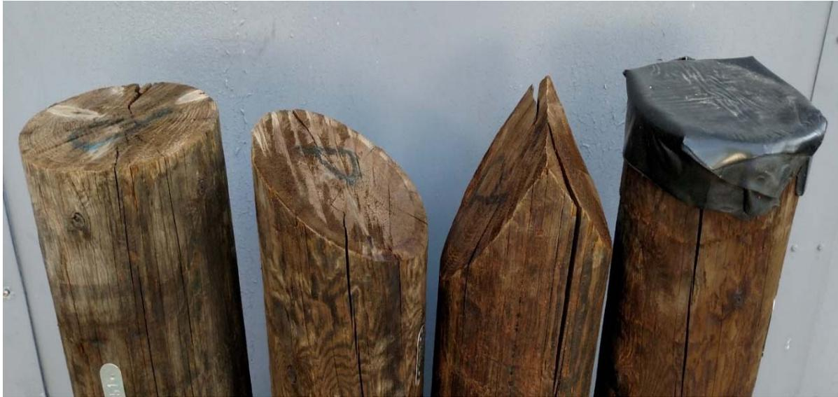
Figure III-4. Examples of the different pole top roofing patterns assessed for their ability to resist moisture ingress.
