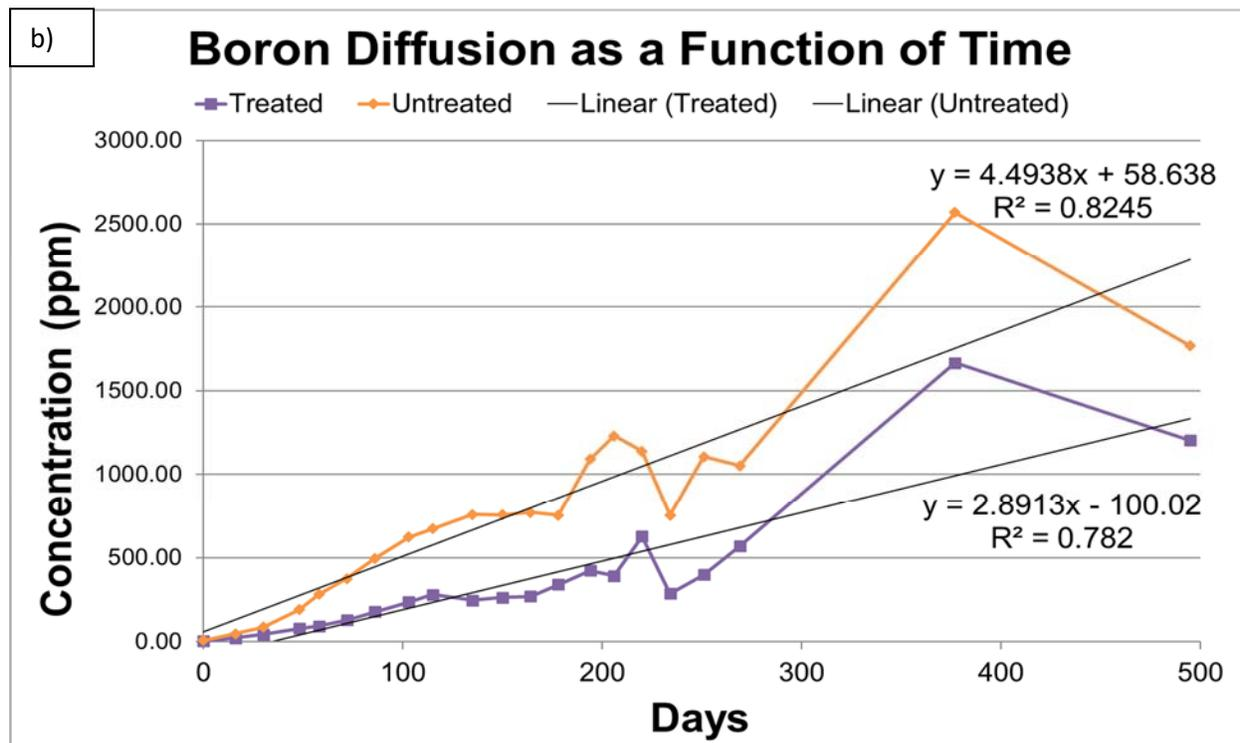
Figure I-12. Boron concentrations over time on the receiving end of diffusion tests using radially oriented Douglas-fir sapwood with biodiesel (treated) or without biodiesel (untreated). Panel a) rate of boron diffusion prior to suspect seal leak between 377 and 495 days. Panel b) rate of boron diffusion after suspect seal leak between 377 and 495 days.
