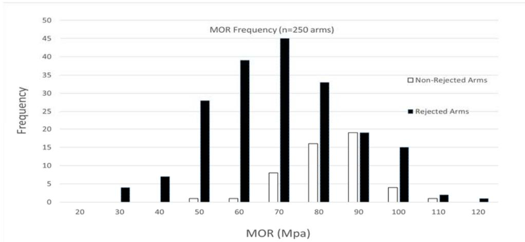
Figure III-23. Distribution of MOR values for acceptable and rejected Douglas-fir crossarms tested to failure where the assumed minimum ANSI value for MOR is 53.78 MPa.
