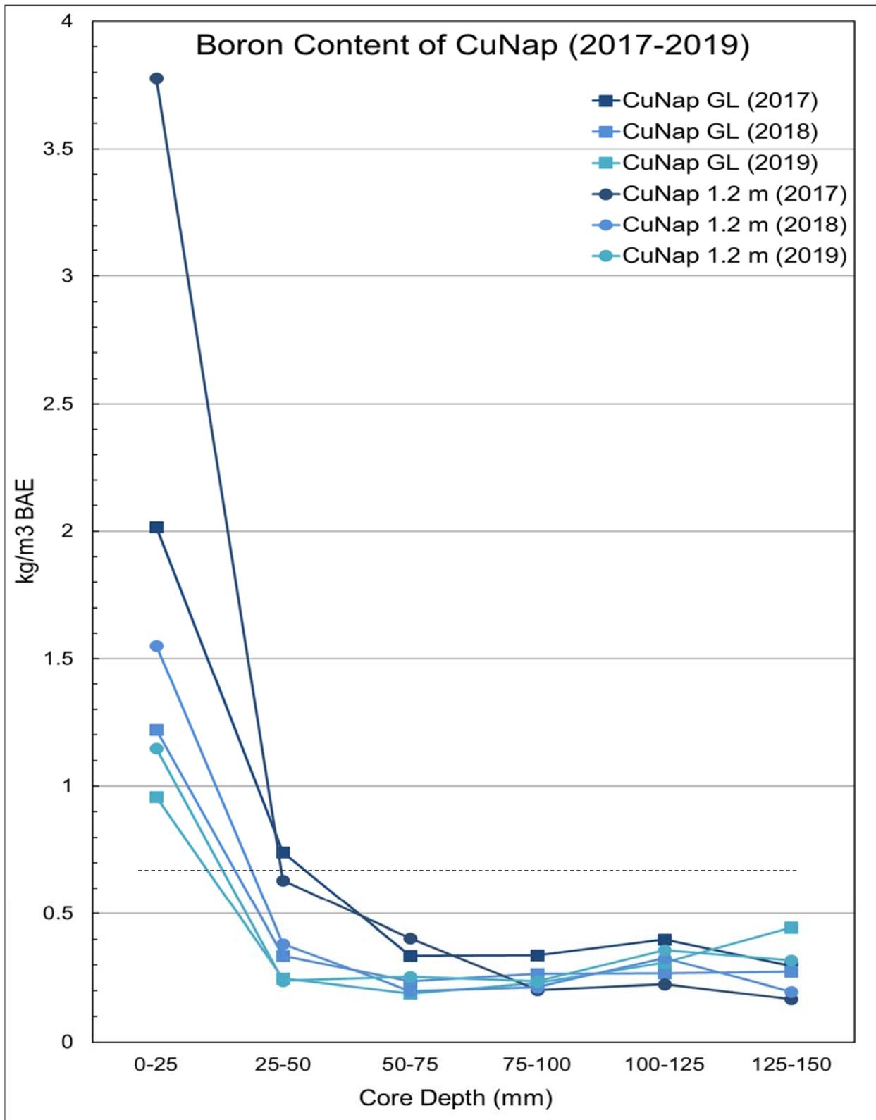
Figure II-8. Boron levels in Douglas-fir poles subjected to a boron pre-treatment followed by over-treatment with copper naphthenate after 3 years. Dotted black line indicates 0.6 kg/m<sup>3</sup> BAE, the threshold for decay prevention.
