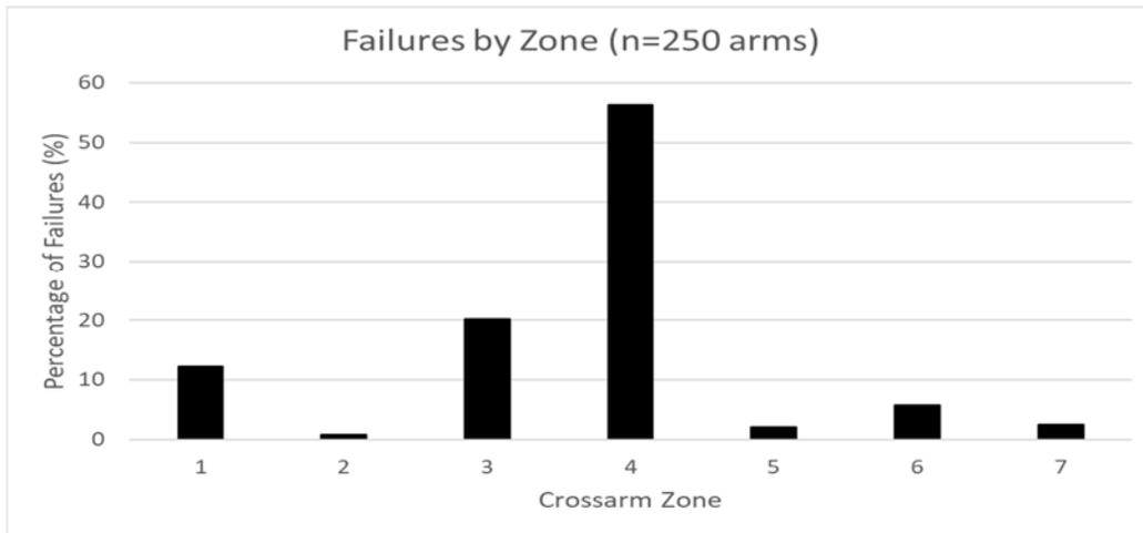
Figure III-24. Frequency of failure in the seven zones of the crossarms as shown in Figure III-20.
