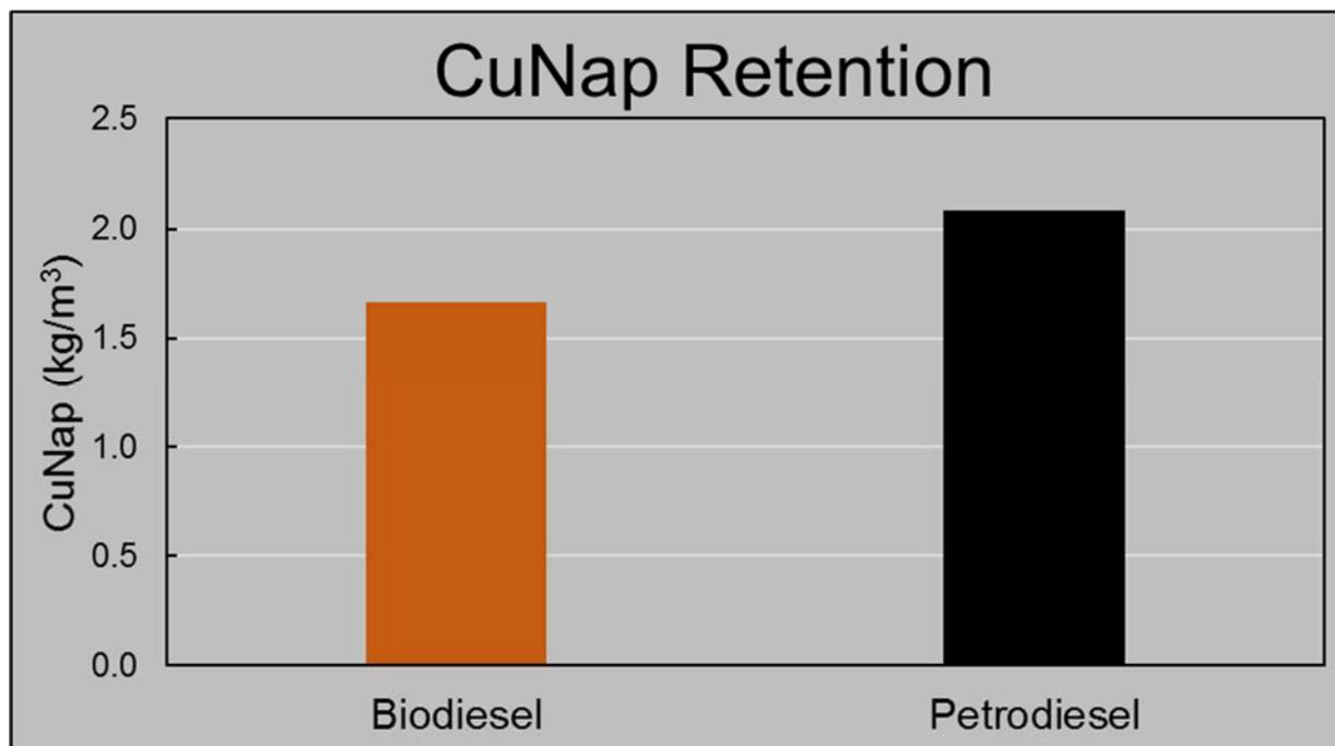
Figure V-8. Average retention levels of copper naphthenate in the outermost 6-25 mm of the poles. Retentions for all poles from each treatment type were averaged.
