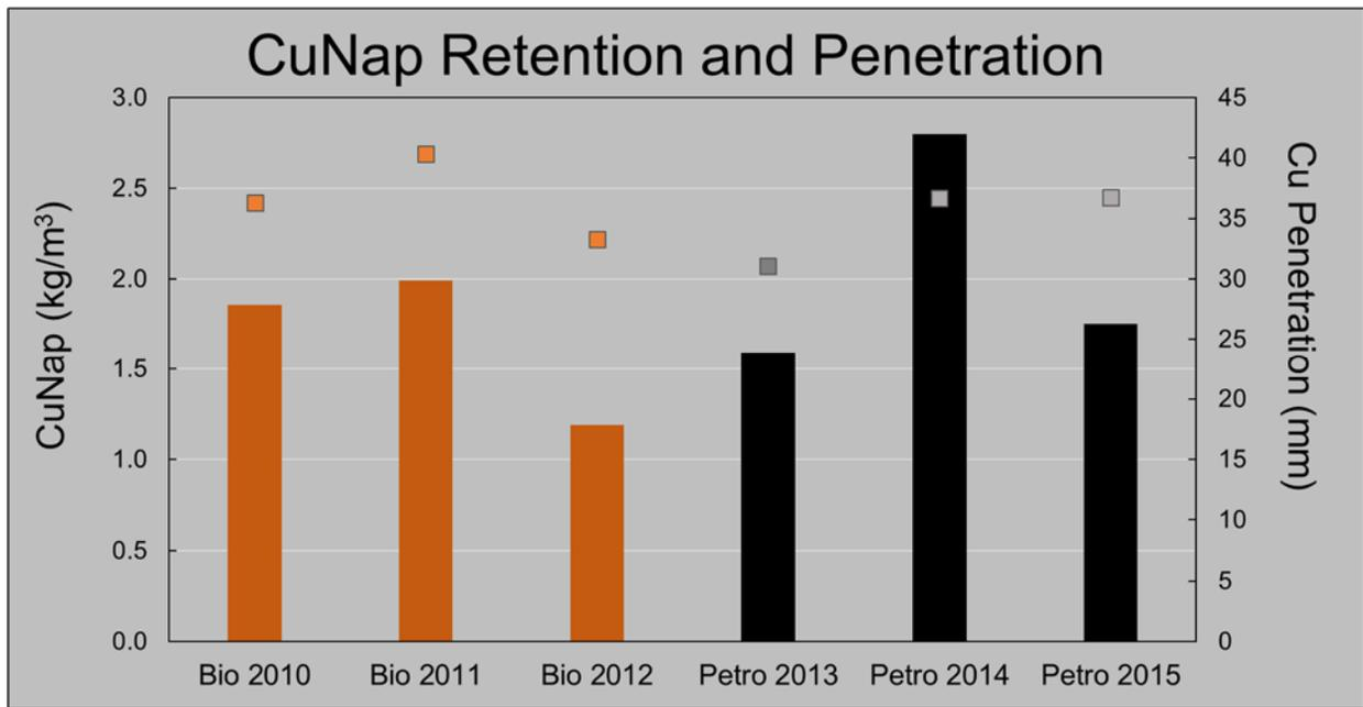
Figure V-9. Average retention levels and penetration depth of copper naphthenate in biodiesel and petrodiesel carrier-treated poles separated by the year they were installed.
