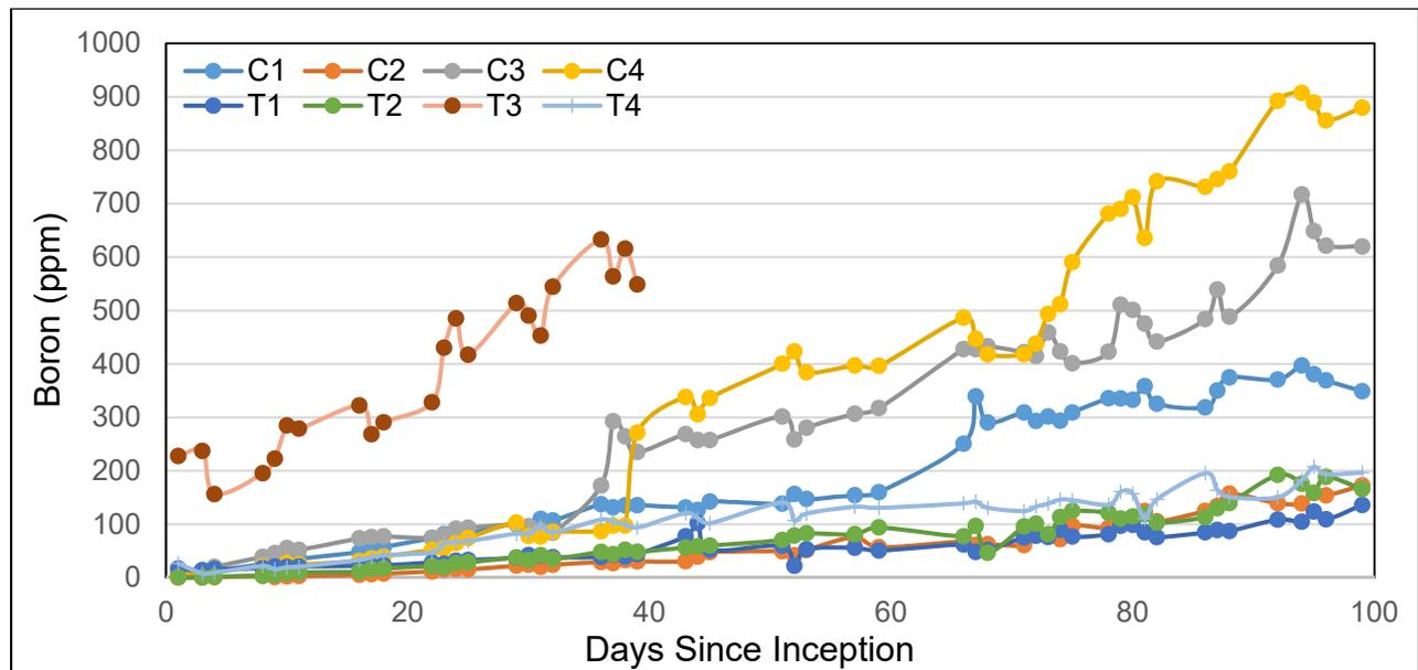
Figure I-11. Detail of boron concentrations early in the time-course on the receiving end of diffusion tests using radially oriented Douglas-fir sapwood with or without a biodiesel treatment, where C= no treatment and T= diesel treated samples. The T-3 sample developed a leak and was dropped from the test.
