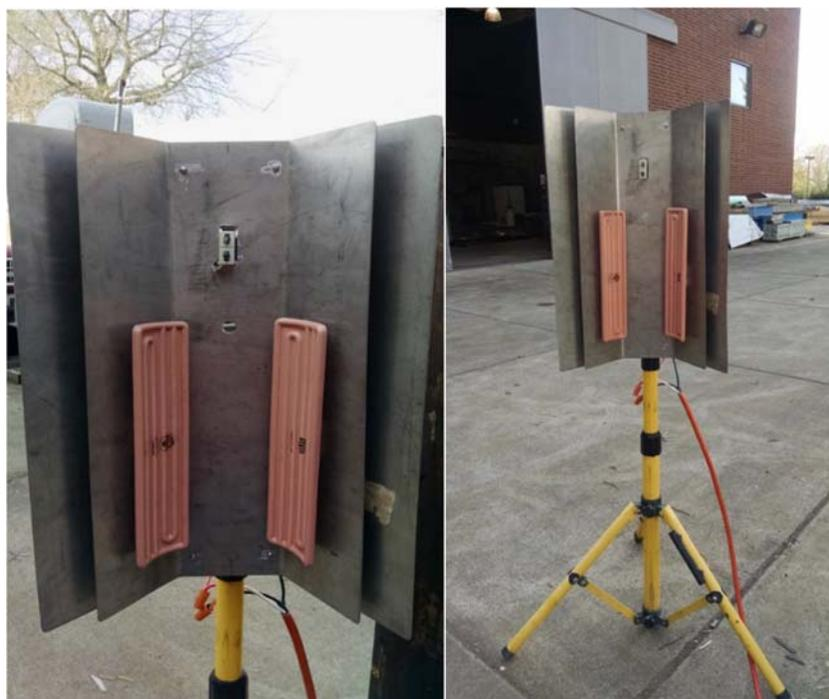
*Figure III-6. Example of the small-scale fire test apparatus showing the heating shield on a tripod and a close up of the heating elements.*
