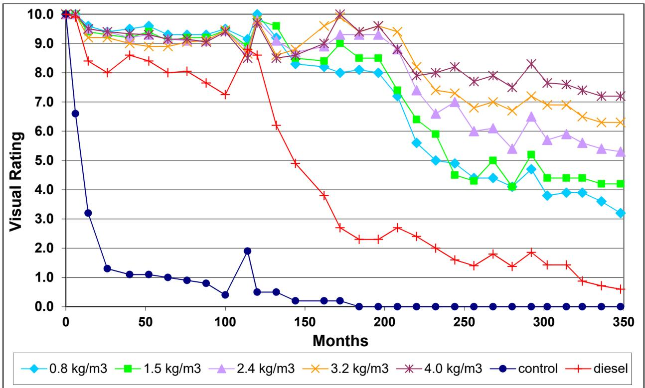
Figure V-1. Condition of freshly sawn western redcedar sapwood stakes treated with selected retentions of copper naphthenate in diesel oil and exposed in a soil bed for 348 months.
