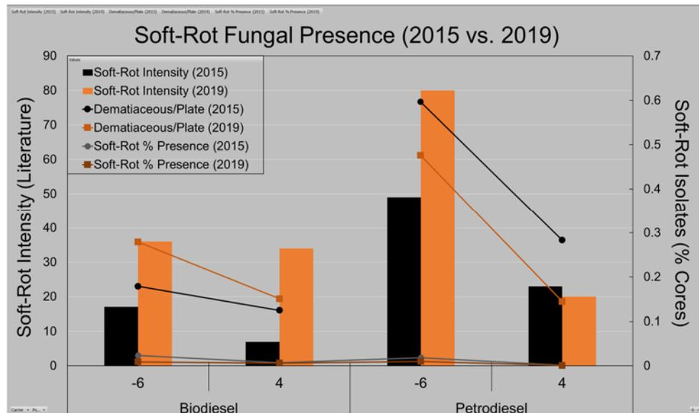
Figure V-5: Soft rot intensity and frequency of soft rot fungal isolations coming from the outer 2 mm of core taken from above and below ground areas of copper naphthenate treated utility poles using either a biodiesel or petrodiesel carrier. Data from the 2015 and 2019 samplings are presented.
