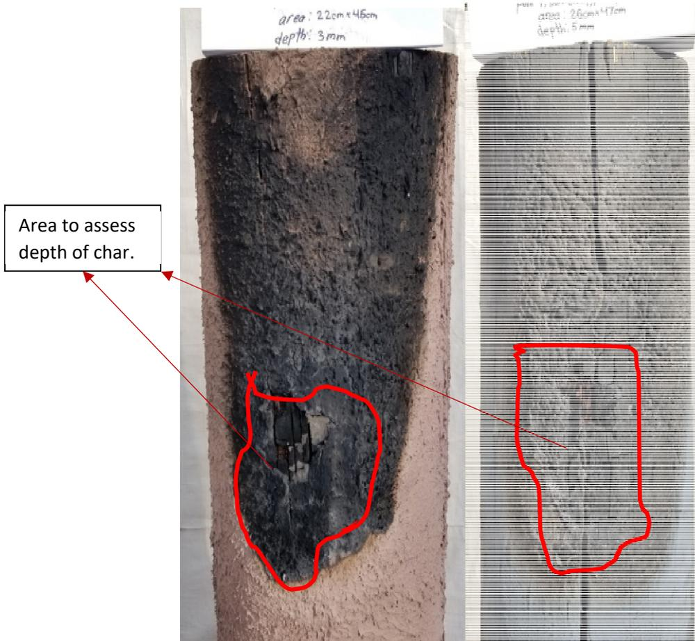
Figure III-8. Example of burned poles showing char, rough char area, and depth of char visualized by scraping surface char away.
