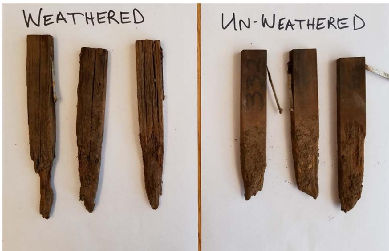
*Figure V-3. Examples of western redcedar stakes cut from weathered poles and freshly sawn lumber that have failed in test showing a tendency for wood to decay towards the lower end of the samples.*
