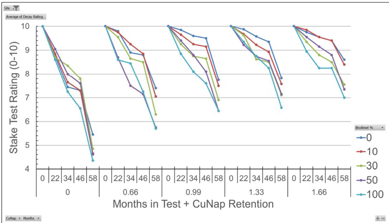
Figure III-13. Average ratings of Douglas-fir sapwood stakes at the forest site treated with copper naphthenate in mixtures of petroleum and bio-based diesel after 22, 34, 46, and 58 months of exposure in soil.
