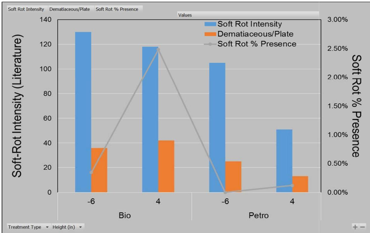
Figure V-10. Soft rot intensity and rates of isolation of soft-rot fungi from the outer 2 mm of increment cores taken 6 mm above ground and 4 mm below ground from poles treated with a biodiesel or petrodiesel carrier.
