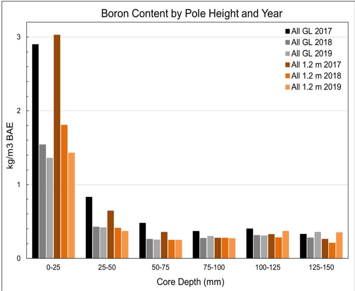
Figure II-10. Combined boron levels in Douglas-fir poles subjected to a boron pre-treatment followed by over-treatment with copper naphthenate or pentachlorophenol, or an ACZA/boron pressure treatment after 3 years. Dotted black line indicates 0.6 kg/m<sup>3</sup> BAE, the threshold for decay prevention.
