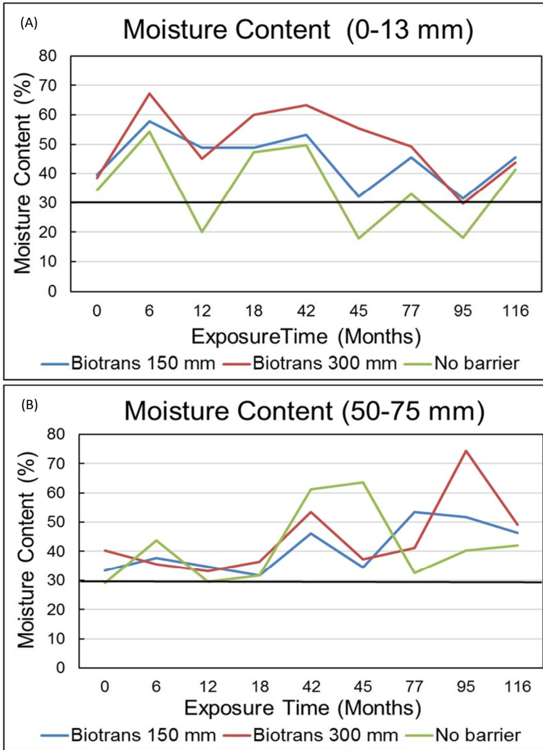
Figure IV-2. Moisture contents in the outer 0-13 mm (A) and inner 50-75 mm (B) zones of pentachlorophenol treated Douglas-fir poles with or without a Biotrans liner set so the liner top was 150 or 300 mm above groundline. The line at 30% represents the approximate fiber saturation point of wood.
