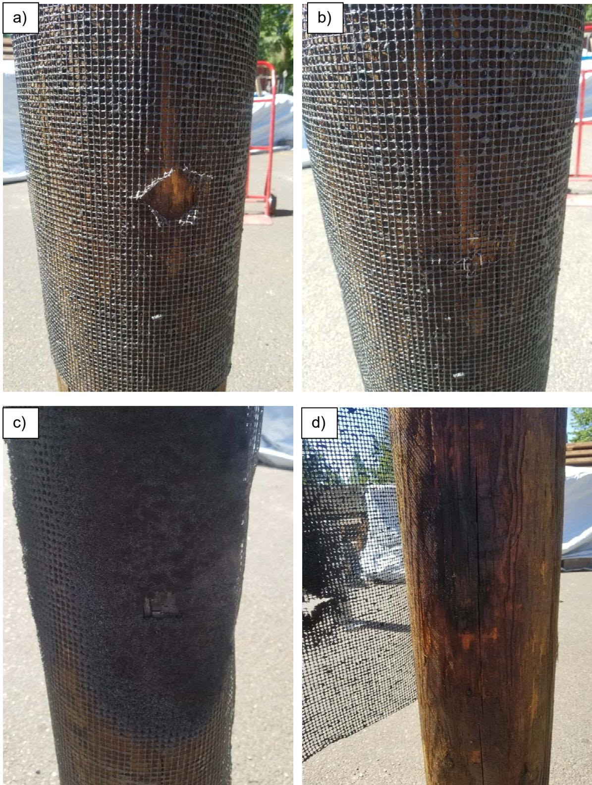
Figure III-9. Example of Genics Fire Mesh burned poles in several configurations. Photos a + b is the “x” configuration. Photo c is the square cutout configuration. Photo d is the pole surface following a burn with Genics Mesh in the “x” configuration.
