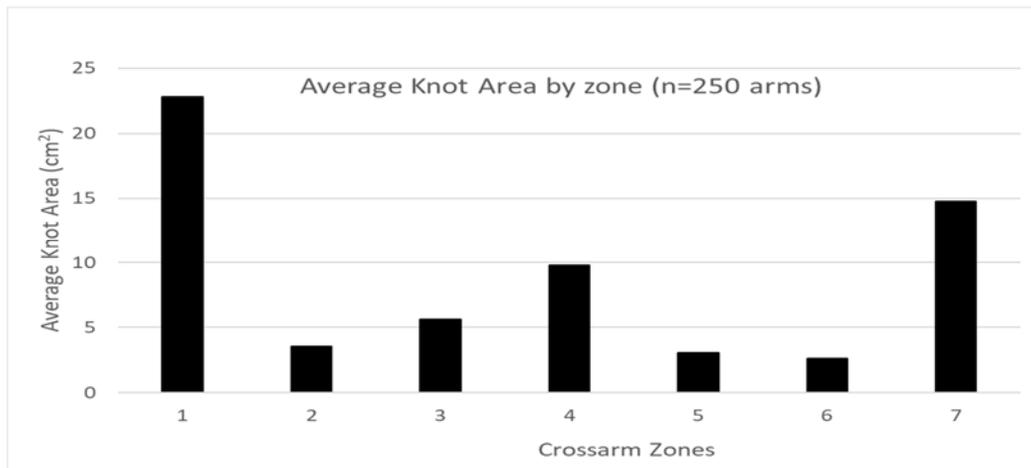
Figure III-25. Average knot area in zones of Douglas-fir cross arms that were accepted or rejected based upon ANSI 05.3 criteria.
