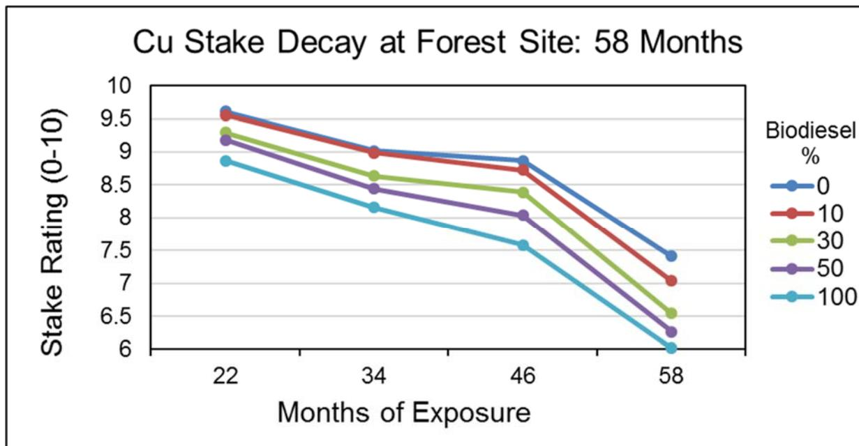
Figure III-16. Average ratings of Douglas-fir sapwood stakes at the forest site treated with copper naphthenate in mixtures of petroleum and bio-based diesel over 58 months of exposure in soil showing the relationship between increased biodiesel content and increased decay. These data combined all of the Cu retentions for each individual biodiesel level and are therefore not representative of industry treatment standards.
