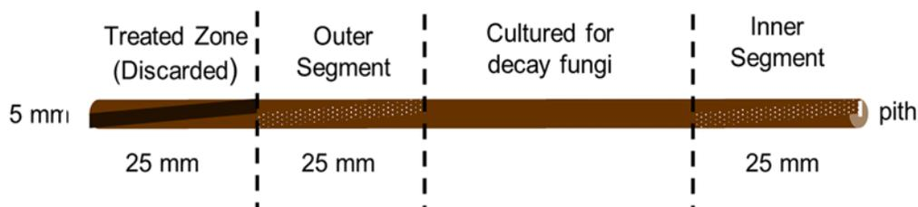
Figure I-1. Schematic of core processing for fumigant analysis and fungal culturing.
