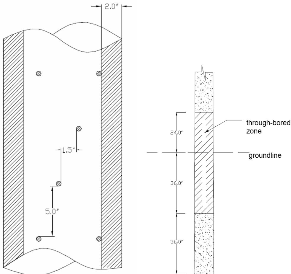
Figure III-1. Illustration of through-boring pattern showing a) hole spacing and b) through-boring zone on pole.
