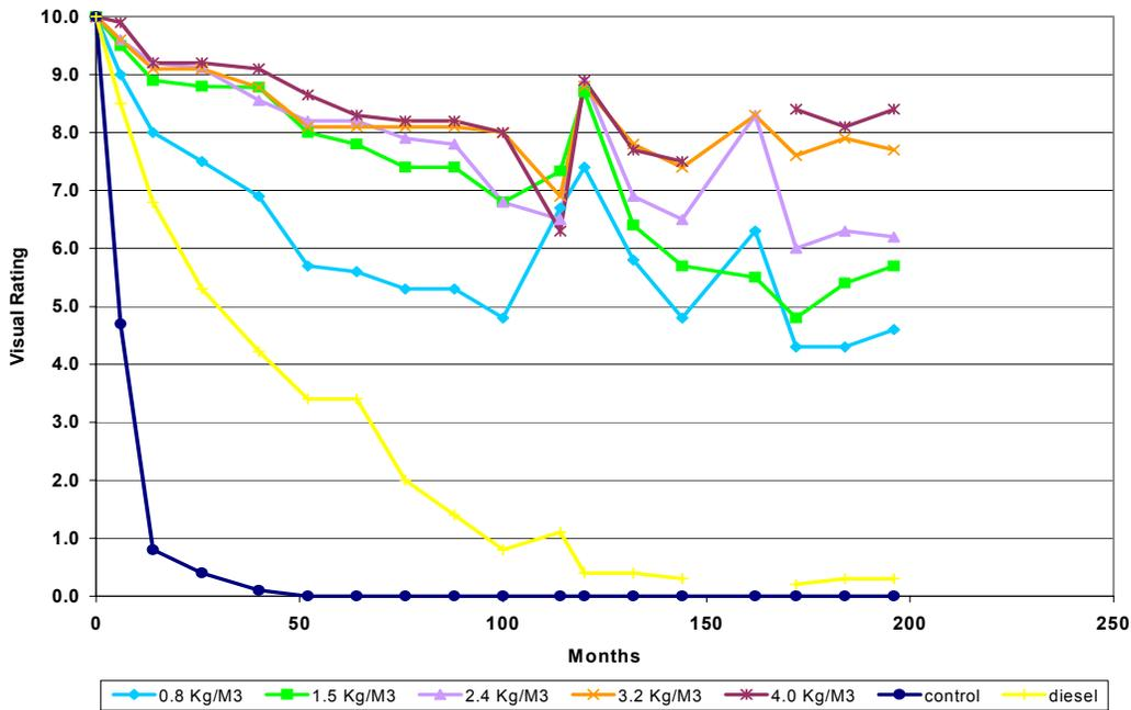
Figure V-2. Condition of weathered western redcedar sapwood stakes treated with selected retentions of copper naphthenate in diesel oil and exposed in a soil bed for 196 months.
