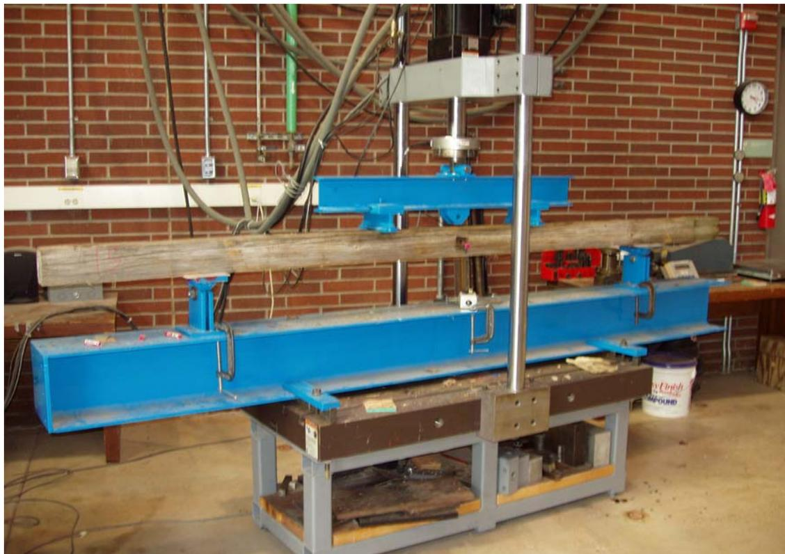
Figure III-16. Example of a cross arm in four point loading.
