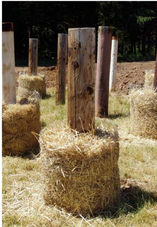
Figure III-28. Example of straw fuel in a wire basket around Douglas-fir poles with or without a fire retardant barrier.
