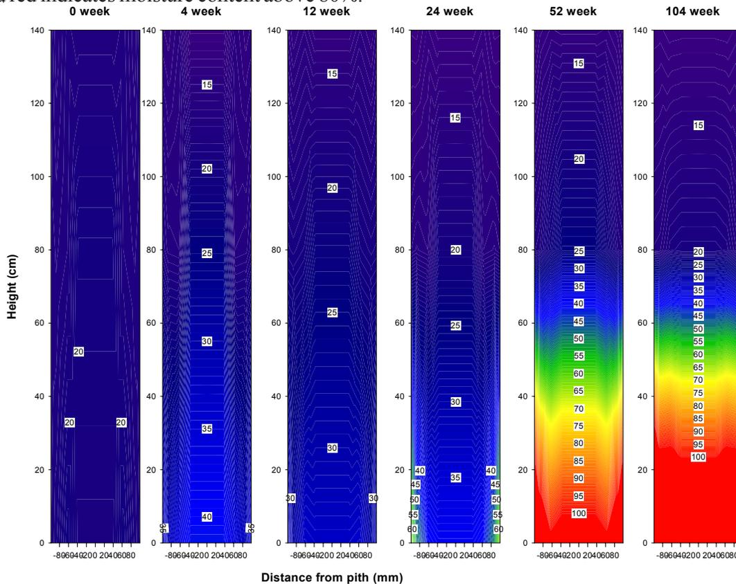
Figure III-10. Moisture contents of copper naphthenate treated western redcedar poles wrapped with a UPC liner from the butt to the groundline and immersed in moist soil for 0 to 104 weeks. Dark blue indicates moisture content below fiber saturation and red indicates moisture content above 80%.
