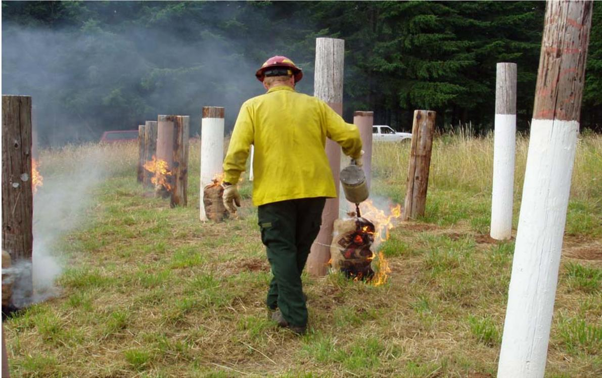
Figure III-27. Ignition of bagged straw with a drip torch at the Peavy Arboretum test burn site in 2005.
