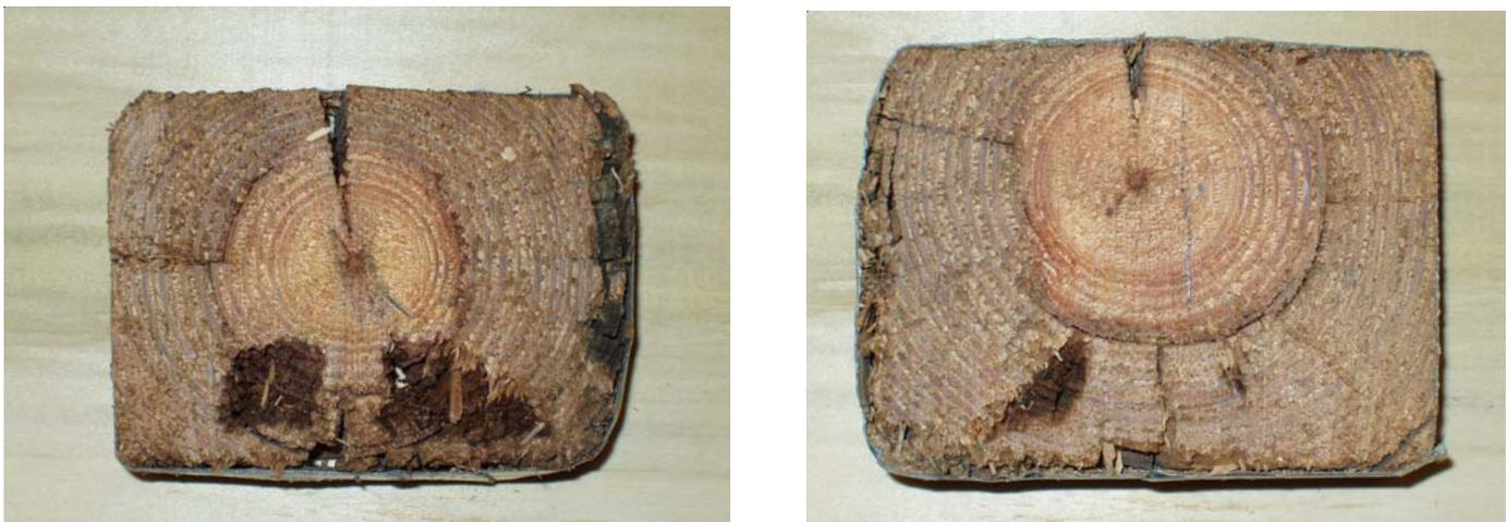
Figure III-19. Examples of cross sections cut from an older southern pine cross arm showing evidence of decay at the heartwood/sapwood interface.
