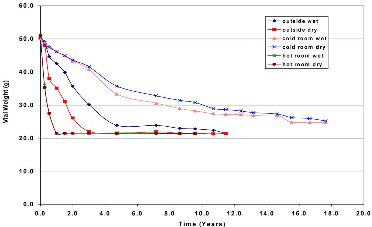
Figure I-1. MITC remaining in glass ampules installed in Douglas-fir pole sections exposed at 5 C, 32 C or ambient outdoor conditions.
