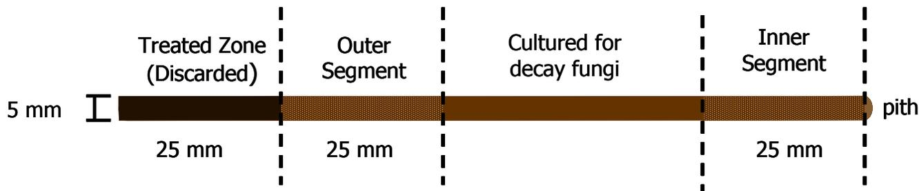
Figure I-3. Representation of increment core showing inner and outer 25 mm segments analyzed for fumigant content.
