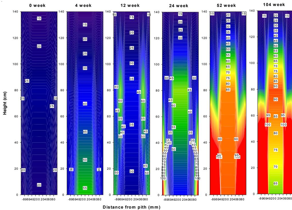
Figure III-13. Moisture contents of pentachlorophenol treated western redcedar poles wrapped with a Biotrans liner from the butt to the groundline and immersed in water for 0 to 104 weeks. Dark blue indicates moisture content below fiber saturation and red indicates moisture content above 80%.
