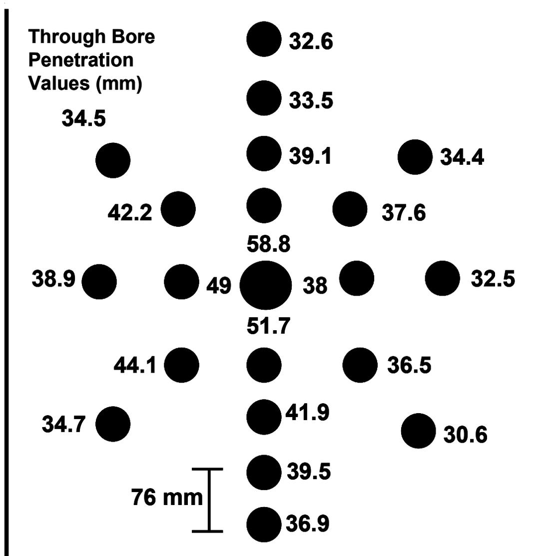
Figure III-2. Increment core sampling pattern employed to evaluate preservative penetration around the through-bored holes in Douglas-fir poles. Numbers represent the average penetration (mm) along cores removed from 3 holes in each of 5 pole sections.
