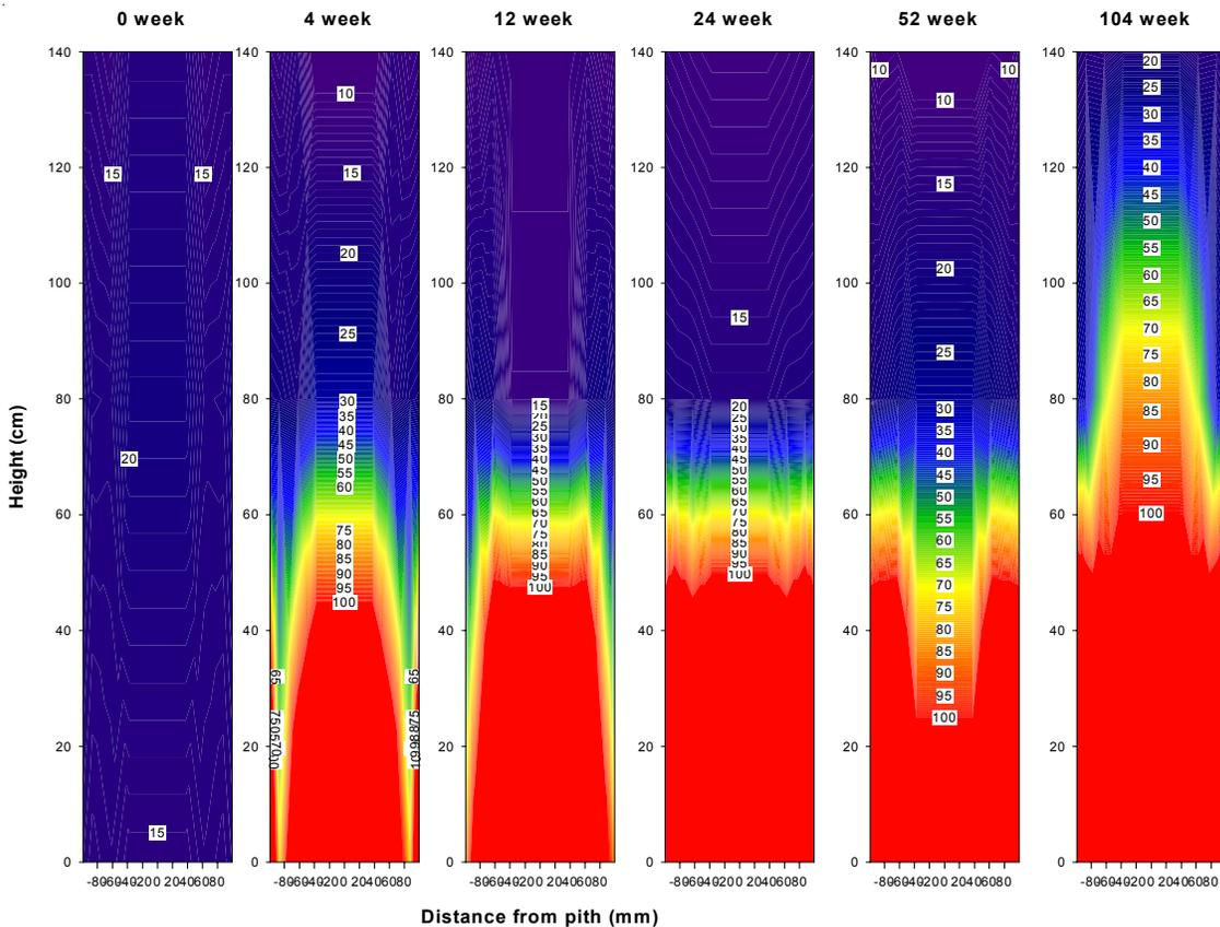
Figure III-8. Moisture contents of untreated western redcedar poles wrapped with a UPC liner from the butt to the groundline and immersed in moist soil for 0 to 104 weeks. Dark blue indicates moisture content below fiber saturation and red indicates moisture content above 80%.
