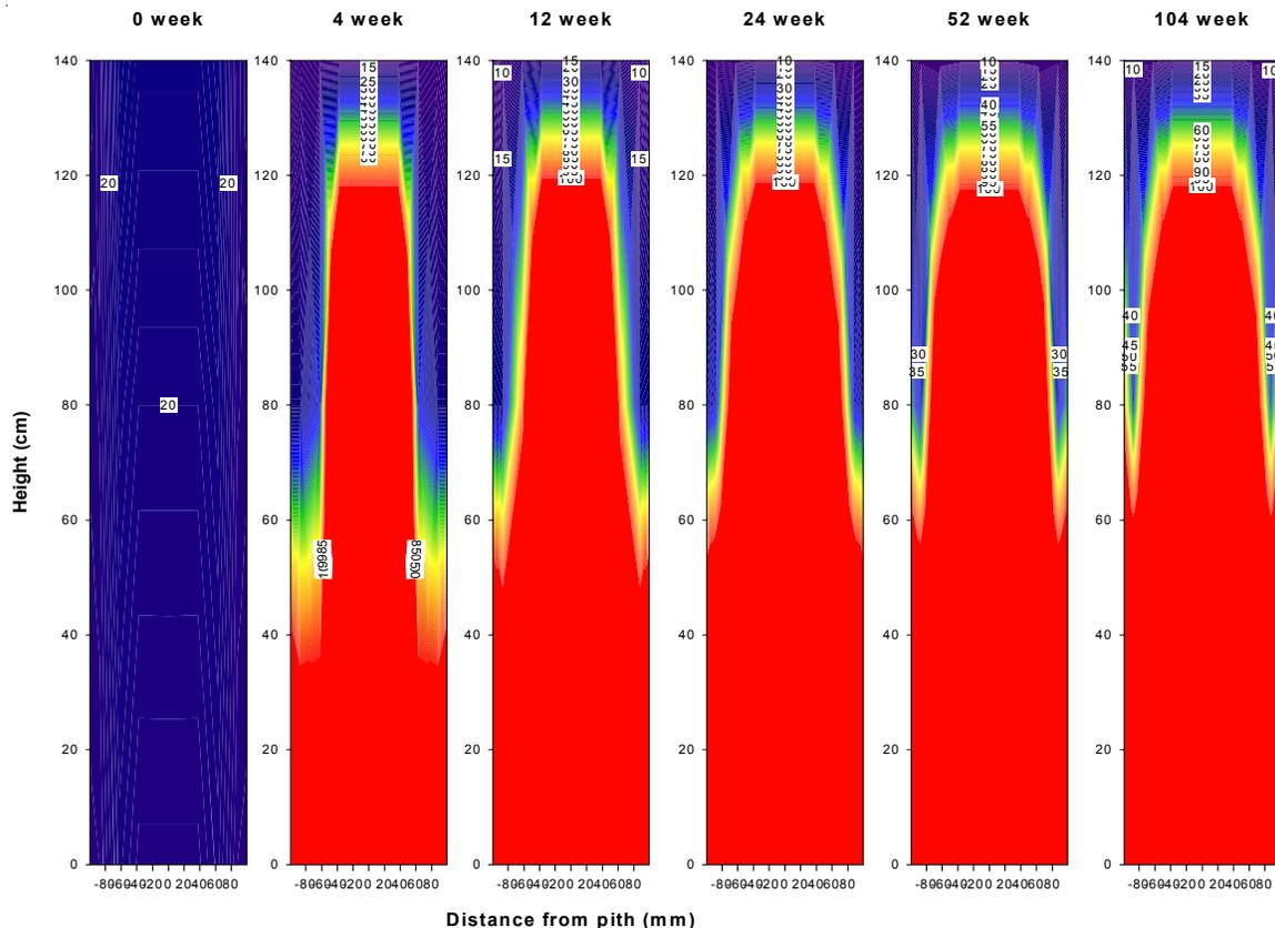
Figure III-6. Moisture contents of untreated western redcedar poles immersed in water for 0 to 104 weeks. Dark blue indicates moisture content below fiber saturation and red indicates moisture content above 80%.
