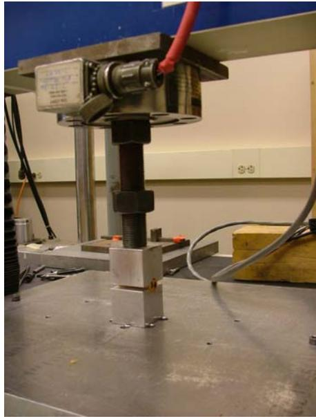
Figure III-22. Example of a longitudinal compression plug in the test jig prior to compression testing.
