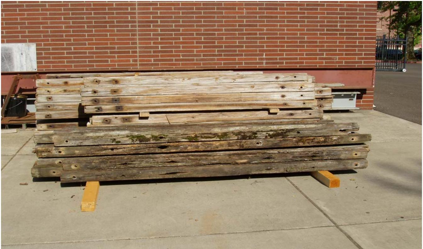
Figure III-15. Cross arms evaluated for residual flexural properties in four point loading. The arms in the foreground are Douglas-fir, while those in the background are southern pine.
