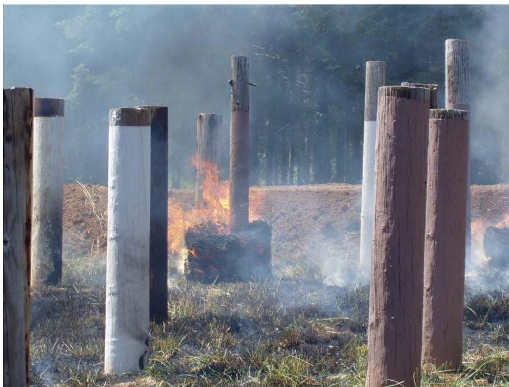
Figure III-30. Example of poles following ignition of the straw fuel.
