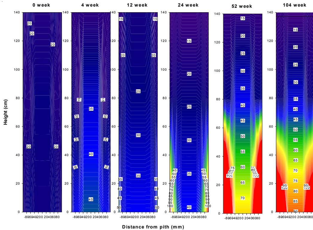
Figure III-9. Moisture contents of copper naphthenate treated western redcedar poles wrapped with a UPC liner from the butt to the groundline and immersed in water for 0 to 104 weeks. Dark blue indicates moisture content below fiber saturation and red indicates moisture content above 80%.
