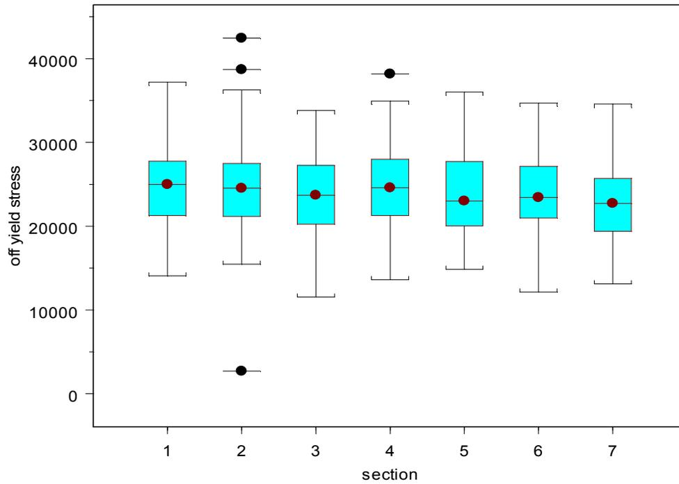
Figure III-25. Box and whisker plot of yield stress (psi) of 9 mm diameter plugs removed at one meter increments along the length of Douglas-fir poles as determined by testing in longitudinal compression.
