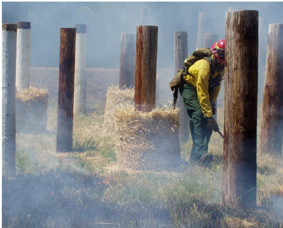
Figure III-29. Ignition of dried grass at the test burn site at Peavy Arboretum in 2006.
