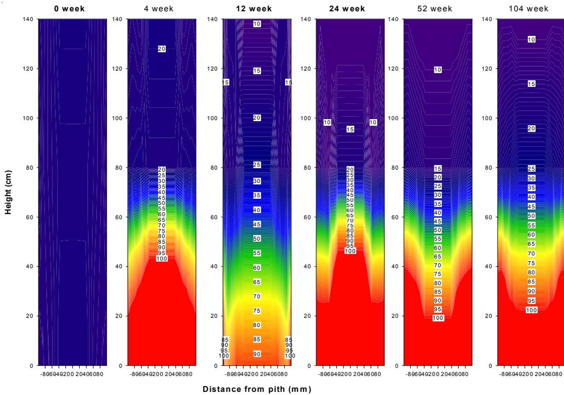
Figure III-7. Moisture contents of untreated western redcedar poles immersed in moist soil for 0 to 104 weeks. Dark blue indicates moisture content below fiber saturation and red indicates moisture content above 80%.
