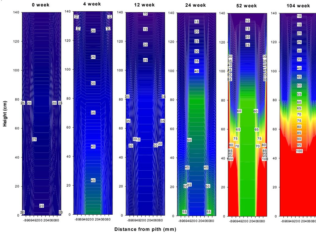
Figure III-11. Moisture contents of copper naphthenate treated western redcedar poles wrapped with a Biotrans liner from the butt to the groundline and immersed in water for 0 to 104 weeks. Dark blue indicates moisture content below fiber saturation and red indicates moisture content above 80%.
