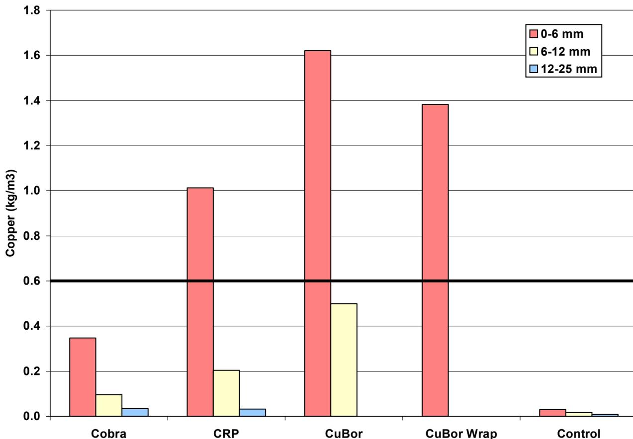
Figure IV-4. Residual copper levels at selected distances from the wood surface 150 mm below groundline on southern pine poles 1 year after treatment with Cobra Wrap, Cop-R-Plastic or CuBor in paste or bandage form.
