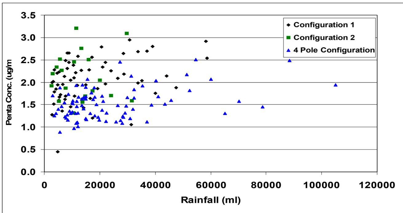
Figure VI-3. Penta concentrations as a function of total amount of rainfall collected in leachate from penta treated Douglas-fir poles following rainfall events over a 4.5 year exposure period showing data for three stacking configurations of poles.
