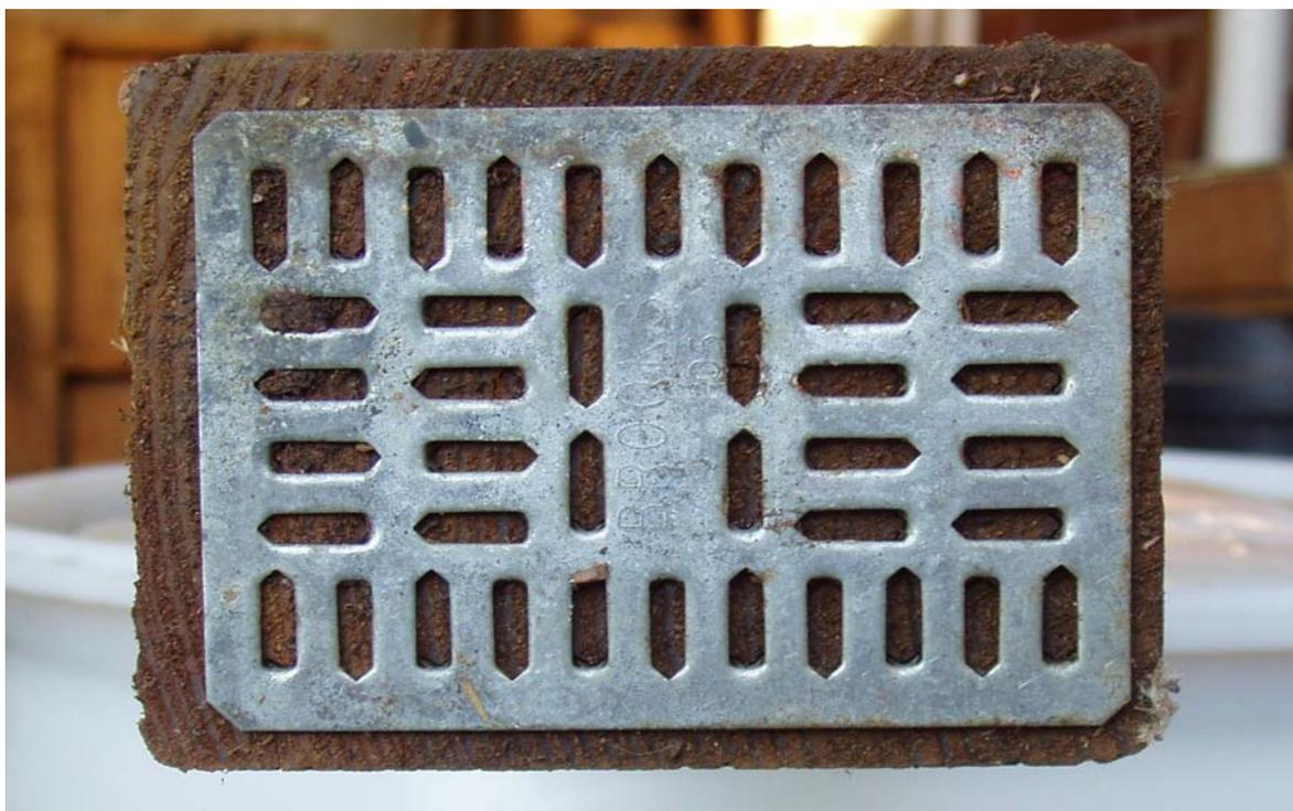
Figure III-34. Example of an end-plate on a penta treated Douglas-fir cross arm.
