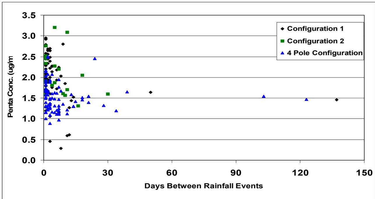
Figure VI-4. Penta concentrations as a function of intervals between collections (# of dry days) in leachate collected from penta treated Douglas-fir poles following rainfall events over a 4.5 year exposure period showing data for three stacking configurations of poles.
