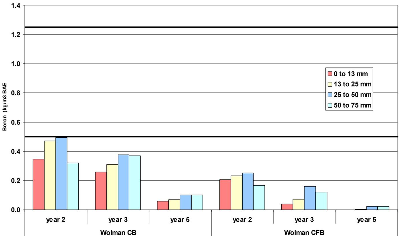
Figure IV-2. Residual boron levels at selected distances from the wood surface 150 mm below groundline on southern pine poles 2, 3 and 5 years after treatment with selected external supplemental preservative bandage systems.
