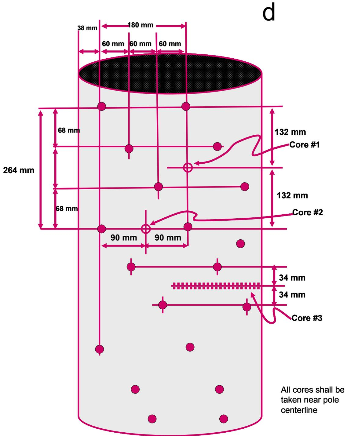
Figure III-4 (cont.). Patterns used by (a) Bonneville Power Administration or (b) Portland General Electric for through-boring of Douglas-fir poles at the groundline prior to treatment along with modifications of each patter (c, d).
