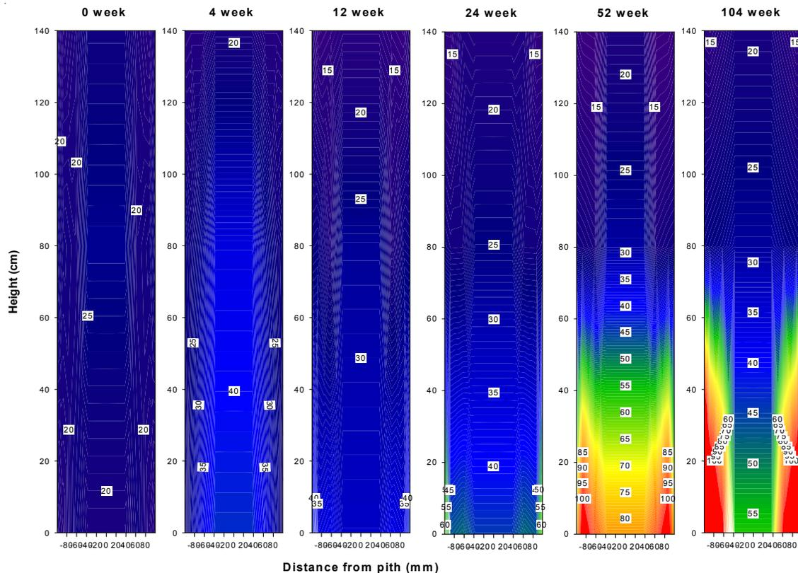
Figure III-14. Moisture contents of pentachlorophenol treated western redcedar poles wrapped with a Biotrans liner from the butt to the groundline and immersed in moist soil for 0 to 104 weeks. Dark blue indicates moisture content below fiber saturation and red indicates moisture content above 80%.
