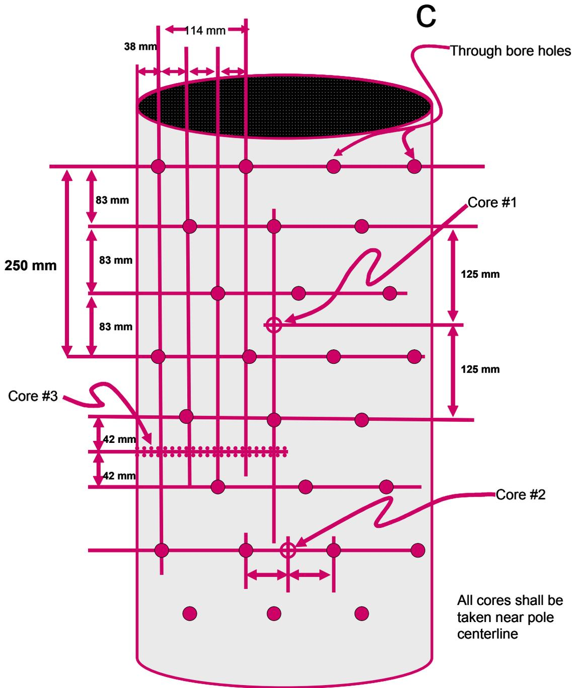
Figure III-4 (cont.). Patterns used by (a) Bonneville Power Administration or (b) Portland General Electric for through-boring of Douglas-fir poles at the groundline prior to treatment along with modifications of each patter (c, d).
