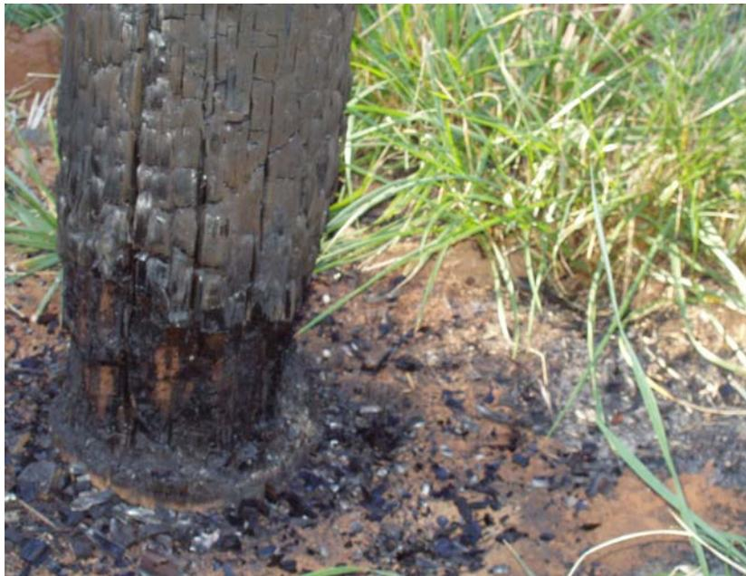
Figure III-32. Example of charring on a non-coated control pole surface following fire exposure.
