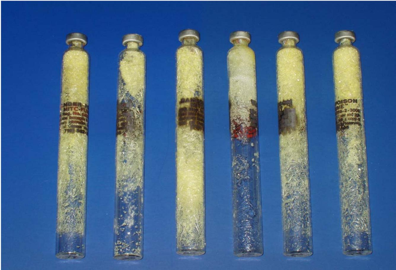
Figure I-2. MITC–FUME tubes 18 years after application to wet (3 tubes on left) or dry (3 tubes on right) Douglas-fir poles sections. The tubes contained 3.3, 2.1, 4.4, 4.9, 3.5, and 3.1 g of MITC, respectively, from the original approximately 30 g of MITC. Some of the material on the glass is elemental sulfur.
