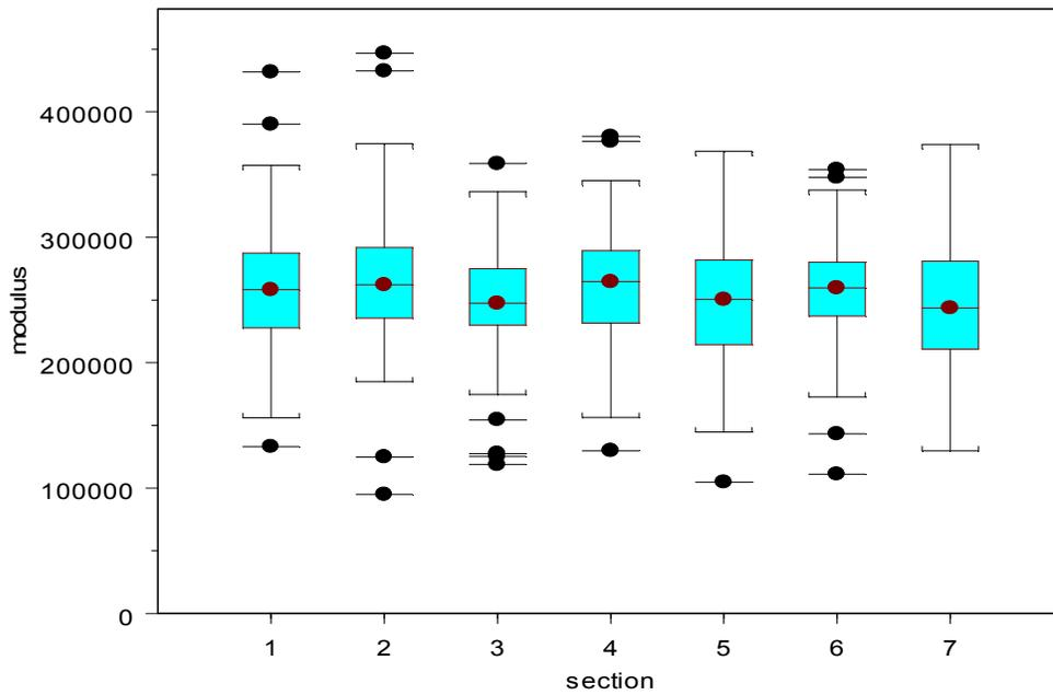
Figure III-23. Box and whisker plot of Modulus of elasticity (psi) of 9 mm diameter plugs removed at one meter increments along the length of Douglas-fir poles and tested in longitudinal compression.
