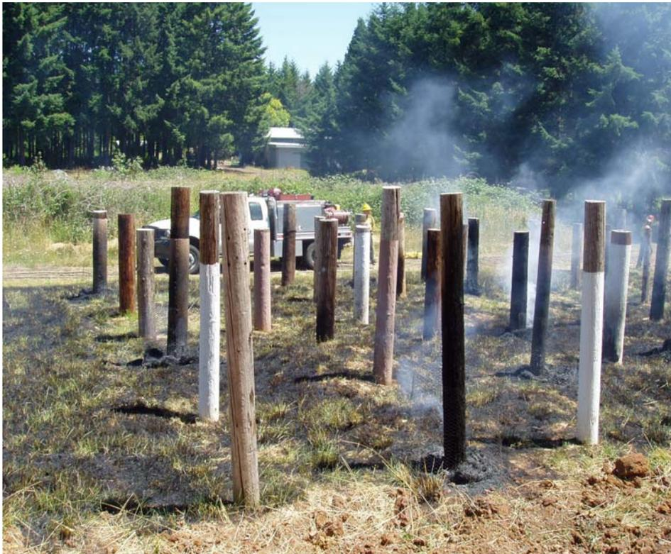
Figure III-31. View of the site after Douglas-fir poles with and without a fire retardant barrier were burned.
