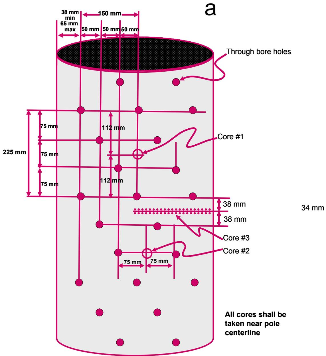
Figure III-4. Patterns used by (a) Bonneville Power Administration or (b) Portland General Electric for through-boring of Douglas-fir poles at the groundline prior to treatment along with modifications of each patter (c, d).
