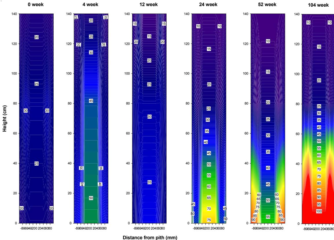
Figure III-12. Moisture contents of copper naphthenate treated western redcedar poles wrapped with a Biotrans liner from the butt to the groundline and immersed in moist soil for 0 to 104 weeks. Dark blue indicates moisture content below fiber saturation and red indicates moisture content above 80%.
