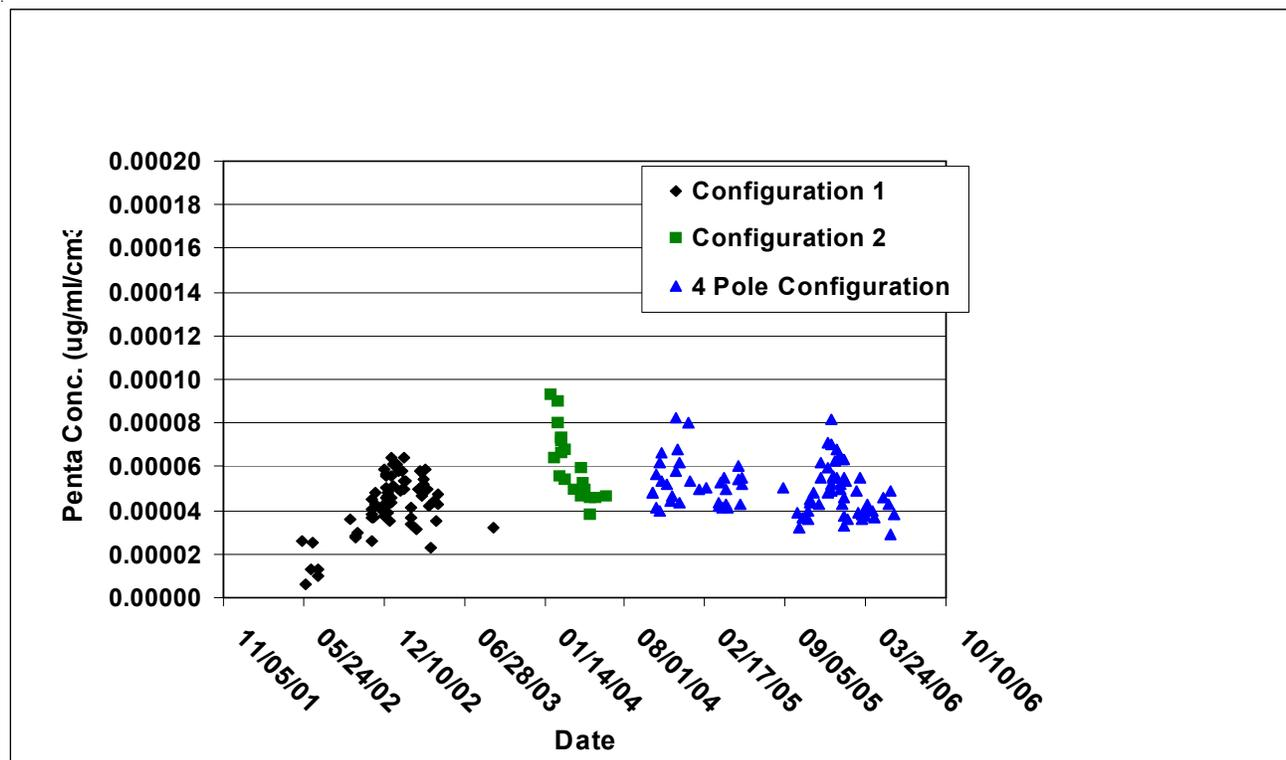
Figure VI-5. Concentration of pentachlorophenol in rainfall runoff from pentachlorophenol treated Douglas-fir pole sections stored in three stacking configurations as a function of total pole surface area.
