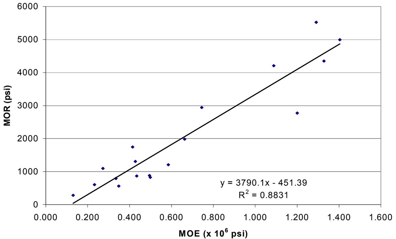
Figure III-20. MOR vs. MOE for weathered Douglas-fir cross arms tested to failure in four point loading.
