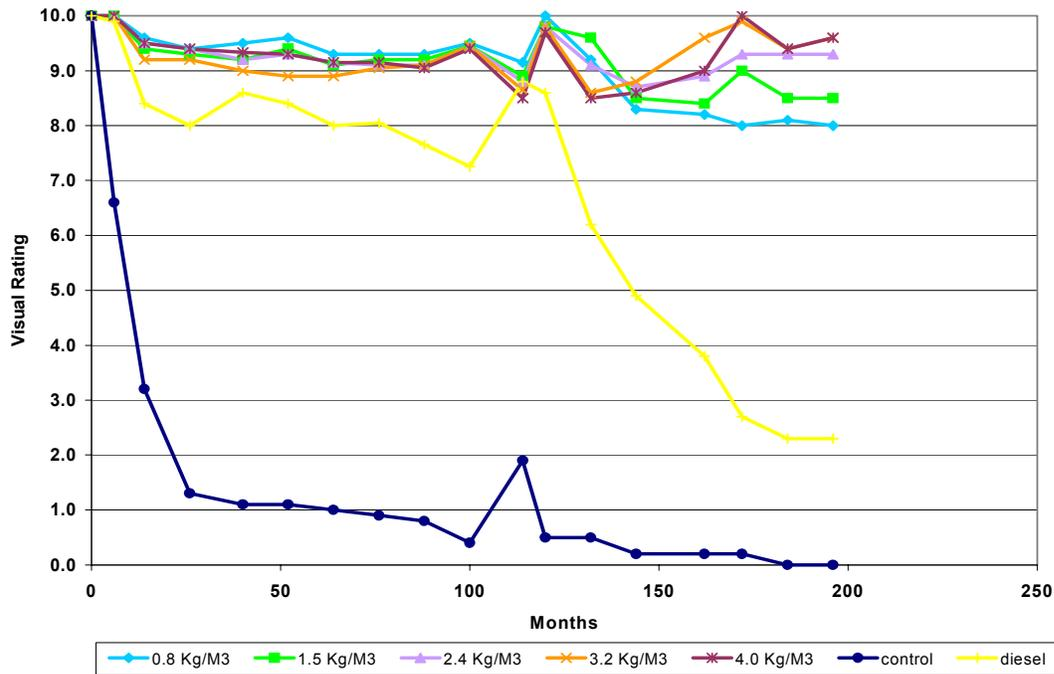
Figure V-1. Condition of freshly sawn western redcedar sapwood stakes treated with selected retentions of copper naphthenate in diesel oil and exposed in a soil bed for 196 months.
