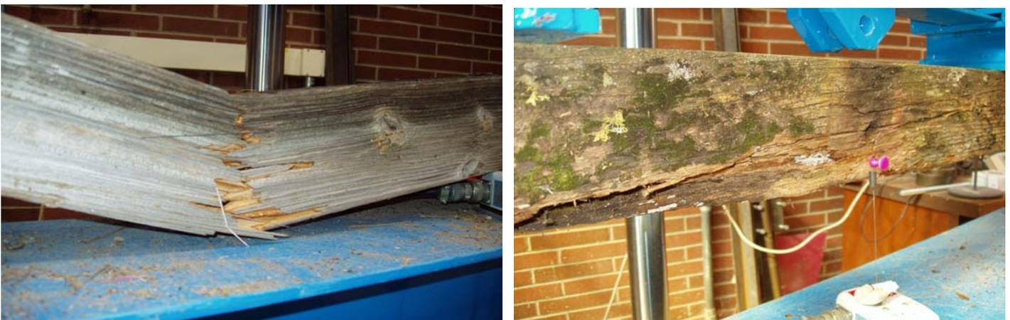
Figure III-21. Examples of failures of southern pine (left) and heavily weathered Douglas-fir (right) cross arms tested to failure in four point loading.
