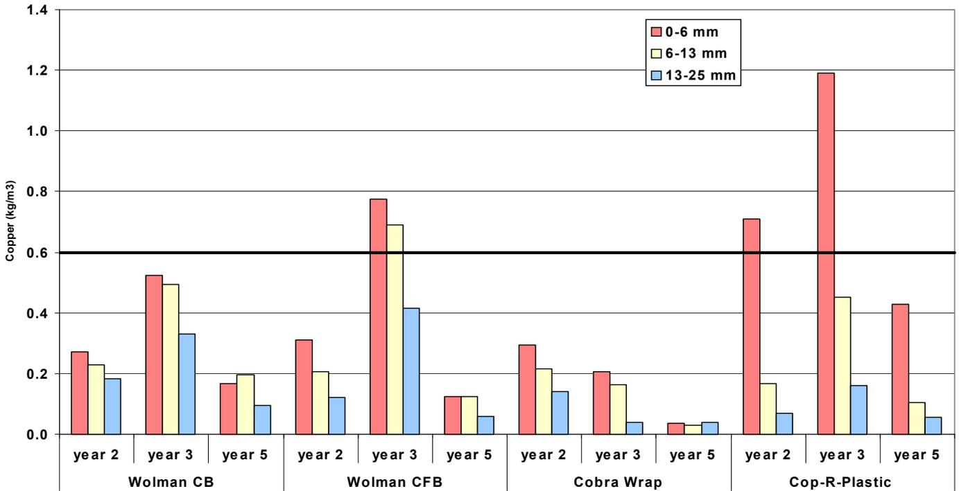
Figure IV-1. Residual copper levels at selected distances from the wood surface 150 mm below groundline on southern pine poles 2, 3 and 5 years after treatment with selected external supplemental preservative bandage systems.
