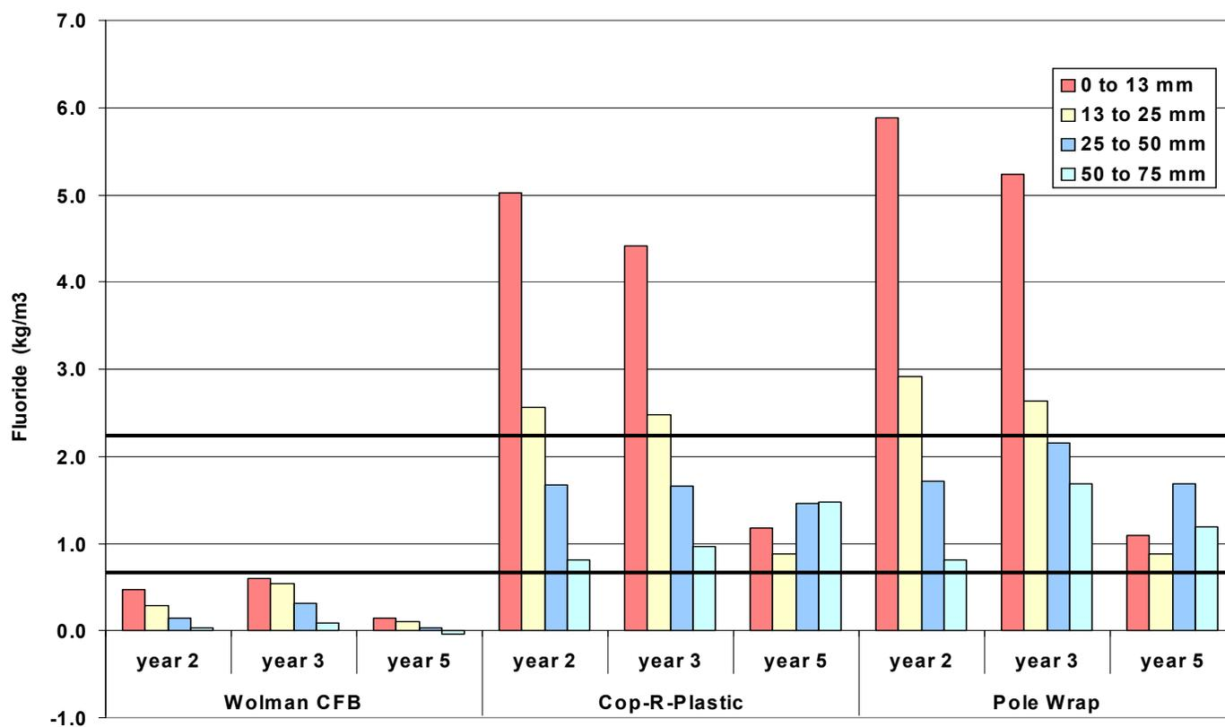
Figure IV-3. Residual fluoride levels at selected distances from the wood surface 150 mm below groundline on southern pine poles 2, 3, and 5 years after treatment with selected external supplemental preservative bandage systems.
