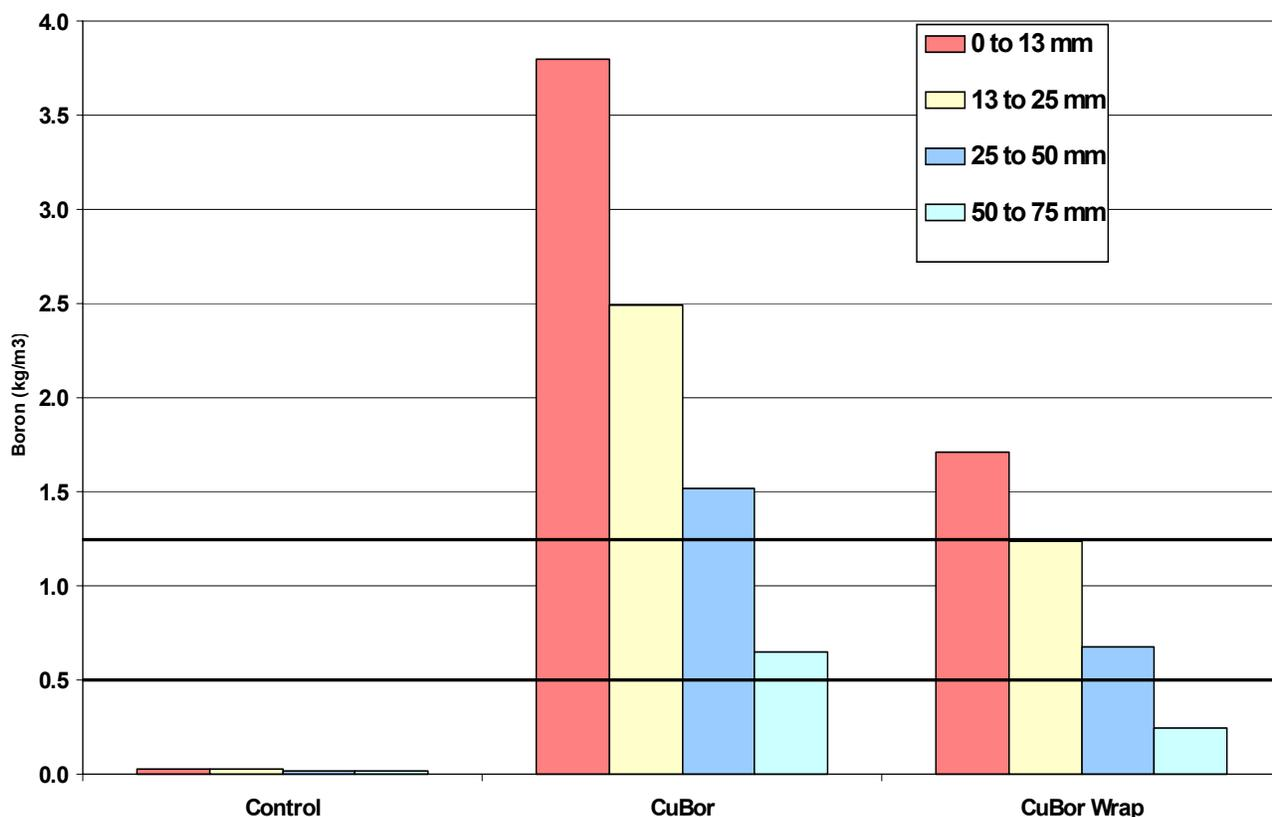
Figure IV-5. Residual boron levels at selected distances from the wood surface 150 mm below groundline on southern pine poles 1 year after treatment with CuBor in paste or bandage form.
