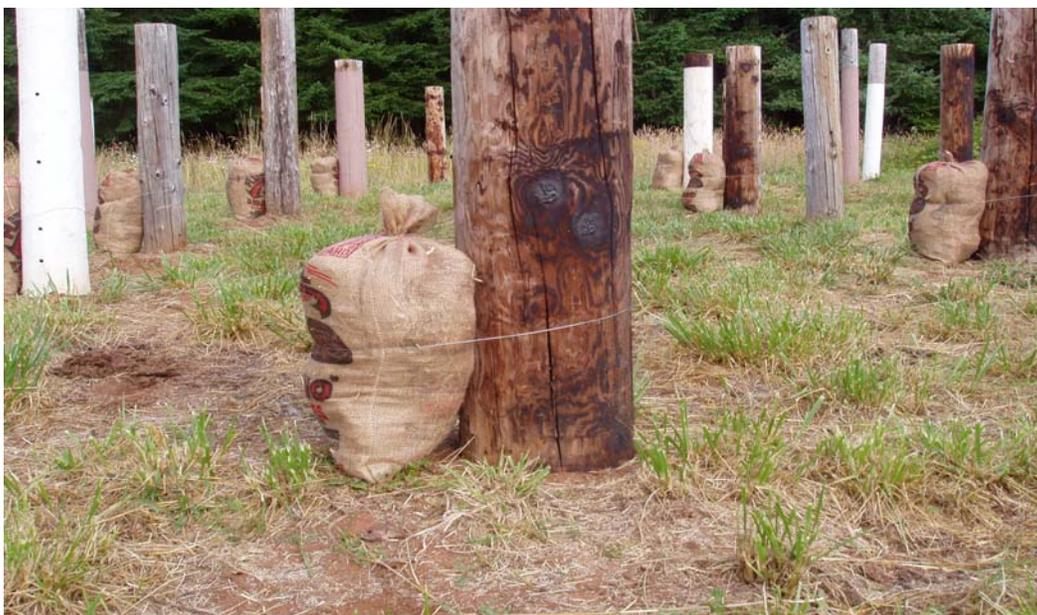
Figure III-26. Example of straw fuel in burlap bags tied around Douglas-fir poles with or without a fire retardant barrier.
