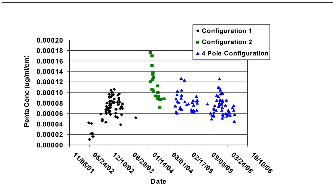
Figure VI-6. Concentration of pentachlorophenol in rainfall runoff from pentachlorophenol treated Douglas-fir pole sections stored in three stacking configurations as a function of only pole surface area exposed to direct rainfall.
