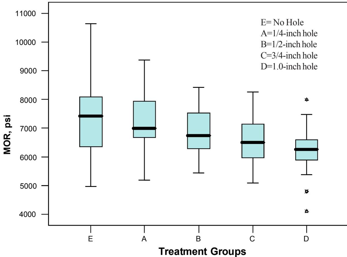
Figure III-5. MOR of Douglas-fir poles with through-boring holes of differing hole diameters. The boxed area represents 50 percent of each data set; the line through the shaded area is the median value. The bars represent the outer limits for the data except where there are outliers, which is only the case for the 1-inch treatment group. The outliers, represented by the stars, are determined as those points that lie outside 1.5 times the inner-quartile range of the plots.
