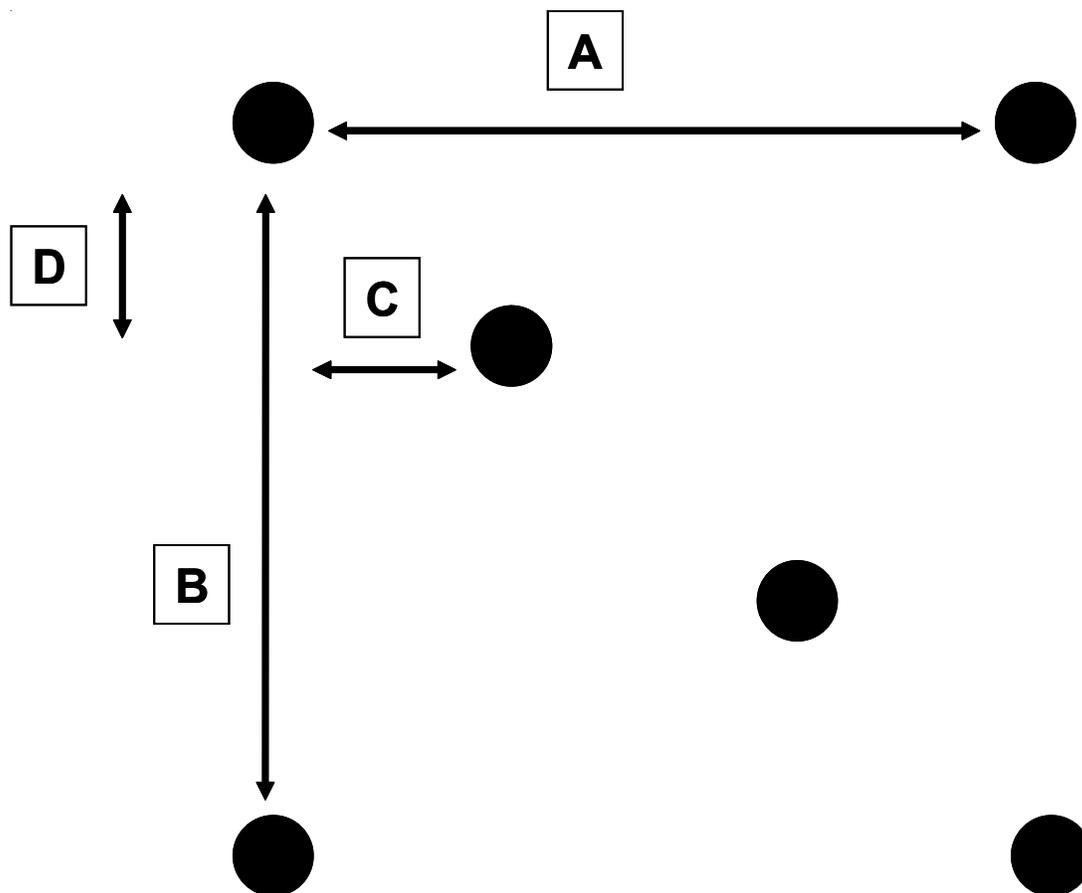
Figure III-3. Distances between holes drilled into Douglas-fir poles to assess the effect of through-boring pattern on treatment.
