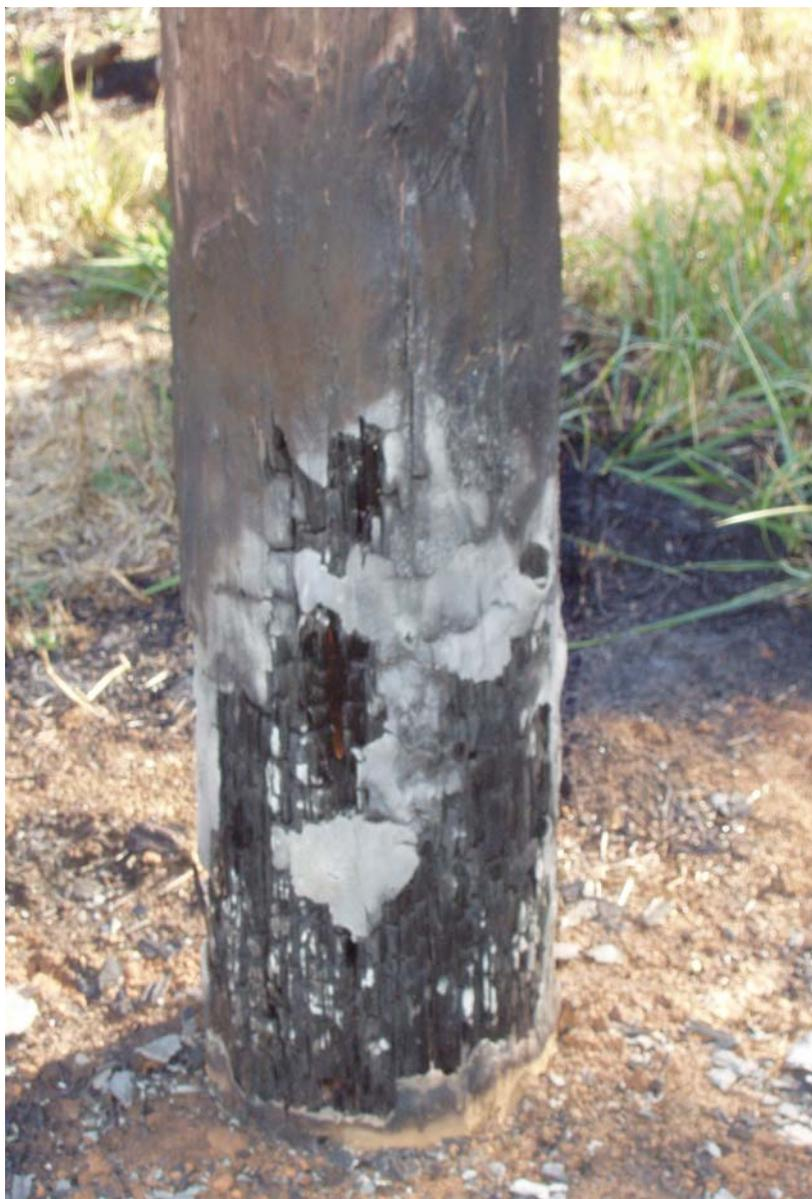
Figure III-33. Example of a fire retardant treated pole following fire exposure.
