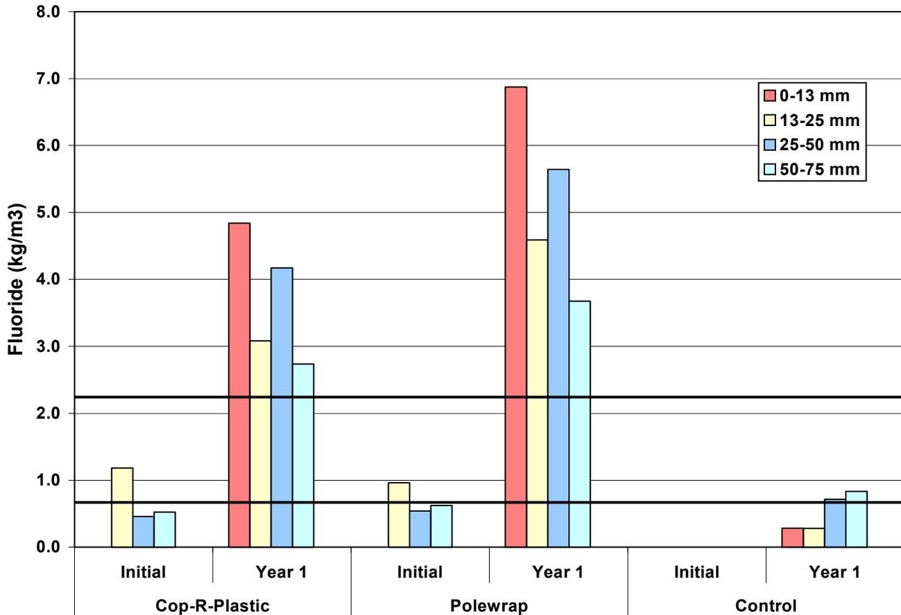
Figure IV-6. Residual fluoride levels at selected distances from the wood surface 150 mm below groundline on southern pine poles 1 year after treatment with Cop-R-Plastic or Pole Wrap.
