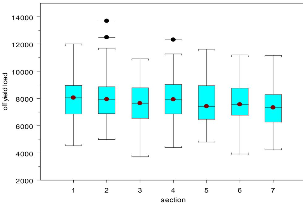
Figure III-24. Box and whisker plot of yield load (lbs of force) of 9 mm diameter plugs removed at one meter increments along the length of Douglas-fir poles as determined by testing in longitudinal compression.
