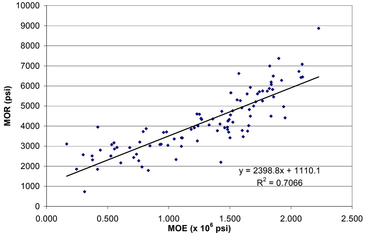
Figure III-17. Relationship between modulus of rupture (MOR) and modulus of elasticity (MOE) of weathered southern pine cross arms tested to failure in four point loading.
