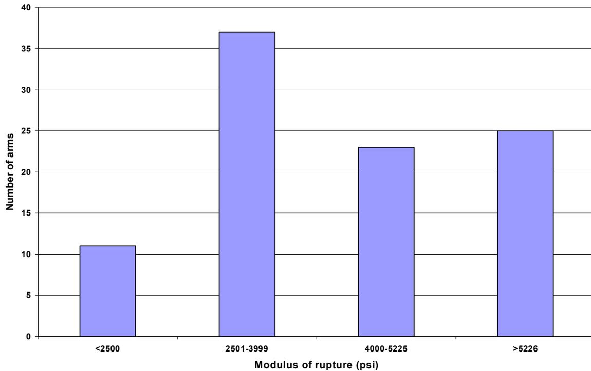
Figure III-18. Modulus of rupture distribution in a population of 96 weathered southern pine cross arms tested to failure in four point loading.
