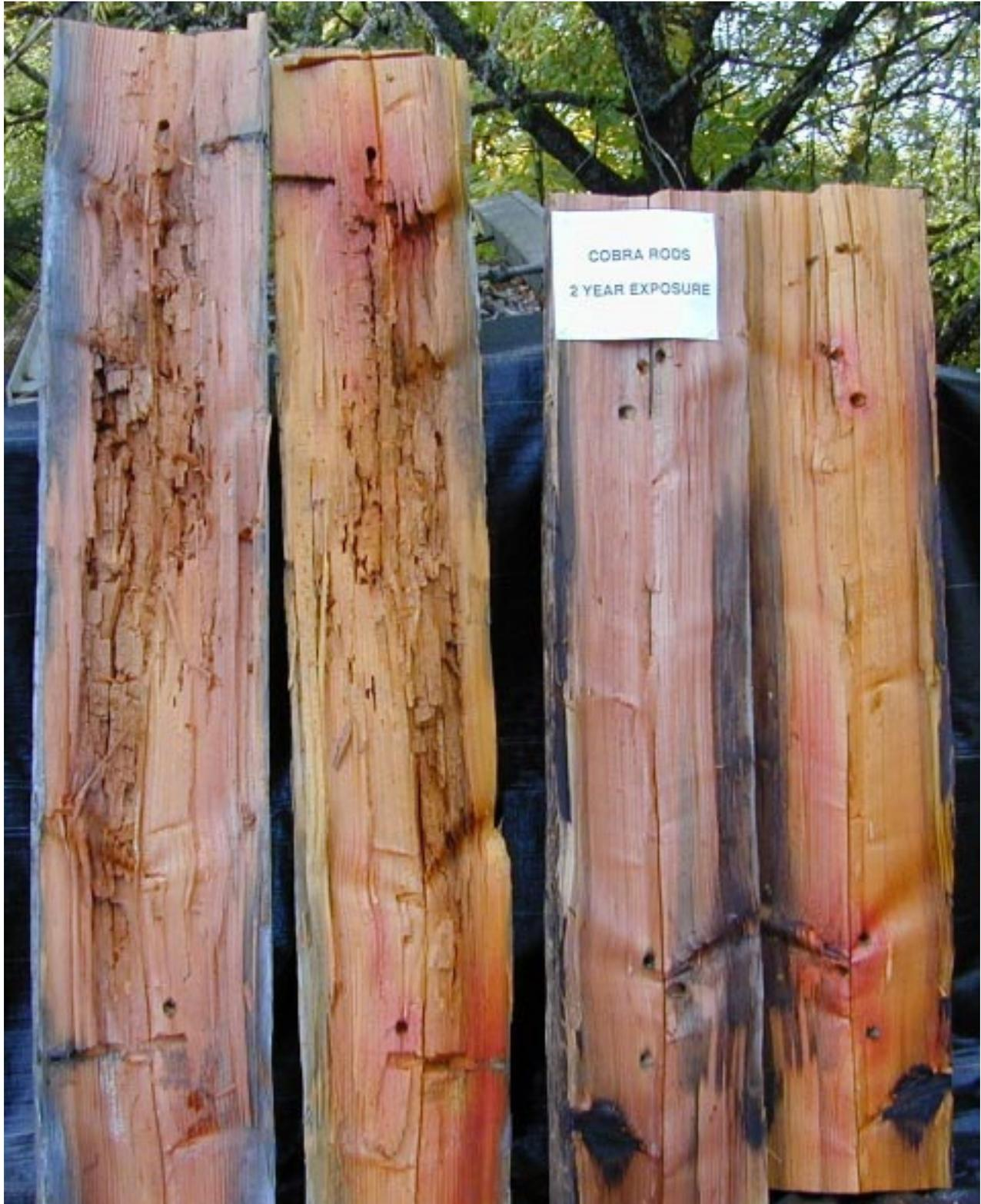
Figure I-30. Degree of fluoride movement in Douglas-fir pole sections two years after treatment with fluoride rods in three holes drilled around the pole at two locations one meter apart as determined using an indicator which turns yellow in the presence of fluoride.
