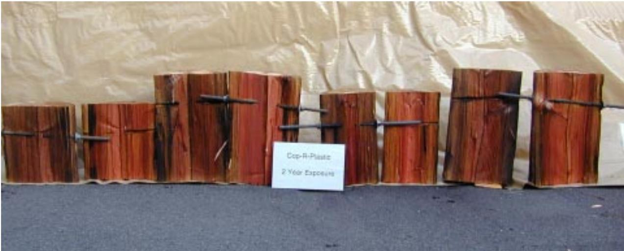
Figure II-3. Degree of copper and boron movement away from the sites in Douglas-fir poles where CuRap 20 coated galvanized rods were installed two years earlier.
