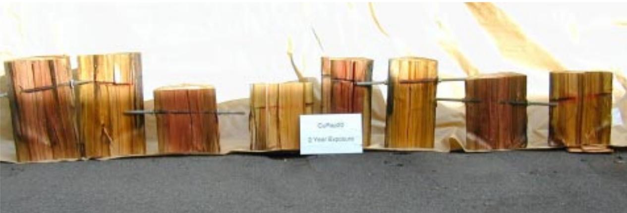
Average boron movement tended to be better 2 years after treatment than fluoride movement, although the maximum distance of fluoride movement was nearly two times higher. In most of our tests, fluoride has tended to move more slowly and at apparently lower levels than boron. Our results for average movement in these tests follow that trend, although it appears that, when conditions are suitable, fluoride can diffuse for considerable distances from the point of application.
