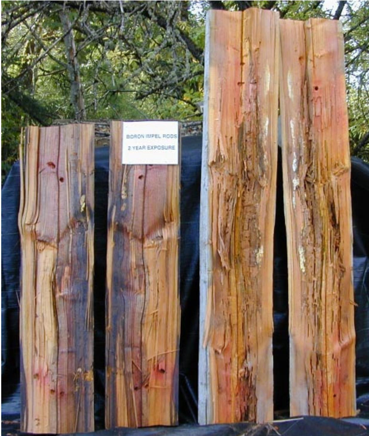
Figure I-29. Degree of boron and copper movement in Douglas-fir pole sections two years after treatment with fused borate/copper rods in three holes drilled around the pole at two locations one meter apart as determined using indicators that turn red in the presence of boron or green in the presence of copper.
