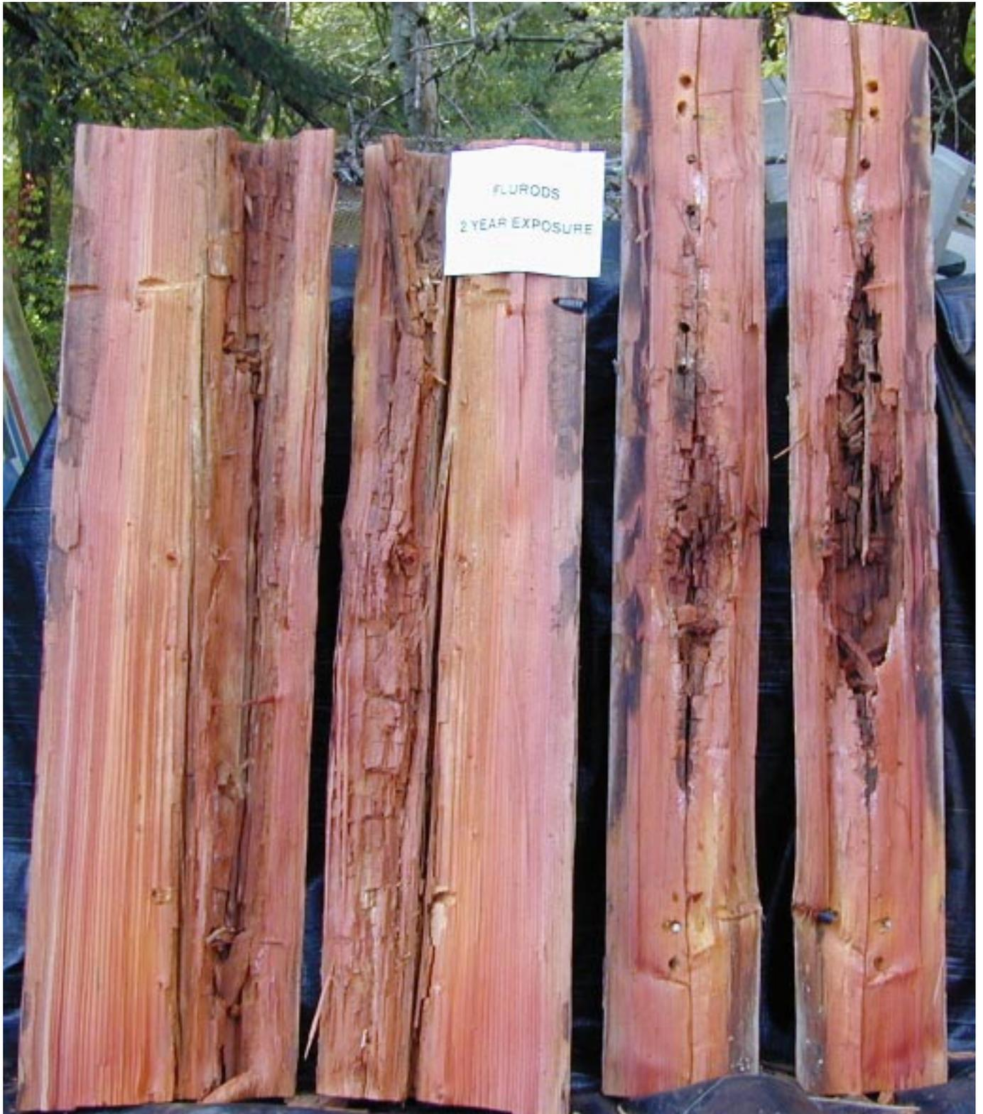
Table I-20. Degree of fluoride, boron or copper movement from remedial treatment rods applied to Douglas-fir pole sections that were then exposed for one or two years near Salem, Oregon.
