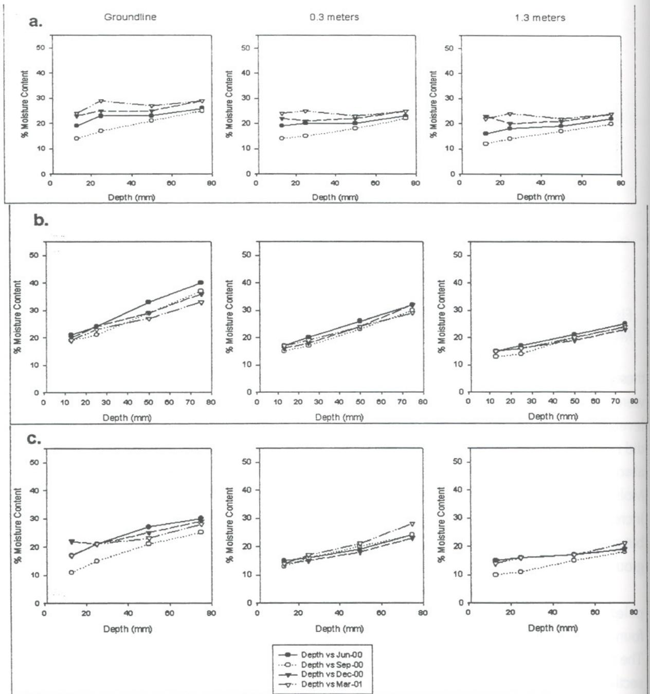
Figure III-2. Wood Moisture content at selected depths for kerfed Douglas-fir poles treated with a) pentachlorophenol, b) creosote or c) deeply incised and creosoted.
