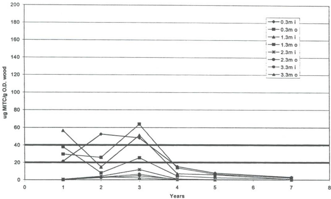
Figure I-4. MITC levels at selected distances above the groundline in Douglas-fir transmission poles 1 to 7 years after treatment with 500 ml of metham sodium.
