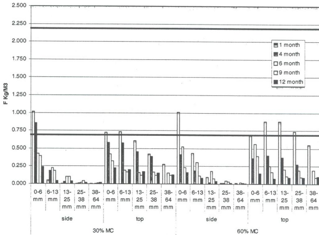
Figure IV-6. Fluoride levels at selected distances from the surface of Douglas-fir heartwood blocks at 30 or 60 % MC 1 to 12 months after application of a copper/boron/fluoride bandage.
