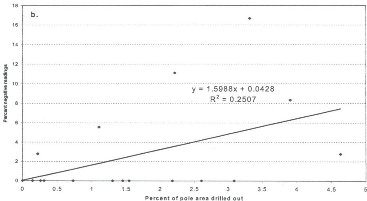
Figure III-19. Frequency of negative readings from the Purl inspection device on Douglas-fir pole sections with increasing amounts of wood removal a) to one side of the pole or b) from the center of the pole.
