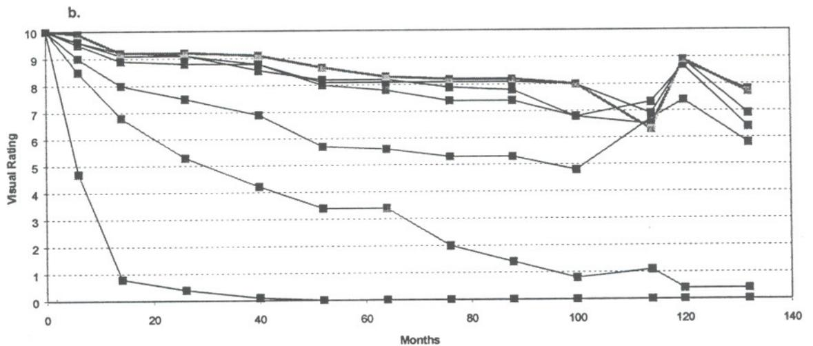
Figure IV-1. Conditions of a) freshly harvested and b) weathered western redcedar sapwood stakes treated with selected retentions of copper naphthenate and exposed for 132 months in a fungus cellar.
