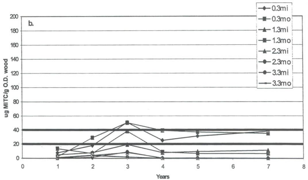
Figure I-2. MITC levels at selected distances above the groundline in Douglas-fir transmission poles 1 to 7 years after treatment with 200 g of basamid a) with or b) without copper sulfate
