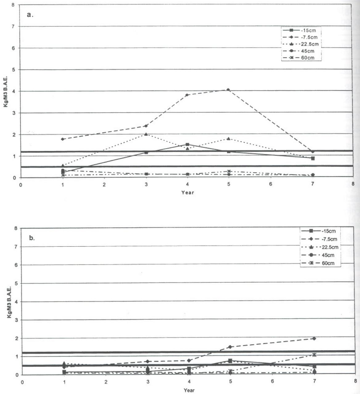
Figure I-5. Boron levels in the a) inner and b) outer regions of Douglas-fir pole sections 1 to 7 years after treatment with 180 g of fused boron rod.
