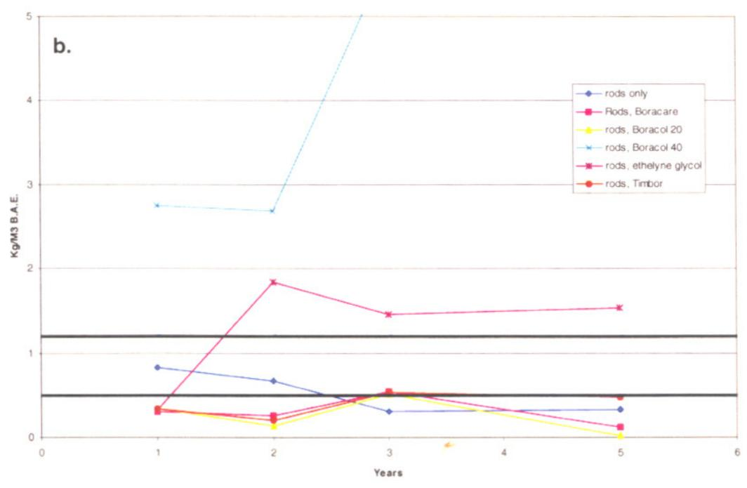
Figure 1-10. Boron levels in the outer (a), middle (b), and inner (c) zones of increment cores removed 300 mm above groundline from Douglas-fir poles sections 1 to 5 years after treatment with fused boron rods with or without various diffusion enhancers.
