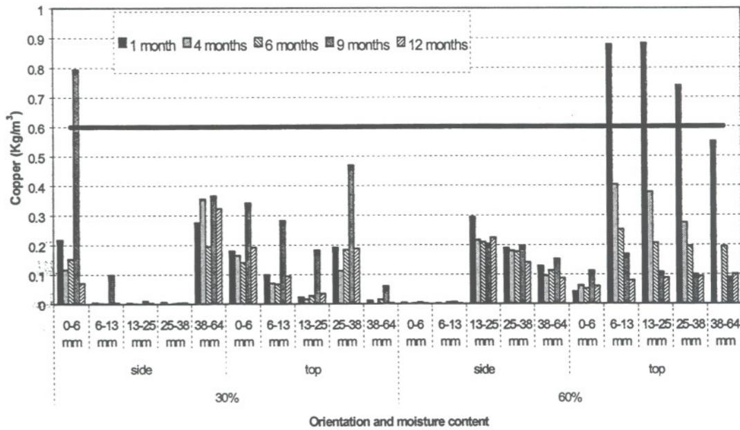
Figure IV-4. Copper levels at selected distances from the surface of Douglas-fir heartwood blocks at 30 or 60 % MC 1 to 12 months after application of a copper/boron/fluoride bandage.
