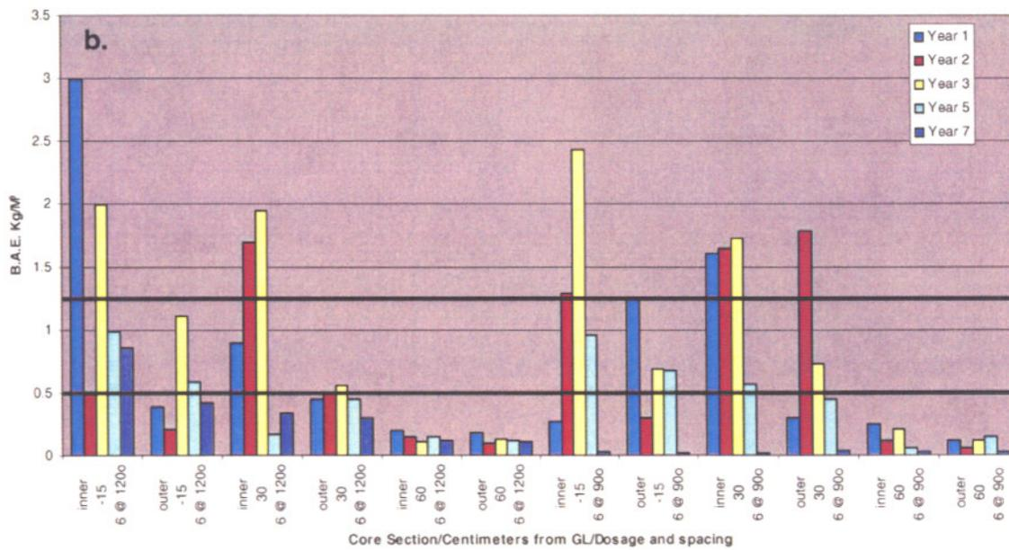
Figure 1-12. Residual levels of boron in Douglas-fir poles 1 to 7 years after treatment with 2) three or b) six fluoride/boron rods distributed in holes spaced 90 or 120 degrees around the pole.
