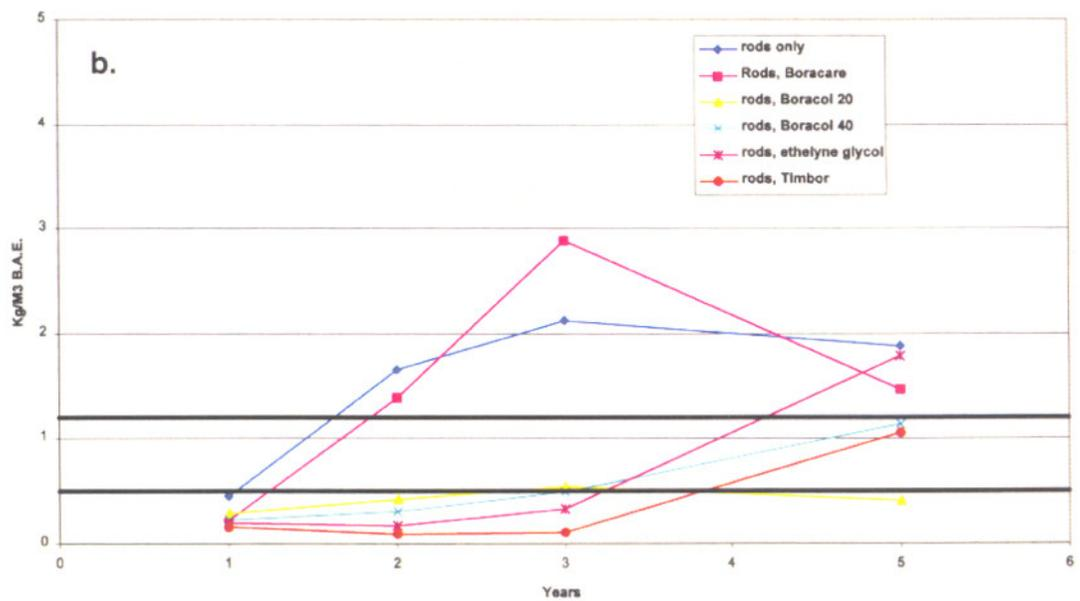
Figure 1-7. Boron levels in the outer (a), middle (b), and inner (c) zones of increment cores removed 300 mm below groundline from Douglas-fir poles sections 1 to 5 years after treatment with fused boron rods with or without various diffusion enhancers.
