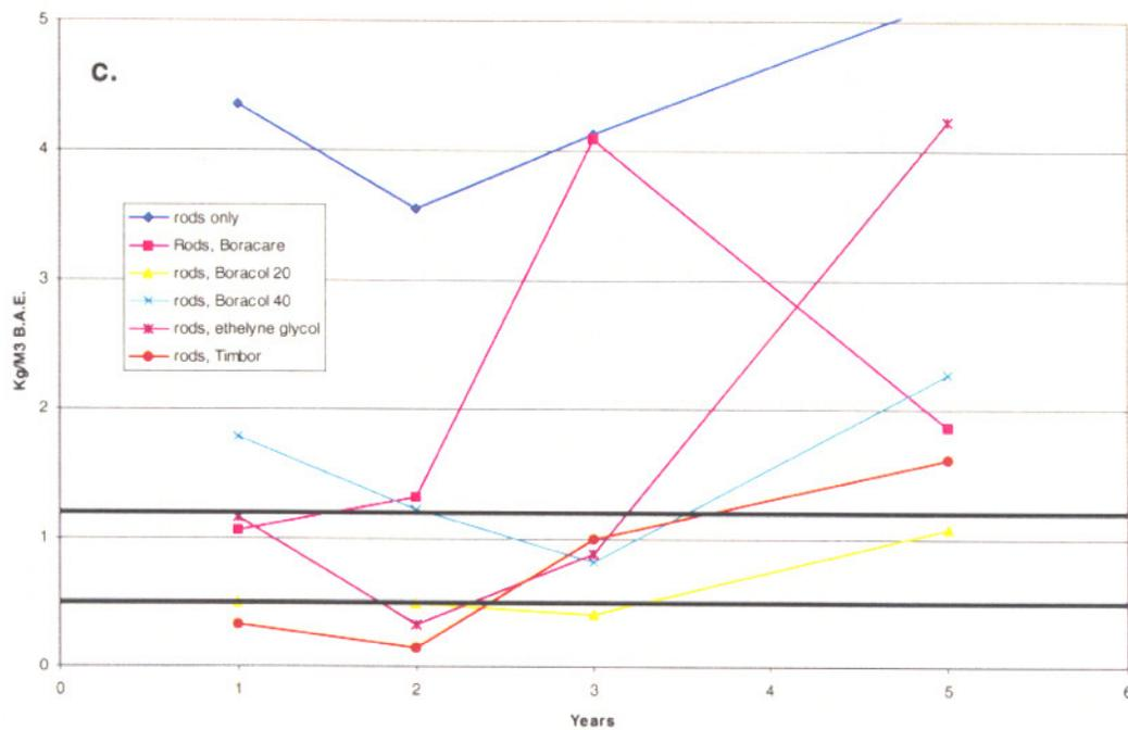
Figure 1-8 cont. Boron levels in the outer (a), middle (b), and inner (c) zones of increment cores removed at groundline from Douglas-fir poles sections 1 to 5 years after treatment with fused boron rods with or without various diffusion enhancers.
