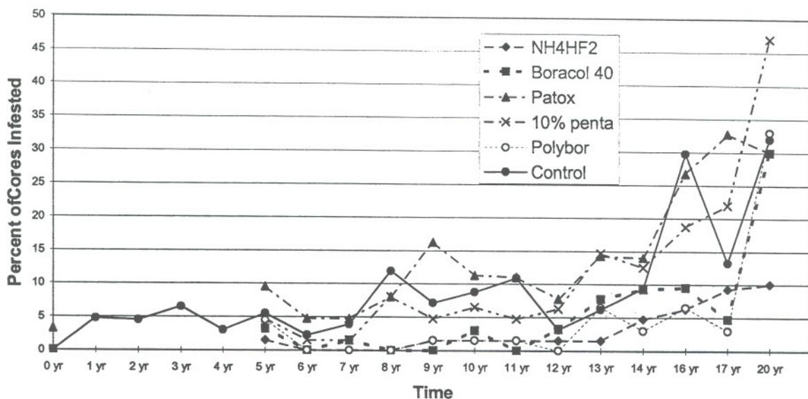
Figure II-1. Effect of application of supplemental treatments to field drilled bolt holes in Douglas-fir poles on the isolation frequency of decay fungi 1 to 20 years after treatment.
