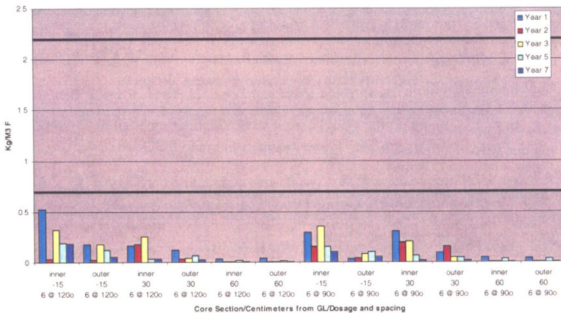
Figure 1-13. Residual levels of fluoride in Douglas-fir poles 1 to 7 years after treatment with three or b) six fluoride/boron rods distributed in holes spaced 90 or 120 degrees around the pole.
