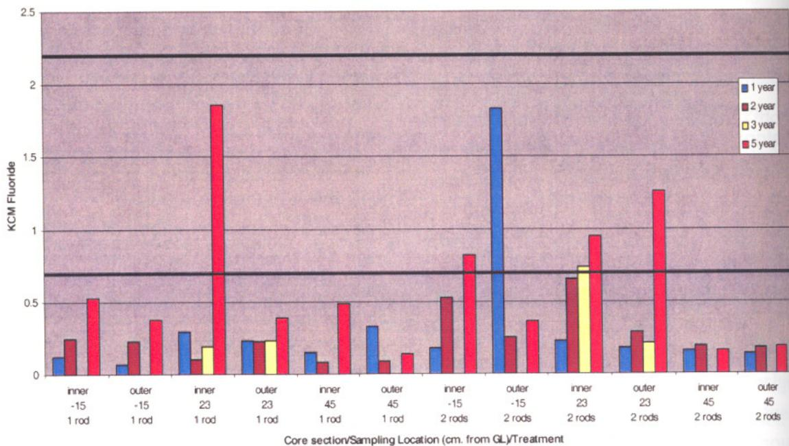
Figure 1-11. Fluoride concentrations at selected distances above or below groundline in Douglas-fir pole section 1 to 5 years after treatment with 3 or 6 fluoride rods per pole.
