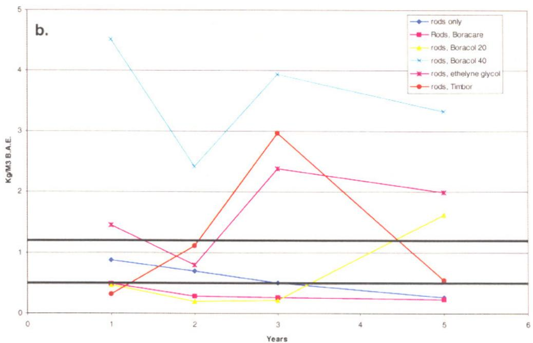
Figure 1-8. Boron levels in the outer (a), middle (b), and inner (c) zones of increment cores removed at groundline from Douglas-fir poles sections 1 to 5 years after treatment with fused boron rods with or without various diffusion enhancers.
