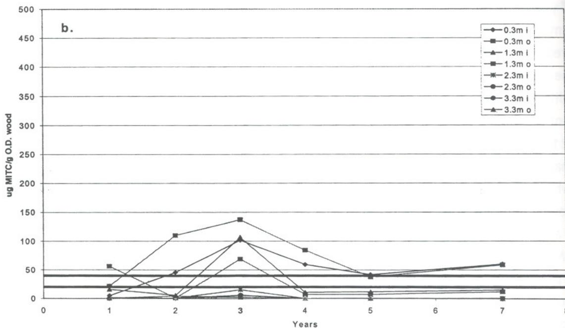
Figure I-3. MITC levels at selected distances above the groundline in Douglas-fir transmission poles 1 to 7 years after treatment with 400 g of basamid a) with or b) without copper sulfate
