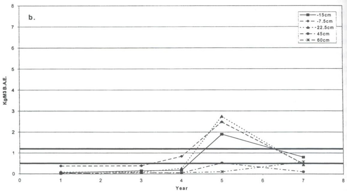
Figure 1-6. Boron levels in the a) inner and b) outer regions of Douglas-fir pole sections 1 to 7 years after treatment with 360 g of fused boron rod.
