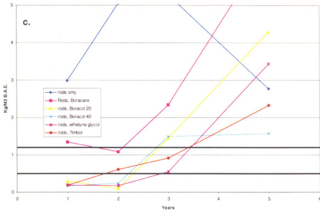
Figure 1-10 cont. Boron levels in the outer (a), middle (b), and inner (c) zones of increment cores removed 300 mm above groundline from Douglas-fir poles sections 1 to 5 years after treatment with fused boron rods with or without various diffusion enhancers.
