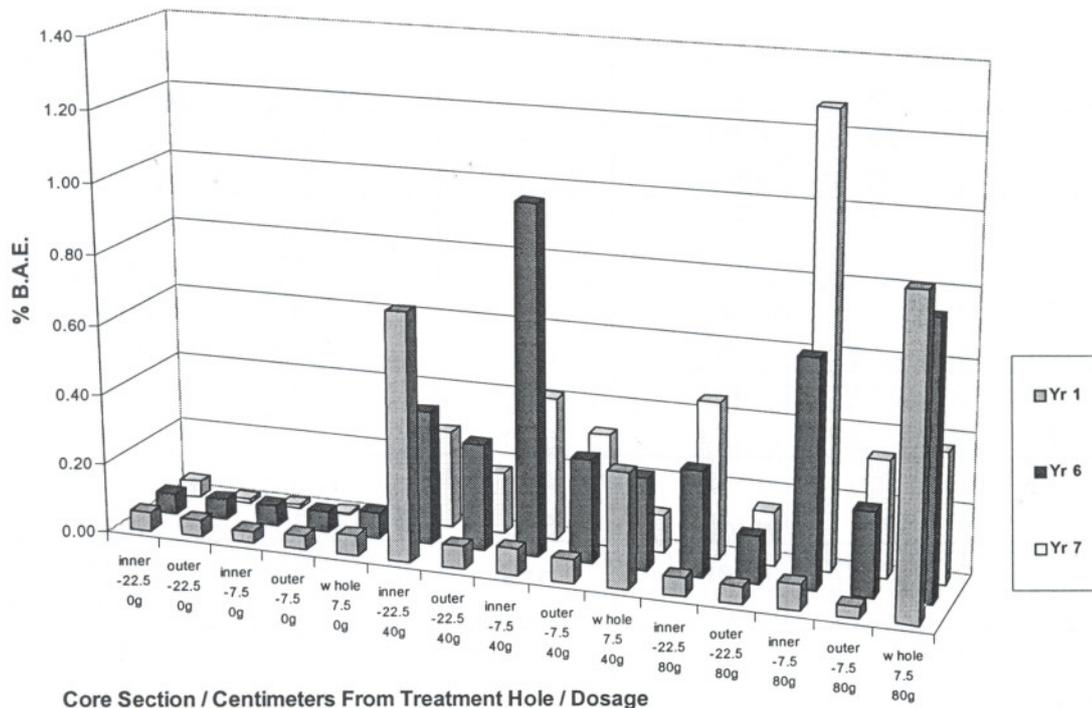
treated shell was discarded, then the remaining wood was split into inner and outer halves which were ground to pass a 20 mesh screen. The samples were then ashed and the resulting material was resolubilized and analyzed using a specific ion electrode as described in American Wood Preservers' Association Standard A2. The samples are being analyzed by Osmose Wood Preserving on a coded sample basis, but the results of the analysis are not yet available.
