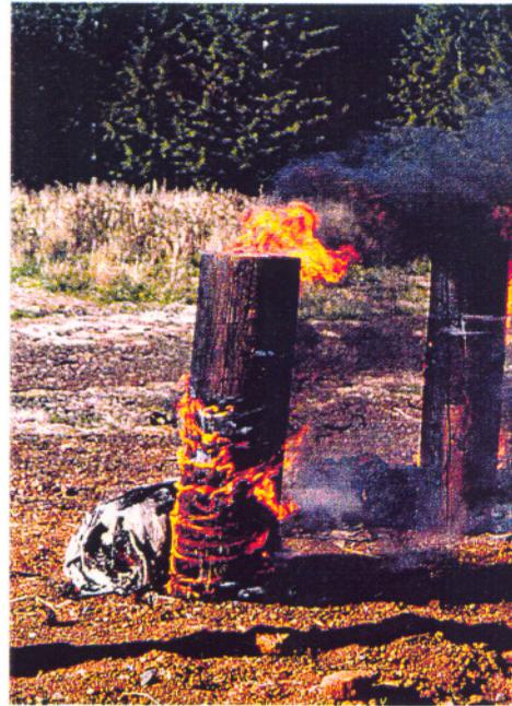
Figure III-10. Pentachlorophenol treated pole burning during the fire test.
