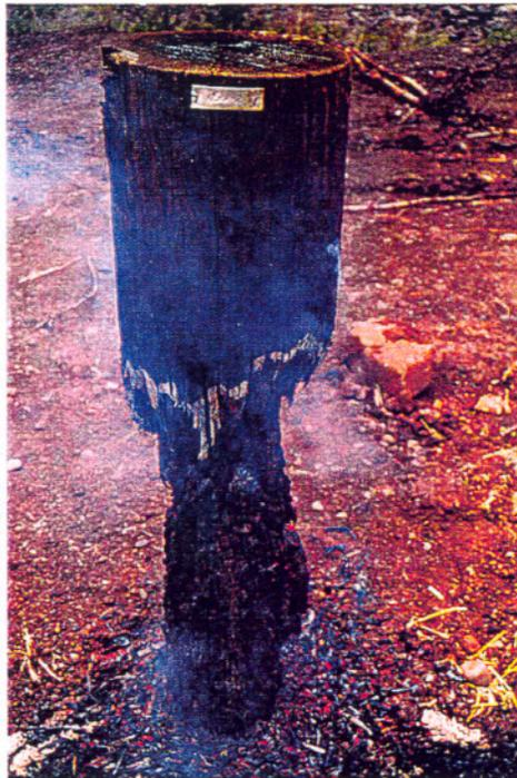
Figure III-12. ACZA-treated Douglas-fir pole exhibiting extensive cross sectional area loss around the groundline following exposure to a 9 minute straw fire.
