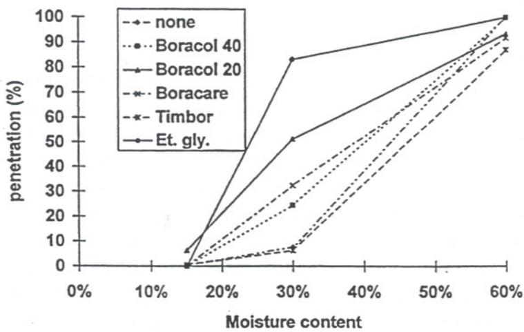
Figure I-14. Boron penetration 60 mm from the ends of Douglas-fir heartwood blocks 8 or 12 weeks after application of various boron treatments.
