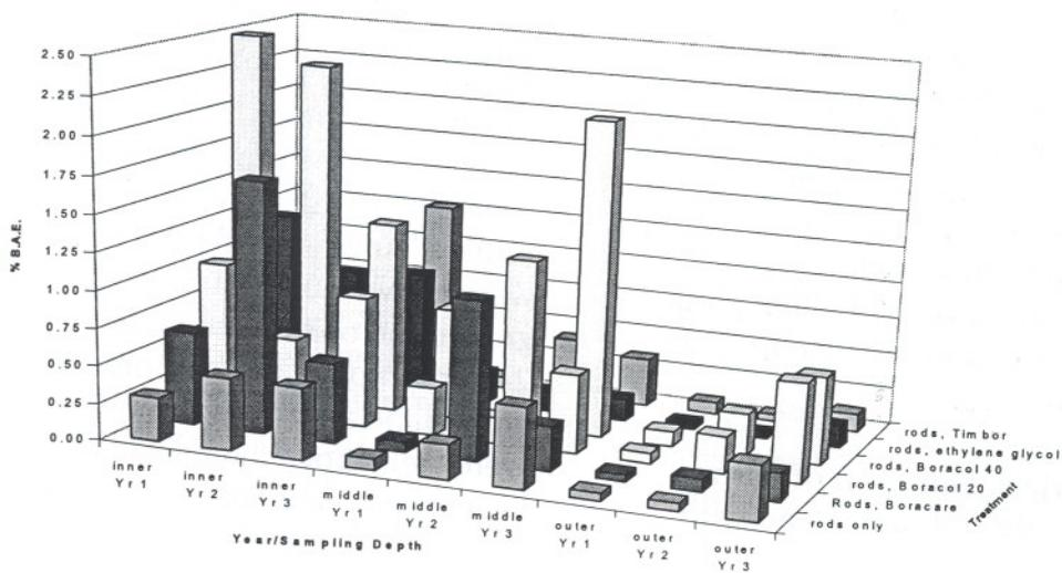
Figure I-17. Boron levels 15 cm above groundline in Douglas-fir poles treated with borates.
