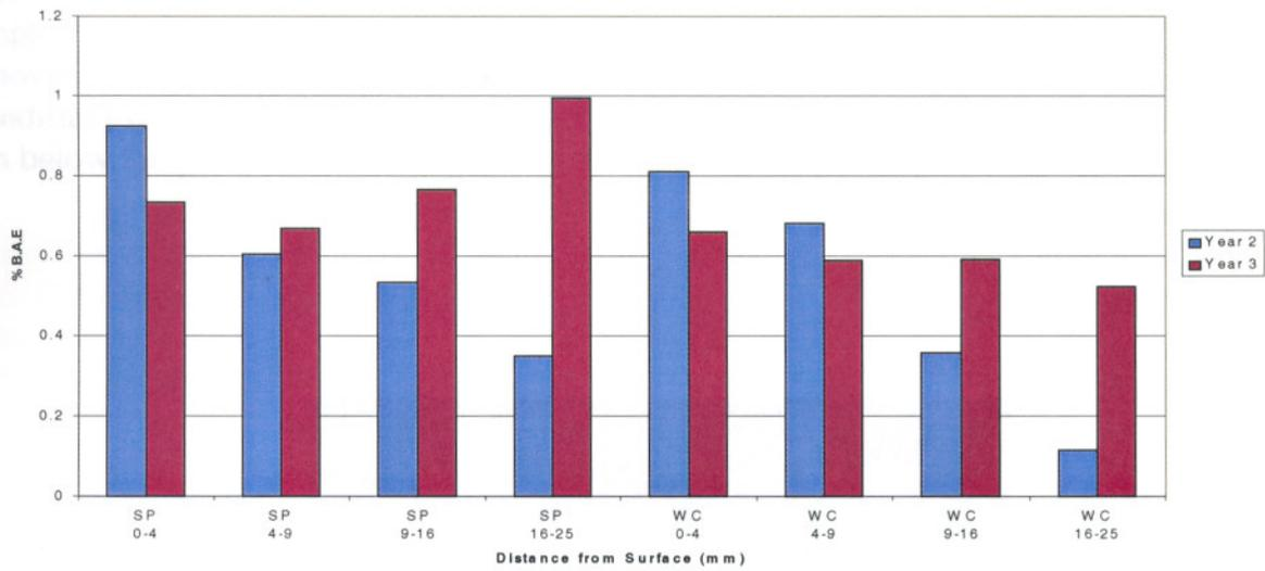
Figure IV-3. Retentions of boron at various depths from the surface of southern pine and western redcedar poles 2 or 3 years after treatment with CURAP 20.
