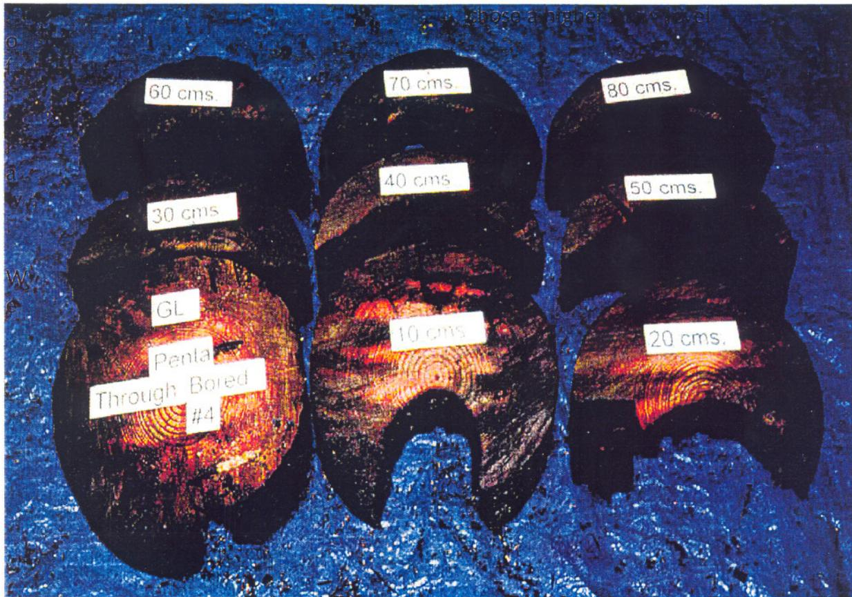
Figure III-11. Cross sections cut from selected locations along the length of a pentachlorophenol treated Douglas-fir pole following fire exposure.
