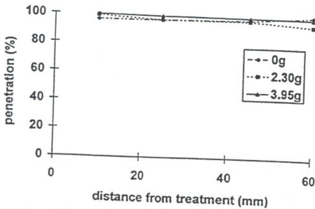
Figure I-5. Penetration of boron in cross sections cut from various distances from holes drilled in Douglas-fir heartwood blocks conditioned to 15, 30 or 60% moisture content and treated 8 weeks earlier with fused boron rod plus selected levels of Boracol 20 to produce a dosage of 3.1 g boric acid equivalent per block.
