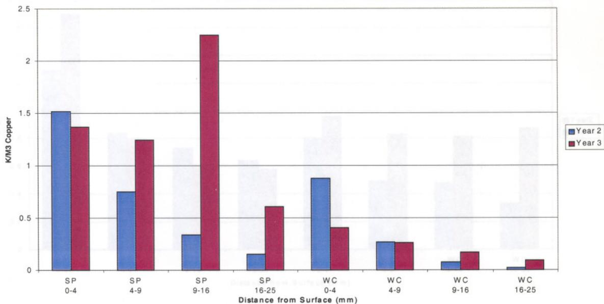
Figure IV-2. Retentions of copper at various depths from the surface of southern pine and western redcedar poles 2 or 3 years after treatment with CURAP 20.
