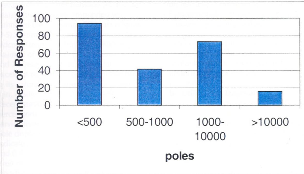
Figure III-4. Frequency of post treatment pole quality inspection by utilities, third party inspection agencies or treating plants.
