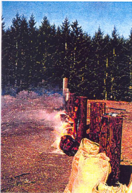
Figure III-9. Burlap bag containing straw that was used to initiate pole ignition.
