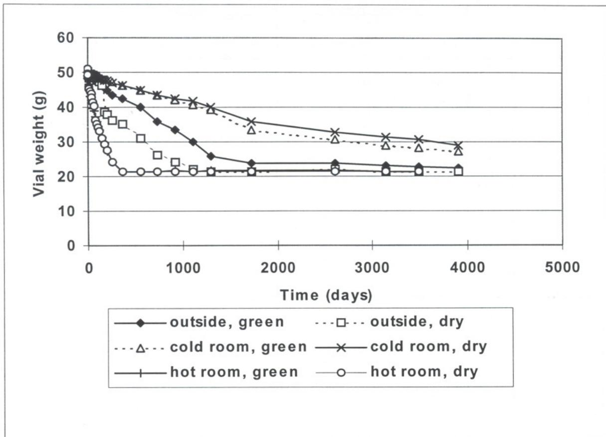
Douglas-fir pole sections incubated at 5 C, 32 C, or in an outdoor exposure remain higher in southern pine poles, a finding that continues to remain puzzling, given the higher permeability of this species.
