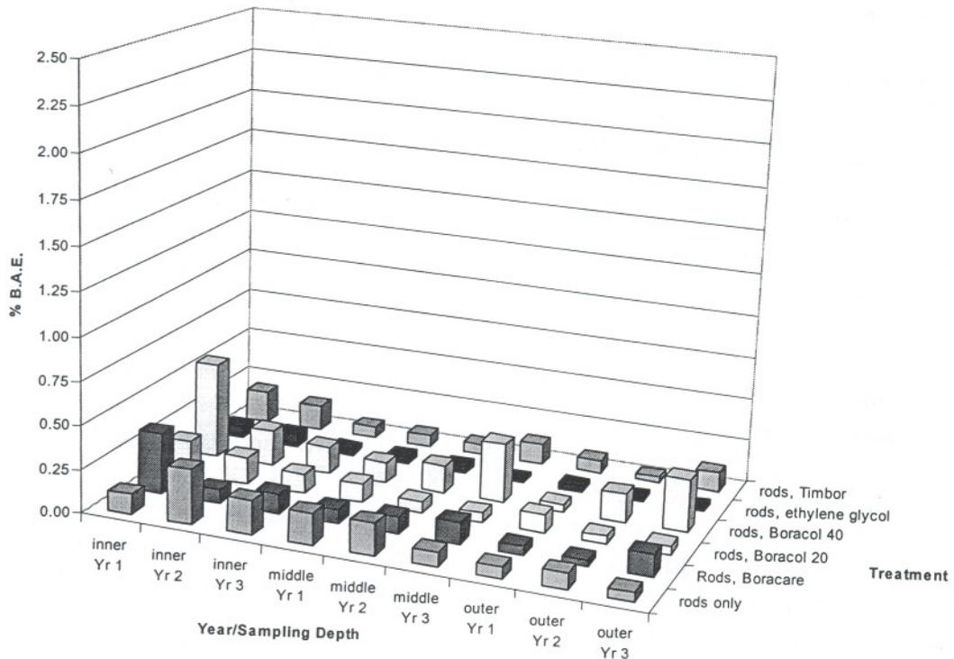
Figure I-16. Boron levels at groundline in Douglas-fir poles treated with borates.
