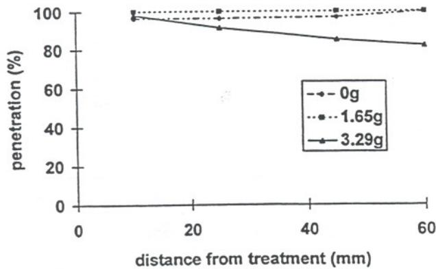
Figure I-6. Penetration of boron in cross sections cut from various distances from holes drilled in Douglas-fir heartwood blocks conditioned to 15, 30 or 60% moisture content and treated 8 weeks earlier with fused boron rod plus selected levels of Boracol 40 to produce a dosage of 3.1 g boric acid equivalent per block.
