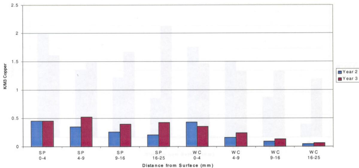
Figure IV-1. Retentions of copper at various depths from the surface of southern pine and western redcedar poles 2 or 3 years after treatment with CUNAP Wrap
