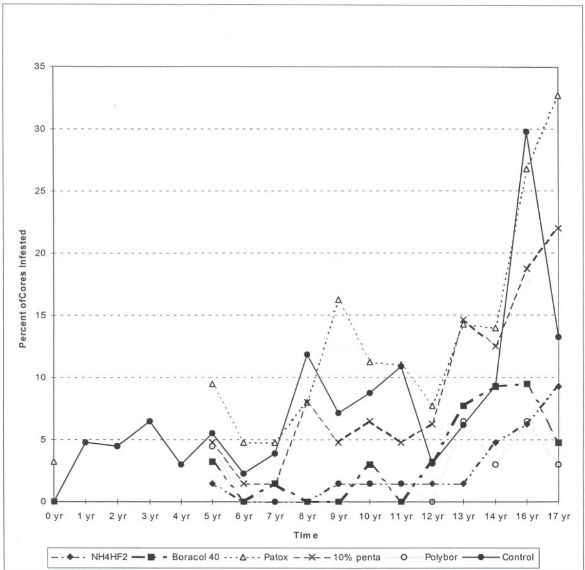
Figure II-1 Effect of topical treatments to field drilled bolt holes in Douglas-fir poles on the percentage of increment cores containing basidiomycetes 1 to 17 years after treatment.
