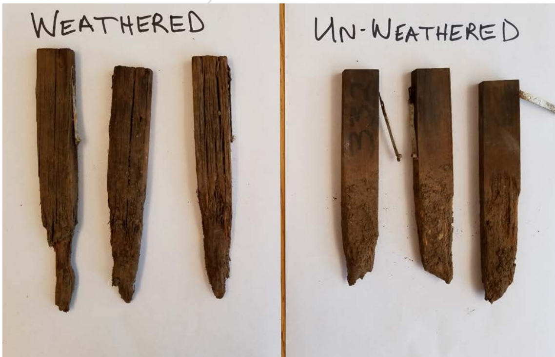
Figure V-3. Examples of western redcedar stakes that have failed in test showing a tendency for the wood to decay towards the lower end of the samples.
