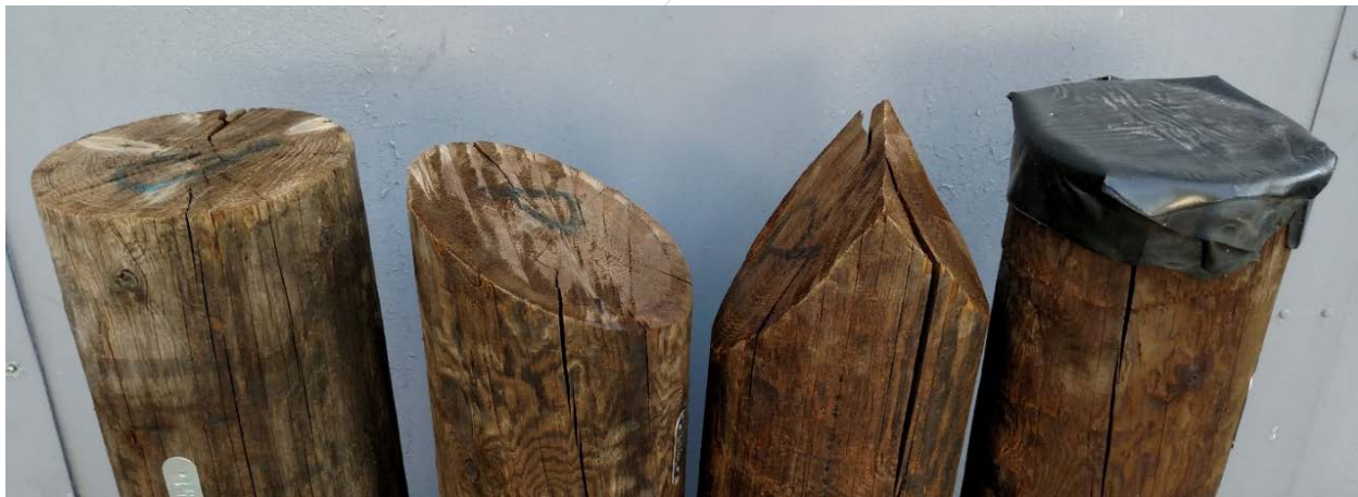
Figure III-22. Examples of the different pole top roofing patterns assessed for their ability to resist moisture ingress.
