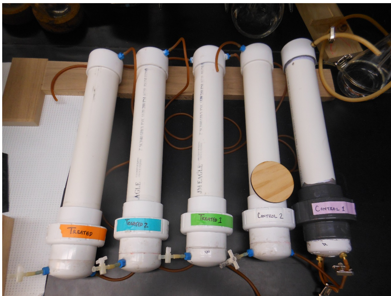
Figure I-4. Photograph of five of the diffusion apparatuses used to assess boron movement through non-treated or diesel oil-treated Douglas-fir lumber. A wood sample is resting on the fourth chamber to provide a measure of scale.
