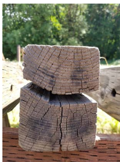
Figure III-18. Example of the opposite ends of a single arm showing a plated end with minimal checking and the opposite non-plated end with a severe split.
