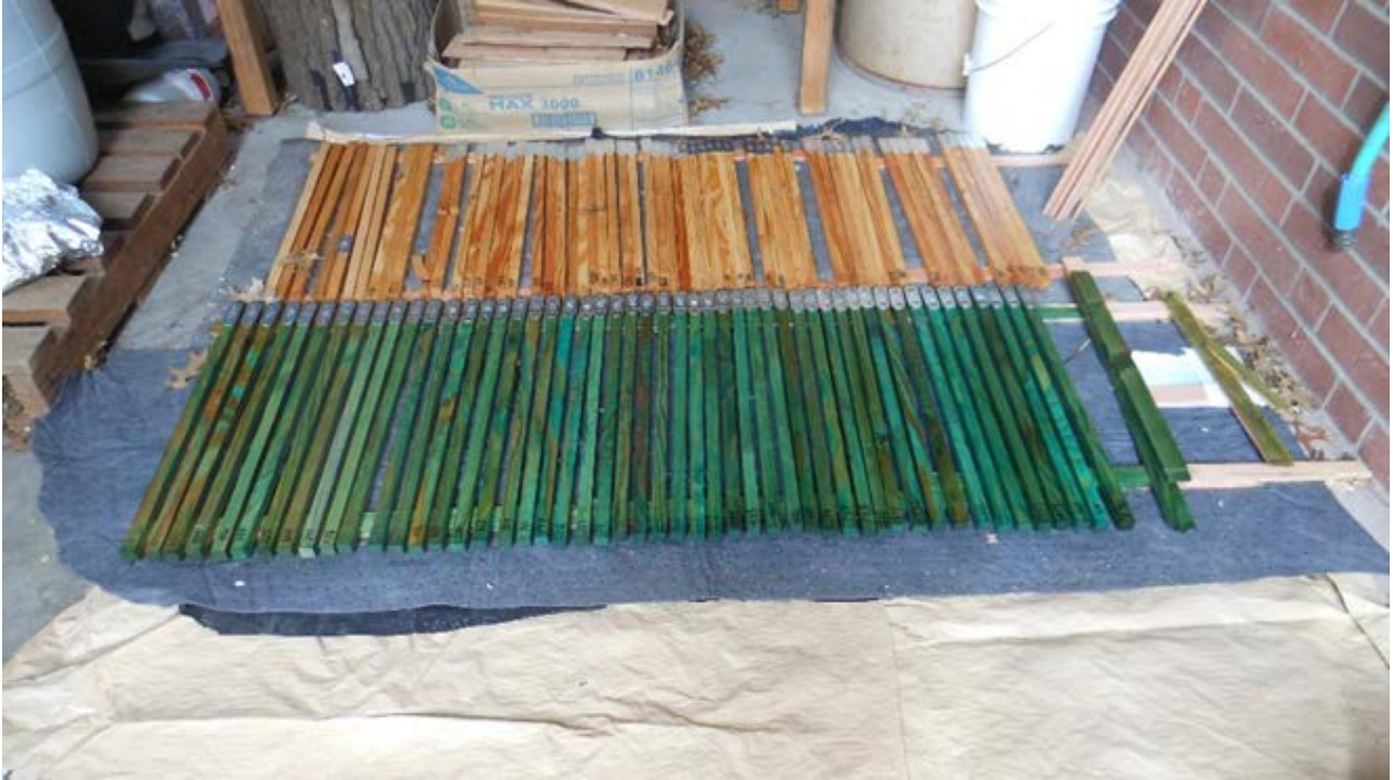
Figure III-23. Stakes drying under cover after treatment with copper naphthenate (bottom) or penta (top).
