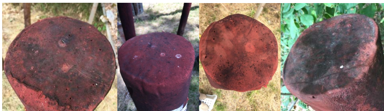
Figure III-21. Condition of polyurea coatings on the tops of Douglas-fir pole sections after 61 months of exposure in Corvallis, OR.
