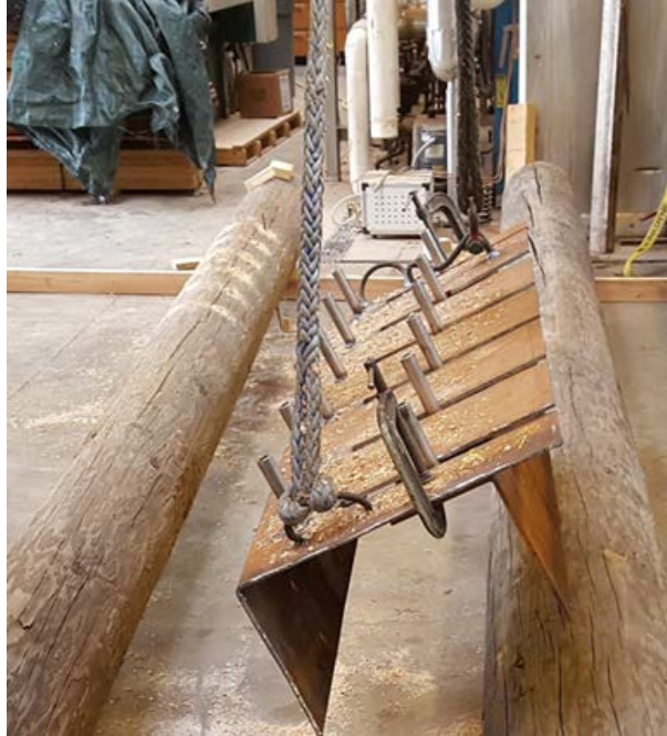
Figure III-9. Drilling apparatus created for the drilling of holes at a constant edge distance. The plate can slide in and out to fit any pole size. Blocks cut to 1 and 2 inches are placed in the interior edges to drill at different edge distances. Holes are drilled downward through the pipes.
