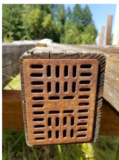
Figure III-18. Example of the opposite ends of a single arm showing a plated end with minimal checking and the opposite non-plated end with a severe split.
